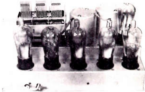
The Small Compact, Sturdy Chassis. Small type, low drain, automobile tubes used exclusively.
