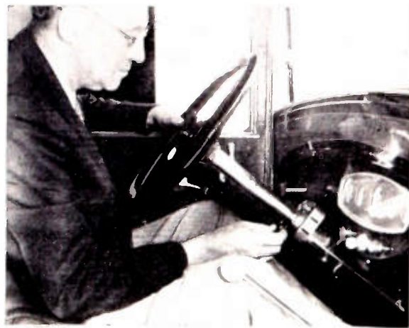
The remote control is attached to the steering post. Inconspicuous, accessible. No necessity to wear the dash.
