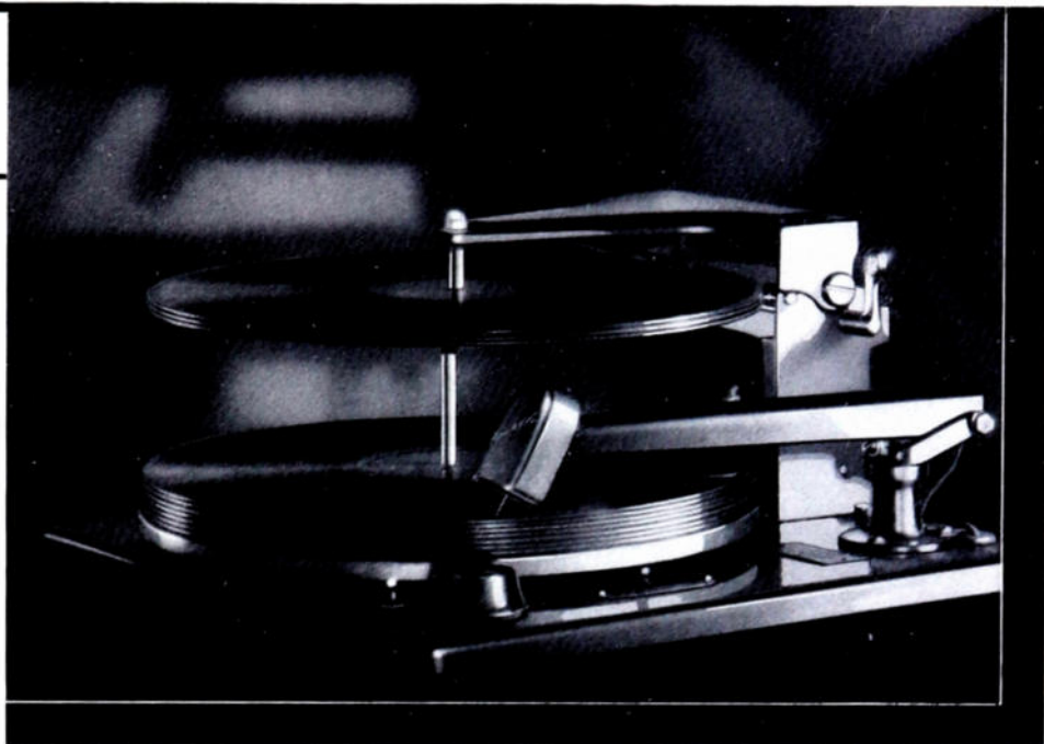
The compact size of the new Capehart record changer—14½" x 14½" x 7½"—makes possible an automatic combination radio-phonograph in a considerably smaller size than ever available before. This unit is equally adaptable to standard and full size instruments. Illustration gives an idea of relative sizes.
