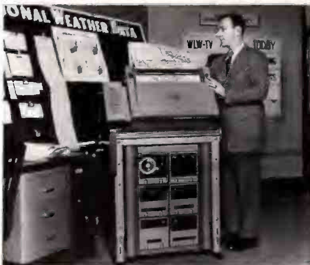
ELECTRONIC WEATHER reports every 20 minutes are recorded on the WLV Cincinnati's new radio-tv weather map machine, which is connected with the U. S. Weather Bureau's Master Analysis Center in Washington, D. C. It is capable of receiving a complete new weather map every two minutes.
