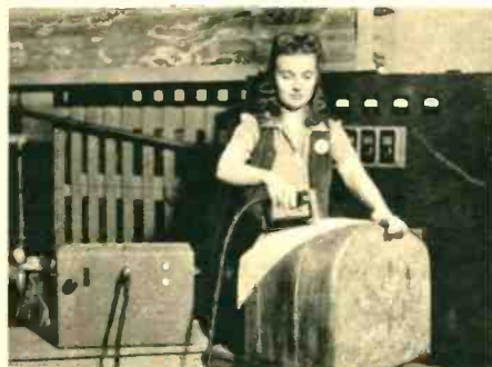
THE "RADIO NAIL" GUN or spot gluer is used instead of tacks or staples to bond thin veneers of wood. A charge of current, shut through the topmost layer, joins it to the sheet below by forming a bond in the glue previously spread between the veneers.
