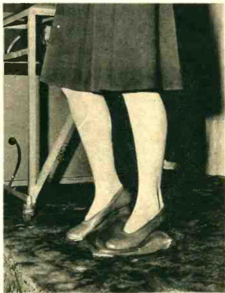
AIR AND WATER-TIGHT FEATURES of "radio seams" are demonstrated by Miss Weatherly, as she stands on an inflated bag of the fabric without bursting the seams. This special material is now used in manufacturing raincoats, balloons and food wrappings.
