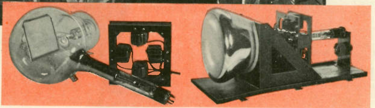
Above, left, the iconoscope invented by Dr. V. K. Zworykin to emulate the human eye and serve in a television camera. The square retina is covered with a light sensitive substance upon which the "gun" in the tube's sleeve projects an electron beam to "paint" the picture. Right, the kinescope. Upon the flat end of the tube the electron beam paints the image.
