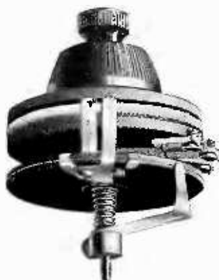
View of Vernier Potentiometer
