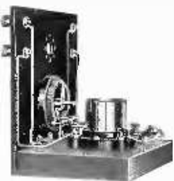
No. 47490 Simplex Detector Panel Side View
