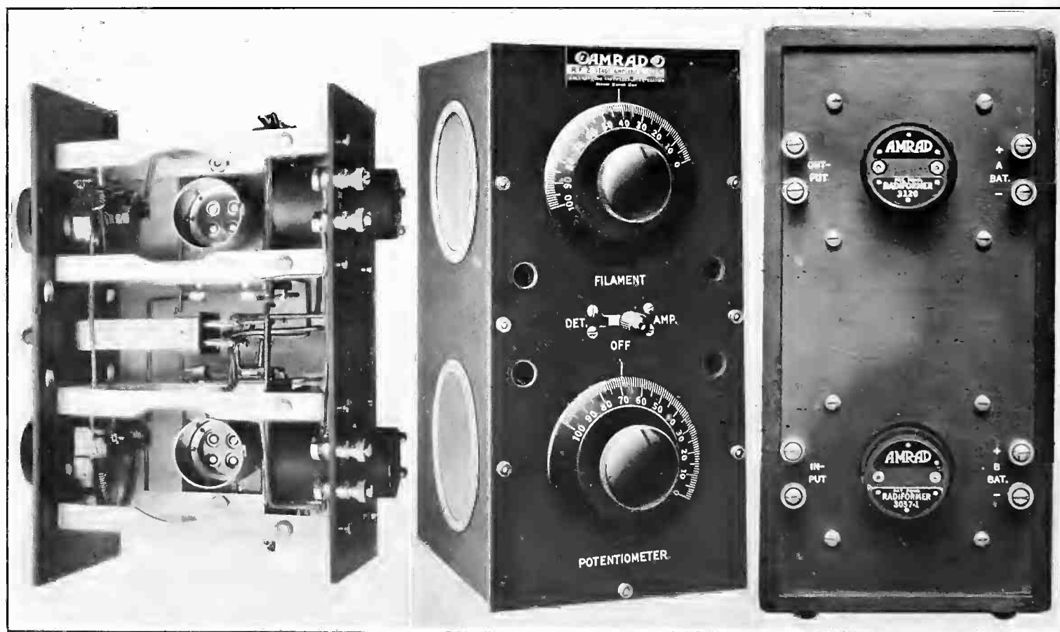
Three Views of the Amrad New Radio Frequency Amplifying Unit
