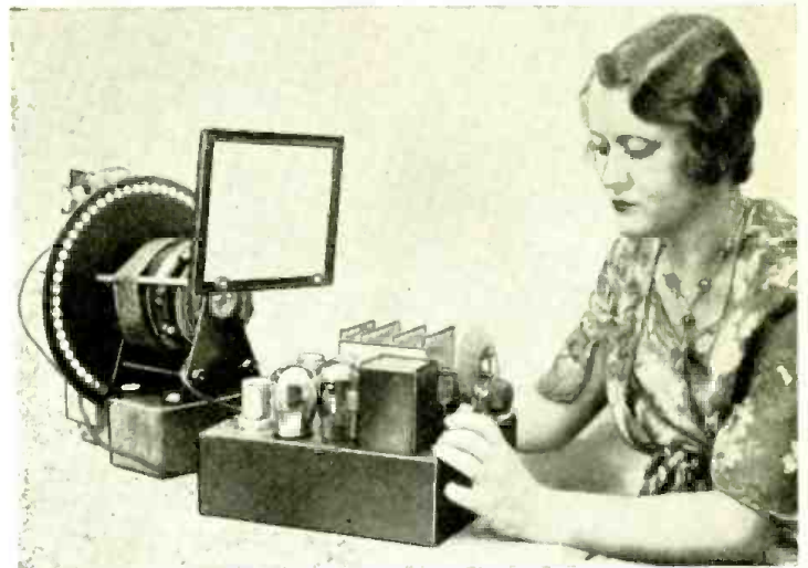
Here is Mr. Matthews' receiver in use with a lens disc scanner and a lens disc glass screen.
