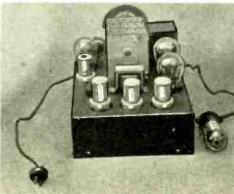
back view. The crater tube is shown next to the chassis, but actually it mounts behind the disc.
