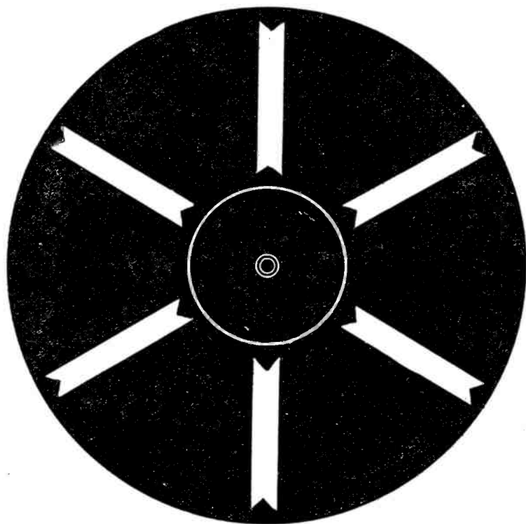
Fig. 3—Above, and Fig. 4 at right, represent two typical charts which can be redrawn larger and mounted on television discs. These designs are to be viewed through a vibrating tuning fork.
