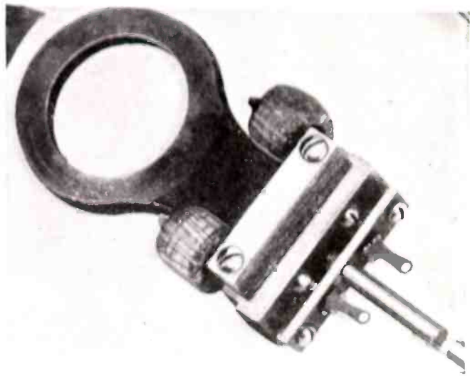
Fig. 6—At left, shows adjustable magnet mounting, forming a part of the special synchronizing motor as shown also in Fig. 5. A toothed rotor rotates between the poles of the two magnet coils and acts to preserve synchronism.
