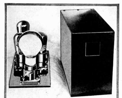
close-up of the photoelectric cell unit appears in the panel above; the cell is the large round bulb at the left; the square opening in the steel can allows the light rays to affect the cell in the proper manner.)
