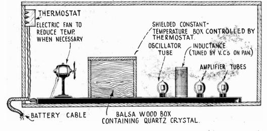
Fig. 4—Elaborate precautions are tal en to keep the crystal at an even temperature, by a double system of thermostatic control.
