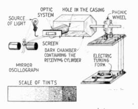
A diagram of the receiving system is shown above. An ordinary sheet of sensitized photographic paper is rolled upon the cylinder, which is placed in a dark chamber. All tasts of the transmitted photograph are received in their exact value.
