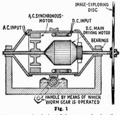
A cross-sectional view of the motor, showing the relative position of the D.C. and A.C. units.
