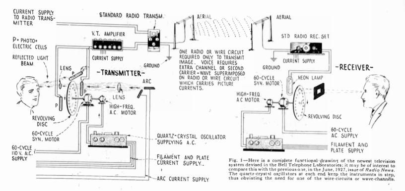
times and not be out of step, during that time, more than one revolution. A correcting button, however, is placed on the television machine cabinet, so that in the event that the picture should "drift" or become distorted, once in a great while, perfect synchronism can again be established by simply pressing a button.
