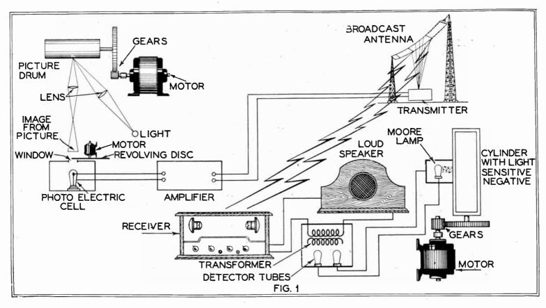
The diagram illustrates the process through which a photograph goes when being transmitted through the ether. When it is finally received on the cylinder on the right, it must be "developed" and "fixed" as with an ordinary print.
