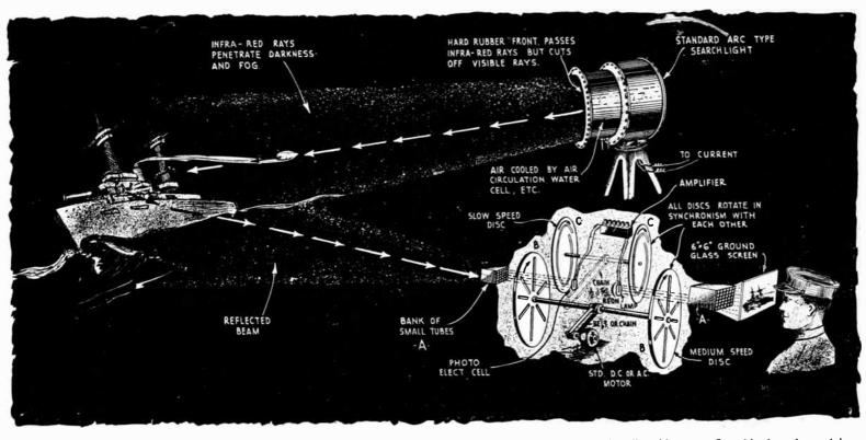
The apparatus used to receive the view lluminated by the invisible beam of th<sup>e</sup> infr-red searchlight and render it visible to the eye of the operator, is shown in th<sup>e</sup> above illustration. The infra-red rays have the property of penetrating darknes<sup>3</sup> and fog and thus lend themselves to use during war time and also in locating ship<sup>8</sup> lost at sea during a storm.
