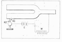
Diagram showing the principle of tuning-fork control.
