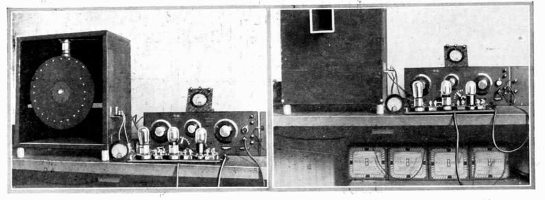
Here we see the disc cabinet at left with cover removed. The neon tube can be seen directly behind the disc. The amplifier appears at right. Photo above shows neat arrangement of amateur television receiving apparatus. The resistance coupled amplifier is shown at right and the disc cabinet at left.
