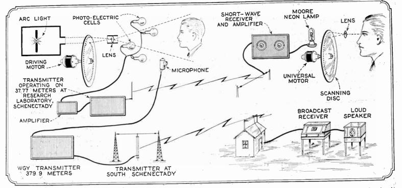
the microphone for the voice, which is broadcast on a different wavelength. At the right are the receivers for television and speech.
