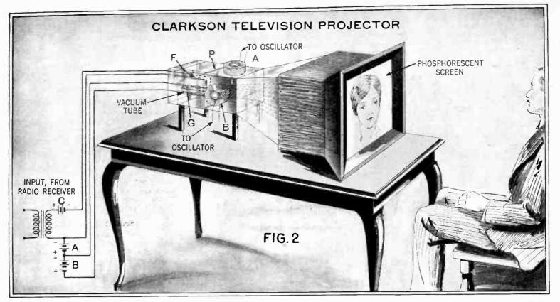
The receiving televisor, similar in construction to the transmitter, makes use of an identical two-element electron-projecting tube. The image will appear on a phosphorescent screen. There are no moving parts at either end, except the electrons. The idea seems very promising indeed.
