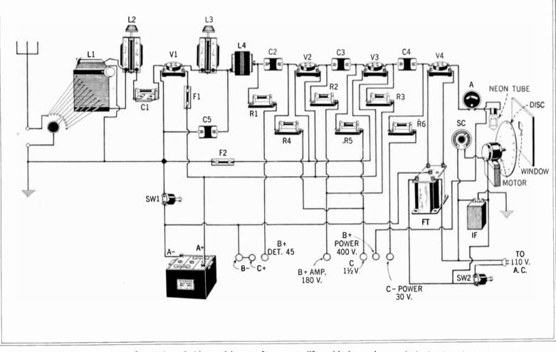
This picture diagram shows the wiring of a complete television receiving set. It consists of a standard regenerative tuner, followed by a resistance-coupled A.F.
