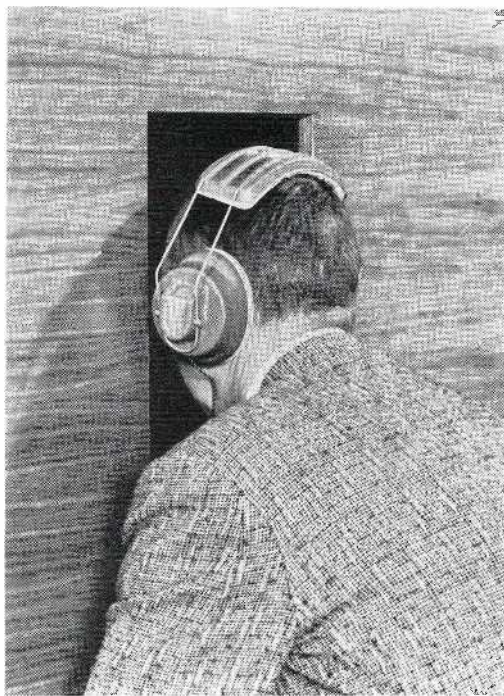
A camera mechanism records pupil dilation and eye movement as the subject looks at picture on opposite interior wall of this cabinet. Earphones exclude outside sounds that might affect subject’s response.
