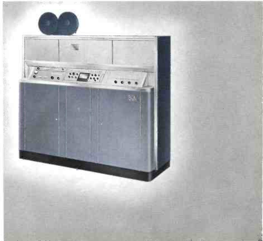
TFR-1 TELEVISION FILM RECORDER. New high-resolution Kine eliminates face plate distortions, resolves up to 900 lines, provides highlight brightness of 160-foot lamberts. New double-aperture camera eliminates shutter bar, lessens vibration. Self-compensating circuits assure uniform contrast, automatic control of exposure. Used with fast film developer to play back pictures in 2 minutes.
