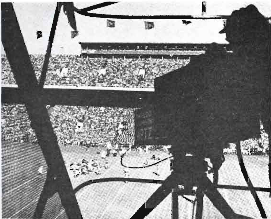
Even back in 1944, the Penn football games had been telecast on Philadelphia's WPTZ for 5 years. Caption in '44 read: "Two cameras are used; both operate on specially built platforms suspended from the upper south stands at about the 50-yard line."
