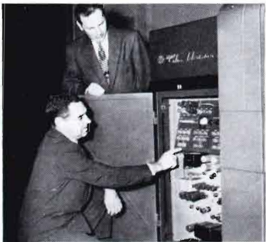
This 3-Vidicon Color-TV Film Camera handles 16mm, 35mm color film and slides.
