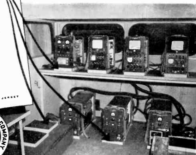
Interior of truck showing rubber mountings
