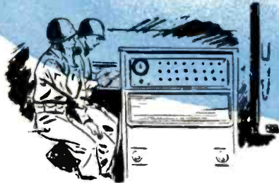
Bell Laboratories designed and Western Electric produced more than 1600 electronic gun directors and gun data computers which greatly increased the accuracy of anti-aircraft and coast defense guns.
