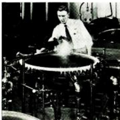
(Left) Sealing picture-tube face plate to metal shell at DuMont.
