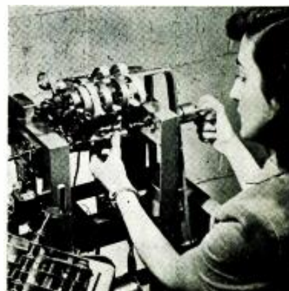
(Left) Sealing picture-tube face plate to metal shell at DuMont.
