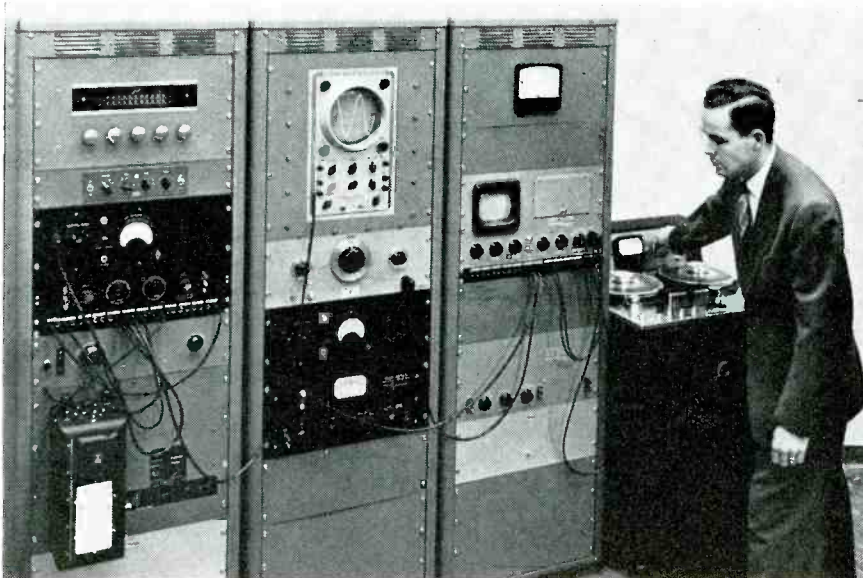
Left: Sound recording tape, recorder and playback lab equipment recently installed by Minnesota Mining to permit measuring of output and uniformity of output at any frequency, signal-to-noise ratios, dynamic range, wow, flutter, harmonic distortion, intermodulation, and modulation noise. Included in equipment are an AM-FM tuner, 'scope, wow meter, Ballantine voltmeters, dual-channel oscillograph with associated dc amplifiers, two hi-fi audio amplifiers, two professional quality recorders that operate at any speed from 3 3/4 to 15 inches per second, and a sonic analyzer for measuring distortion and frequency response and for showing noise spectra. Bias circuit, built into recorders, is said to permit introducing wide variations in bias.
