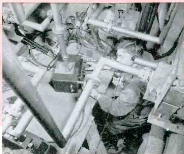
The Type 1601-A V-F-H Bridge set up to measure the antenna of WCBS-TV on the Chrysler Building, New York City. The antenna consists of 16 radiating elements. Measurements of the impedance variation of an individual element over the operating frequency band as well as impedance measurements of the whole array were made easily and accurately.
