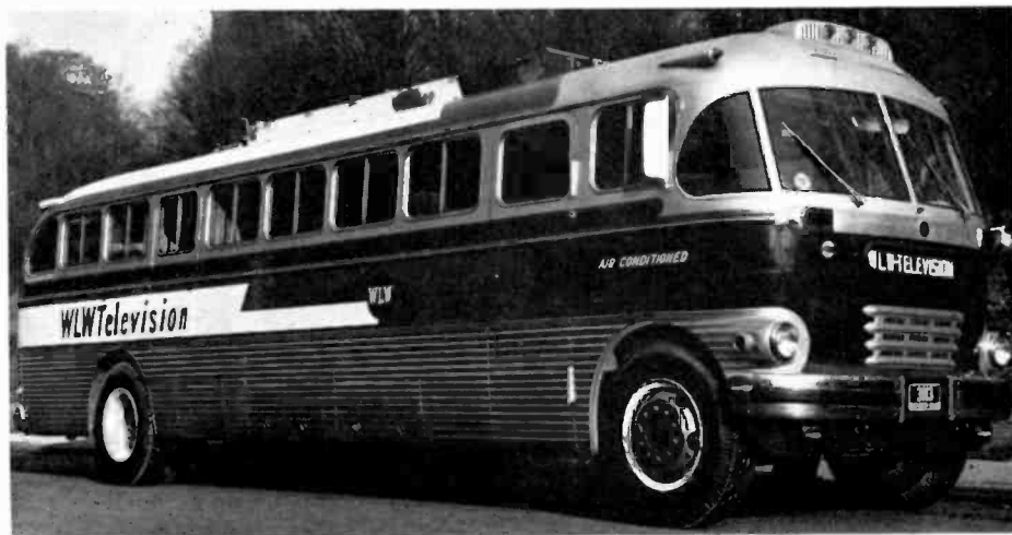
This unit can carry 22 remote crew and all necessary remote equipment. It is 35 ft. long and weighs 23,000 lbs.; air-conditioned for summer; has hot water heat for winter; has fluorescent lighting. Was used as WLWT's first studio relaying its originations to Carew Tower in Cincinnati.
