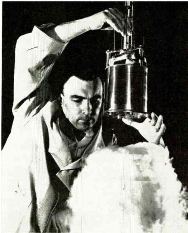
A superconductive magnet, producing 107,000 gauss, is lowered into a vapor-shrouded bottle of liquid helium by Frank Kolondra of RCA. The magnet will enable small and medium-sized laboratories to carry out experiments which are now possible only in large installations.
