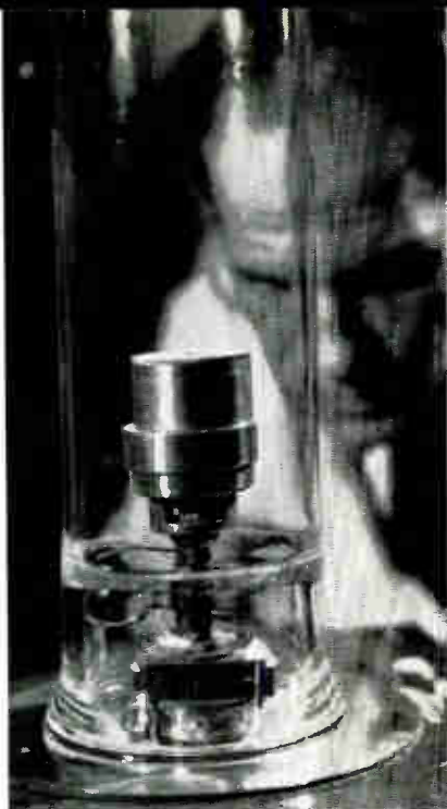
A new thermoelectric material, consisting of an alloy of germanium and silicon, produces a great amount of electricity directly from high-temperature heat. Tests performed by its developer, RCA, indicate that a generator using a sq. ft. platelike arrangement of the material heated to 1000°C could produce 10 kw.
