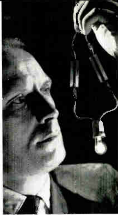
Dr. John H. Lupinski, of GE, demonstrates new conducting polymers, visible in photo as black strips of special plastic material painted on an ordinary white plastic insulator. Electric current flows through thin polymer strips and lights a small bulb.
