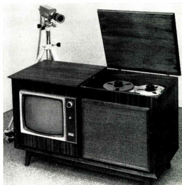
Fig. 1: Lab prototype of Industrial TV Video Recorder.
