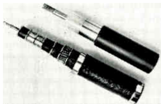
New armorless deep-sea cable (upper right) is of simpler construction, and has lower transmission losses than previous cables of the same overall diameter (lower left). Unlike armored cable, it twists very little during laying.
