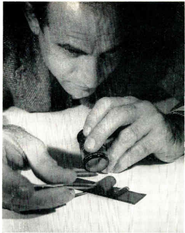
Dr. R. Shahbender inspects thin ferrite sheets which will become a computer memory when laminated and cured. Unit shown here will store 16,384 bits of information in a total volume only 1 x 3 inches square and 5 one-thousandths of an inch thick.
