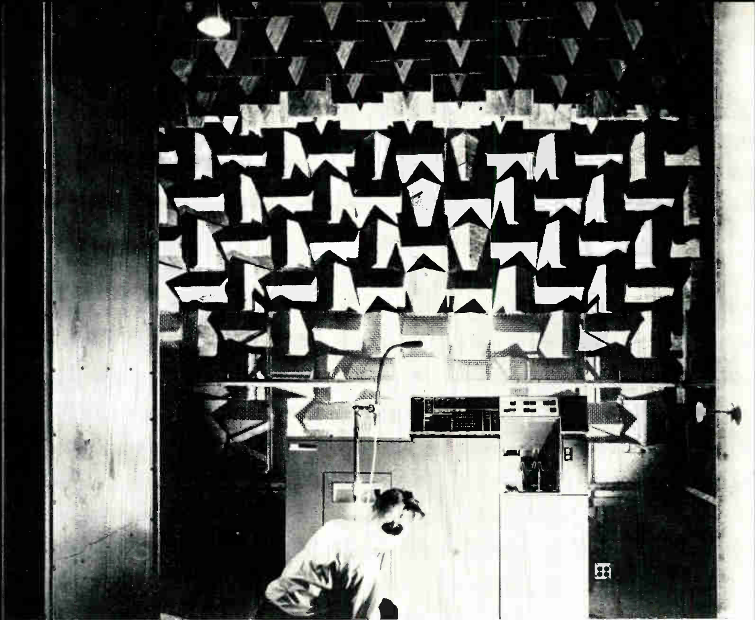
Fig. 1: Acoustical absorbers made from glass fiber boards in the shape of wedges provide 99% absorption in anechoic rooms.
