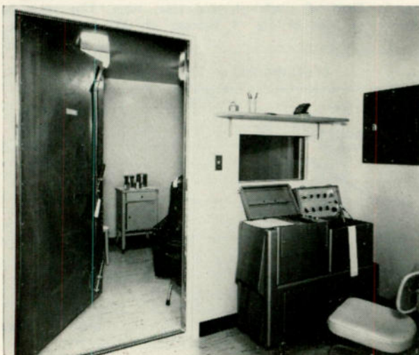
Single steel room used at Stanford Medical Center in Calif.
