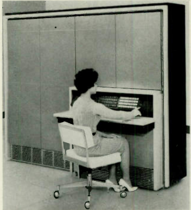
RCA 30 computer will produce up to 20,000 lines/hr. of automatically justified and hyphenated type on teletypesetter tape.
