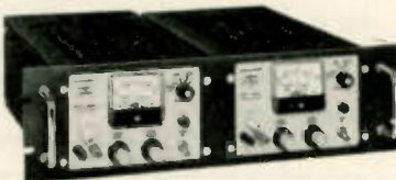
Two Trygon HR20-1.5's, rack-mounted side by side.
