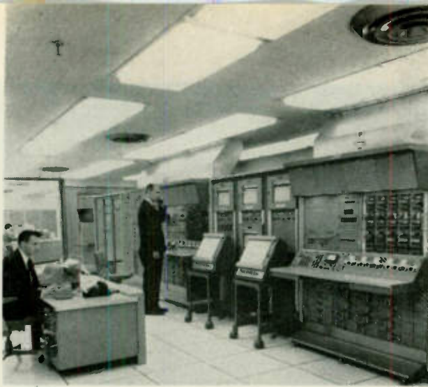
Industrial processes are simulated by analog computers and controlled by a digital computer at Honeywell's systems simulation center in Pottstown, Pa. Hybrid facility consists of two EAI 231R analog computers (foreground) of special design and a Honeywell 290 digital computer (background).
