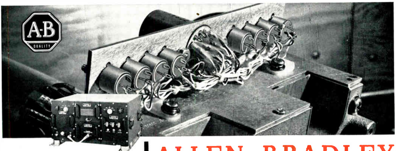
Electronic Communications' AN/ART-42 UHF 1 KW AM/FM Transmitter in service with the SAC, and internal view showing use of A-B's Type G controls.
