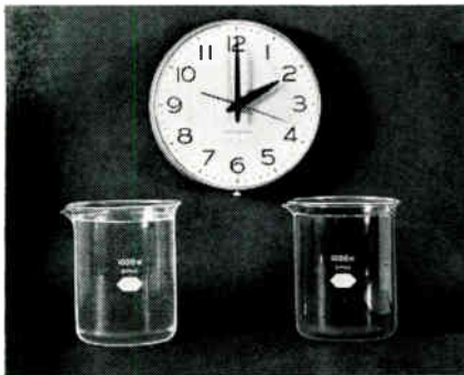
Both resins (1,000 gram quantities) are room-curing epoxies. "Scotchcast" No. 8 is at right, ordinary epoxy resin is at left.
