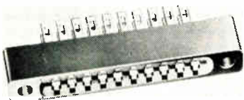
Miniature connector made by Continental accepts either pc boards or tape cable. It uses "Bellow-form" contacts which provide coil spring action grip that clasps the pc board over the entire contact area.
