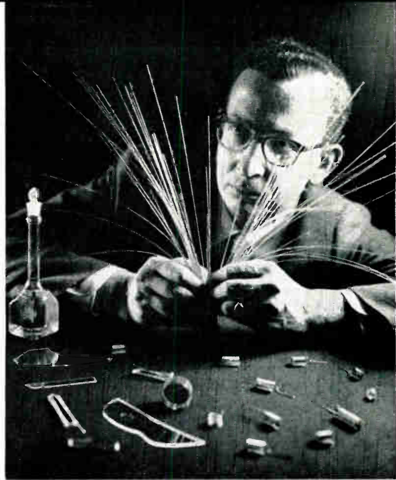
Dr. Nikolaus Wolff holds a spray of plastic fibers similar to those which have produced laser action. In the foreground are other shapes that future plastic lasers might take.
