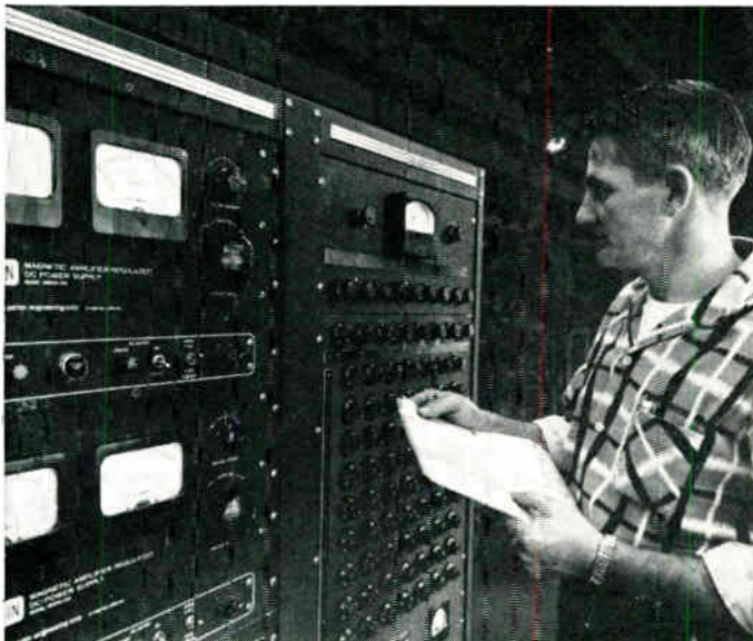
Production line sorting. The next to the last quality control check made before shipment. All COLDITE 70+ Resistors coming down production lines pass this machine which automatically measures resistance values. Machine unerringly classifies resistors according to specified tolerances.
