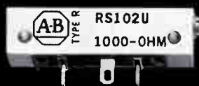
(C) HOT MOLDED ADJUSTABLE FIXED RESISTORS —Rated 1/4 watt at 70°C. Values to 2.5 meg. Tol: \pm 10 and 20%.
