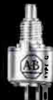
(D) TYPE G HOT MOLDED POTENTIOMETERS —Only 1/2" diam. Rated 1/2 watt at 70°C. Resistance values to 5 meg. Tol: \pm 10 and 20%.
