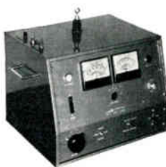
Model 424 HYPOT provides 0-5000 v d-c for testing cables, condensers, coils, transformers and assemblies. Measures leakage 0.1 to 100 microamperes over four scale ranges. Rapid charging of capacitors with 5 ma. output. Self-contained power supply. Complete $497.00.
