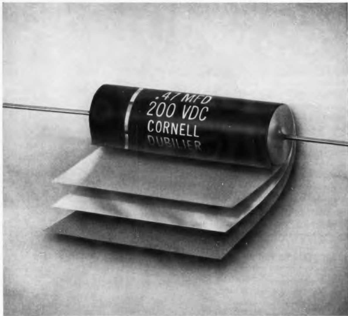
Jaguar: Cornell-Dubilier's new dual-dielectric (polyester film and impregnated kraft paper), triclاد cardboard tubulars, Type PTL. Triclاد case consists of specially-impregnated glossy black kraft envelope enclosing a bonded shield of aluminum foil and moisture-resistant polyester film.
