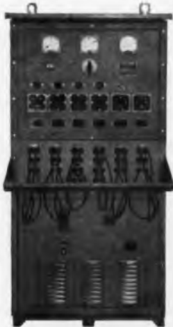
ABOVE — 6 CIRCUIT POWER SUPPLY Output: 4 circuits, 45 amp, 65 volt DC 2 circuits, 1.8 amp, 65 volt DC Input: 460 volts, 3 phase, 60 cycle
