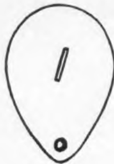
Fig. 4: Drawing may be used as the pattern for the metal gear change piece on switch.
