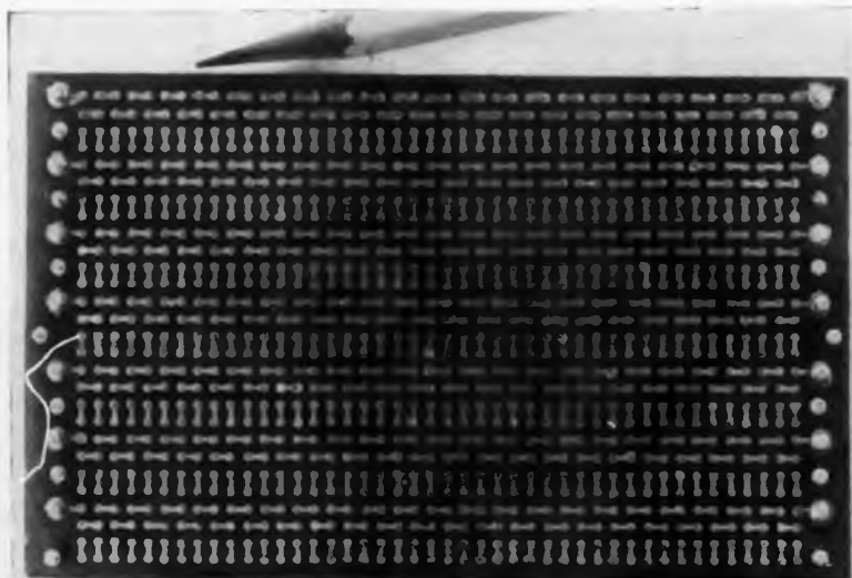
Fig. 6 (right): This is the connection test board which contains some 1200 brass slugs, or feedthroughs, connected in series.
