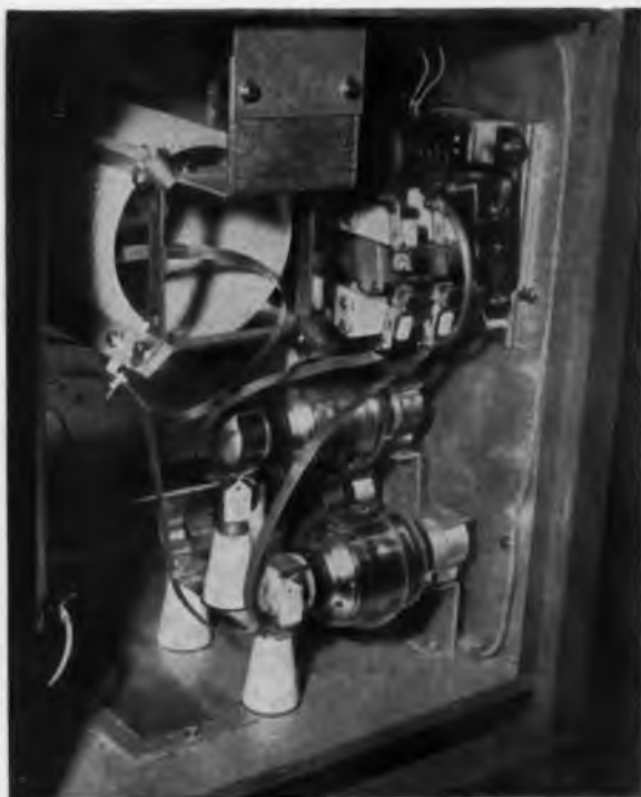
Gates Radio Company Broadcast Transmitter utilizing Jennings type M-1000 and M-750 Vacuum Fixed Capacitors.
