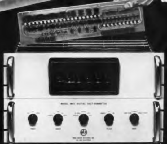
Digital voltmeters — originated by NLS — permit rapid and accurate voltage measurements. New Series 20 unit — with one plug-in decade board removed — shows the use of Allen-Bradley fixed resistors.
