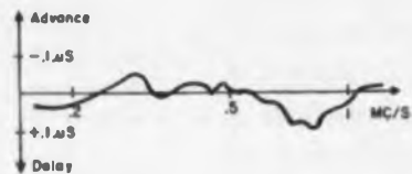
Fig. 6: Overall envelope delay curve for the Mincom CM-100; the tape speed is 120 cps.
