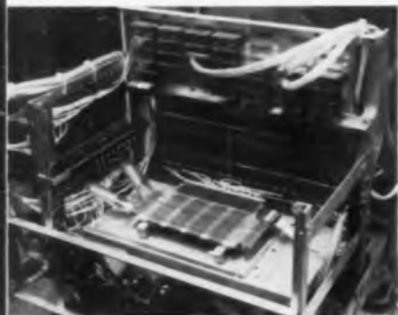
Fig. 2: Completed 3328-bit, 0.3 \mu sec. magnetic-film main memory of the FX-1 computer.
