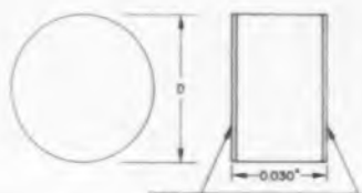
Fig. 1 (left): Disc-shaped component with a thickness of 0.030 in. is standard of the Dot System.
