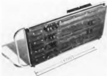
Fig. 4: Development plated-circuit tray, holding up to 20 plug-in units, has two layers of wiring on either side of a central ground plane, functioning as strip transmission line with uniform impedance characteristics.
