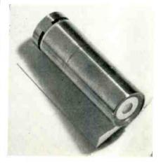
microns; detector area,  $3.5 \times 3.5 \text{ mm.}$ ; impedance, 50,000 ohms to 1 megohm; acceptance angle, approx. 100°; response, measured with a blackbody at 500°K at 800 CPS and referred to 1 cycle bandwidth. NEP =  $7 \times 10^{-10}$ to  $7 \times 10^{-11}$  w; D\* =  $5 \times 10^8$  to  $5 \times$  $10^9$  cm/w; time constant, less than 1 microsecond. Applications Engineering Dept., Raytheon Co., Waltham, Mass.
