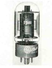
rounded-top envelope for "rattle control" which reduces microphonic action under vibration. Zero-bias characteristics: plate, 70 v.; screen, 300 v.; control grid voltage, zero; plate current, 210 ma.; and screen, 25 ma. Max. ratings: 500 v plate, 450 v screen, 30 w plate dissipation, and 5 w screen dissipation. General Electric Co., Receiving Tube Dept., Owensboro, Ky.
