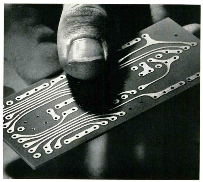
FOTOCERAM circuit baard blanks are made using the micra-accuracy af photography. All holes and shapes are produced by simple expasure to light, heat, and an etching operation.
