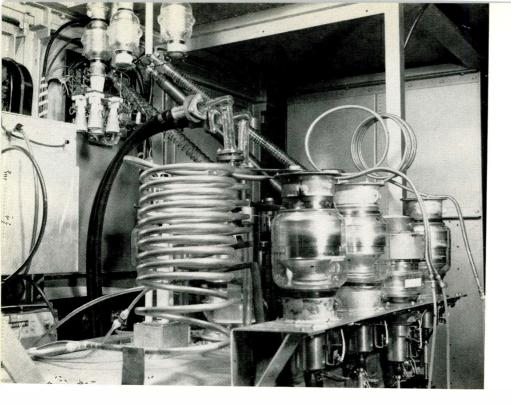
Fig. 1: Final amplifier plate circuits and r-f chokes utilizing motor operated vacuum variable capacitors are shown.
