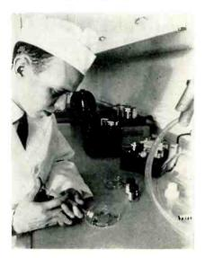
This "White Room" lab is part of the new West Coast headquarters of Miniature Precision Bearings, Inc. It is located at 8621 Bellanca Ave., Los Angeles, Calif. Engineer Robert Pierson is lubricating a miniature precision bearing.
