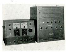
Model 8514 HYPOT<sup>R</sup> high voltage test set used with the tester. The rate of rise for this test potential and the length of time it is applied to each unit (up to 15 min.) is adjustable. All units, when not under test, are short circuited. Leakage current metering circuits have ranges of 0-10/25/100/250 ma. Automatic reject controls are adjustable from a min. of 0.5  $\mu$ a to a max. of 250 ma. Associated Research, Inc., 3777 W. Belmont Ave., Chicago 18, Ill.
