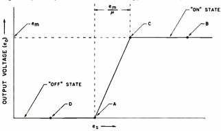
the first phase  $(e_o = 0$  to  $e_o = e_m/\mu)$  when the output is dependent on the input voltage and, consequently, that output pulses would not be the same shape for all input waveforms. For these reasons the hysteresis (which is equivalent to the peak-to-peak sensitivity of the trigger circuit) must be 6v or more.
