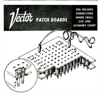
Vector Patch-Boards provide simple, economical units for multiple-connection, single conductor patching. Useful for low cost computers, test boards and a multitude of connecting applications. Receptacles are 0.265" on centers and take .087-.091 diameter plugs. Patch cords also available. Standard boards available or readily made to size required. Write for information:
