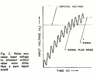
are ineffective. The circuit cannot switch to the "off" state until the input voltage falls to the "off" level. The "on" and "off" levels should, therefore, be separated by more than the peak-to-peak noise but less than the peak-to-peak signal. For this reason the hysteresis should be adjustable to accommodate various signal and noise amplitudes. We will find that the best way to modify the effective hysteresis is by amplifying or attenuating the input signal.
