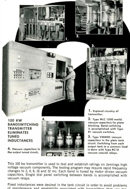
of maintenance and resetability associated with transmitters that use tap switches and sliding contacts. This was made possible by taking advantage of the low minimum capacitances, small size, and low inductance of vacuum variable capacitors. This circuitry would be particularly useful in any rf transmitter design demanding daily repetitive frequency changes.
