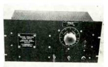
and a step function of  $\pm 5\%$  line change; slow regulation: no load to full load and a  $\pm 10\%$  line change; total regulation: slow, dynamic and ripple will not exceed  $\pm 1\%$ ; ripple voltage: will not exceed 10 mv max. Power supply is short circuit protected and will meet electrical specs to 35°C. Dc output voltage floating from chassis, with external voltage sensing available. The Daven Co., Livingston, N. J.
