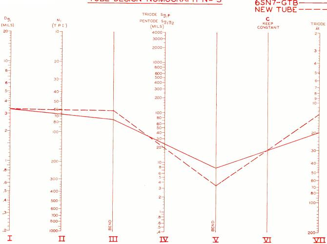
Fig. 7: The parameters of the new tube, which used the 6SN7-GTB as an original, can be determined by working back on this nomograph.
