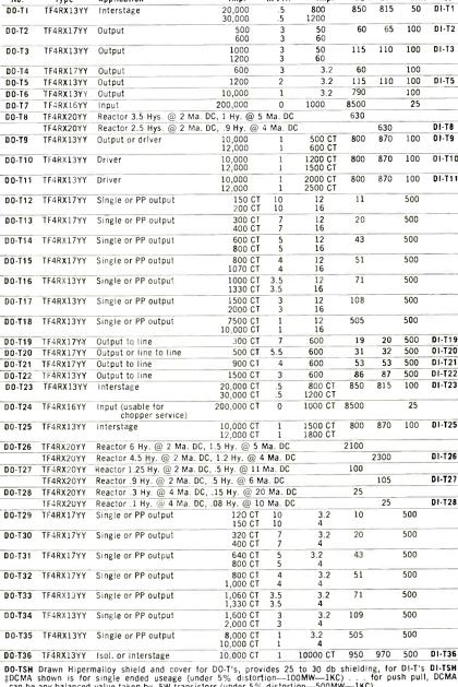
**D0-TSH** Drawn Hipermalloy shield and cover for D0-T's, provides 25 to 30 db shielding, for D1-T's D1-TSH 2DCMA shown is for single ended useage (under 5% distortion—100MW—1KC)... for push pull, DCMA can be any balanced value taken by .5W transistors (under 5% distortion—500MW—1KC) "D0-T units have been designed for transistor application only... not for vacuum tube service. Pats. Pend.
