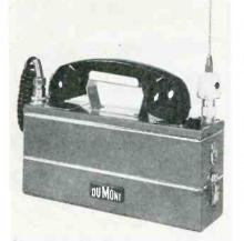
less than 12 in. in length. It includes a handset, FM receiver, 1 or 2 channel FM transmitter, demountable whip antenna, battery pack, and carrying strap. Available with loudspeaker and palm microphone and for use on the 25-54 MC frequencies or 144-174 MC band. Power output in excess of 1 w on lower frequencies. Allen B. Du Mont Laboratories, Inc., Clifton, N. J.
