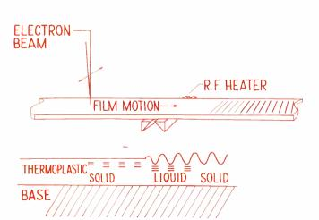
Fig. 1 (left): The melted thermoplastic coating is deformed by the charges. The ripples are then frozen in place.
