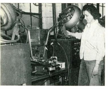
A PRODUCTION combination of standard component feeding devices and hydraulic operated presses can often solve difficult assembly problems encountered in electronic part manufacture. Radio Condenser, Co., Watseka, Ill., in their assembly of miniature components, has employed this production combination.
