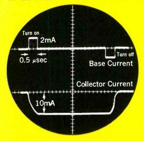
The TRANSWITCH is a new bistable silicon device that can be TURNED OFF with gate current.
