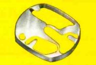
Full stock thickness at top of draw on .018 brass case improved watch quality and saved assembly time.
