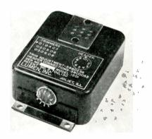
are: amplifier output impedance, 1000 ohms (max.); amplifier output signal, 0-5.0 v.; amplifier output linearity,  $\pm 1\%$  of full scale ( $\pm 50$  mv); amplifier zero shift,  $\pm 1\%$  of full scale ( $\pm 50$  mv); amplifier frequency response, approx. 2 CPS; excitation voltage, 28 vdc  $\pm 5\%$ ; amplifier input impedance, 100 ohms per 1 mv input signal. Lumen, Inc., Moen Ave., P.O. Box 905, Joliet, Ill.
