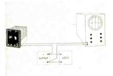
istics of dc power supplies by removing the dc component and utilizing the scope to its max. capabilities. Voltage adjustment is in 75 v. steps for coarse adjustment, with fine adjustment potentiometer 0.25 v./degree; ripple is less than 1 mv RMS. The unit has current limiting and short circuit protection. Acme Electric Corp., Cuba, N. Y.
