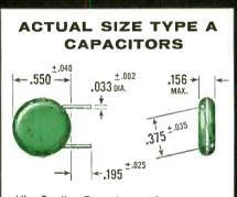
Allen-Bradley Type A capacitors are available in the mast frequently used types and capacitance values.
