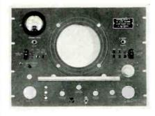
the absolute power level, and a cathode ray tube to display in visual form, the information necessary to evaluate network characteristics. Hallamore Electronics Co., 714 N. Brookhurst Ave., Anaheim, Calif.
