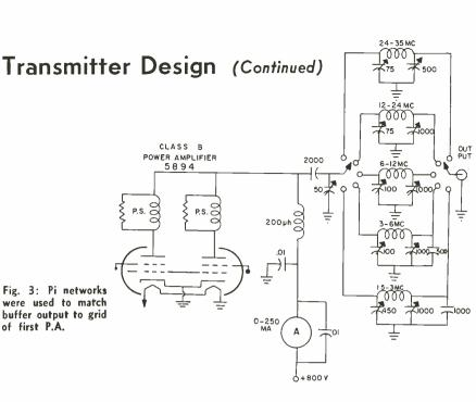
put circuit and dissipating a given amount of energy, we simultaneously reflect a low impedance at the grid itself. This assures stable operation and reduces the tendency towards non-linearity should we use this for AM or SSB linear amplifier service.
