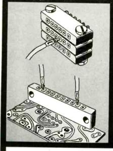
That's the purpose of Kulka Type 399 Miniature Taper-Pin Terminal Blocks. On one side, taper-pin receptacles accept AMP Type 53, Burndy or other equivalents for solderless wiring. On the other side, counter-bored brass terminal studs accept wire up to No. 20 AWG. Or the same studs can be slipped through printed wiring board holes for dip-soldering on reverse side.
