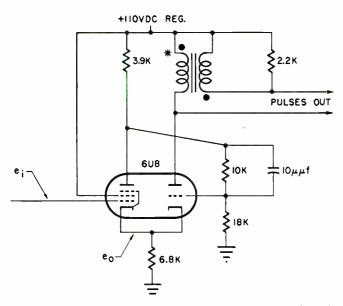
Fig. 7: Actual Schmitt Trigger circuit used in "7000 Series". Amplification occurs in the pentode circuit. The second stage (triode) operates as a cathode follower to provide a low-impedance feedback signal which is direct-coupled to cathode of the pentode. A pulse transformer in the plate circuit of the triode differentiates plate current changes to create output pulses.
