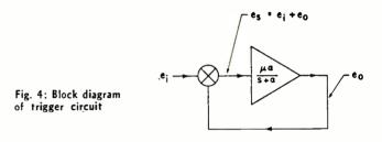
$$e_{o} = \frac{R}{\alpha \ (\mu-1)} \left[ \frac{\mu}{\mu-1} \ \epsilon^{\alpha(\mu-1) t} - \alpha \ (\mu-1) \ t-1 \right]$$
