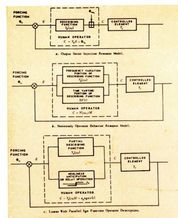
Fig. 7: Human Engineers see man as a "component" in a control system. The non-linear portion of the human's output is as important as the describing function in describing human behavior. From "A Review and Summary of Tracking Research Applied to the Description of Human Dynamic Response." See bibliography.
