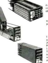
Airborne Time Code Generator illustrates high-density packing obtainable with T-Series circuits.
