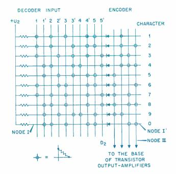
Fig. 9: The resistor matrix is capable of code translation from teletype to an excess-three code
