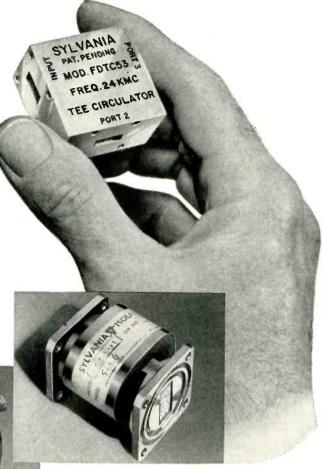
Waveguide Isolator – FD-5213A – this miniature X-band isolator is representative of Sylvania's success in miniaturizing these important components. Units from 2.6 to 26 KMC are available.
