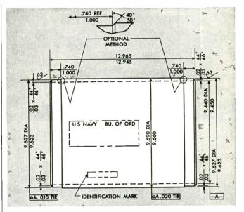
In the drawing above, a reinforced plastic battery shell that we have made in quantity for the U.S. Navy Bureau of Ordnance. Tolerances were tight... such as  $\pm .002''$ on this 10-1/4" dia. part, which had a wall thickness of only 3/32".
