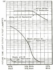
Fig. 8: Actual light output from the face of a picture tube under both restored and unrestored conditions. White and black input signals held constant. Percentage of white and black areas in picture indicated along the abscissa.
