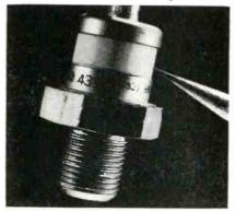
is 50 ma at the rated peak inverse voltage. Features include: operation at high ambient temp. (up to 190°C at the junction); solid copper base for ruggedness; and small size (max. cell length is 3 in.). Weight is 8 oz. Rectifier is nickel-plated and has ceramic insulation. Westinghouse Electric Corp., P.O. Box 2088, Pittsburgh 30, Pa.
