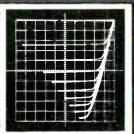
HIGH COLLECTOR CURRENT PNP transistor, collector current vs collector voltage with constant-current base steps. Collector sweep is 0 to 5 v with a 0.25-ohn load, base current is 100 ma/step. Vertical deflection is 2000 ma/div, horizontal 0.5 v/div.
