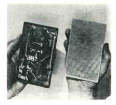
persulfate are used for removing excess copper. Boards are 1/16 in thick and available in 3 sizes:  $3 \times 5$ .  $6 \times 8$  and  $9 \times 12$  in. Components can be soldered to the board more than 50 times without circuit run failure. Fotoceram, a glass-ceramic with high strength, high temp. resistance, and zero water absorption, is non-flammable and dimensionally stable. Electronic Components Dept., Corning Glass Works, Bradford, Pa.
