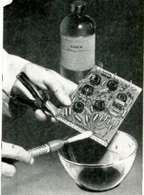
Plating circuit contacts without dismantling electronic components.
