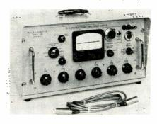
$\mu$ v). The resistor network is controlled by 6 decade switches covering voltage ranges from  $\pm 10 \ \mu$ v to  $\pm 10$ volts. Hallamore Electronics Company, 714 N. Brookhurst Street, Anaheim, Calif.
