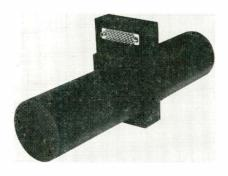
package. Each individual potentiometer can be supplied with its own independent function so that simultaneous control, feedback and telemetry signal can be provided. Specs are: linearity,  $\pm 0.1\%$ ; resistances, 1000 to 100,000 ohms; resolution, as low as 0.03%; power rating, 1.5 w per element; temp. range -65 to  $\pm 200^{\circ}$ F. Bourns, Inc., P.O. Box 2112, Riverside, Calif.
