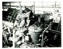
A 5000 lb. high vacuum induction furnace, the only unit of its kind and the world's largest, has been installed by the Metals Div., Kelsey-Hayes, Co., Hartford, N. Y. The entire melting chamber of the furance, designed and built by ASEA, Vasteras, Sweden, tilts to pour. Vacuum is as low as one micron. Ingot size can range from 200 to 5000 lb.
