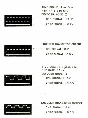
Fig. 10: Waveshapes show the performance of resistor matrix
