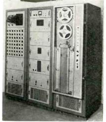
can be direct from any number of channels or from analog magnetic tape recording. Playback speed is a max. of 100 times recording speed. signal frequency is a max. of 600 cycles per sec. The system recognizes and digitizes only during defined voltage peaks, bands, or zones which are established by mathematical criteria. Consolidated Electrodynamics Corp., 360 Sierra Madre Villa, Pasadena, Calif.
