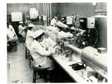
Transistors are now being manufactured in this new "controlled conditions" plant of National Semiconductor Corp., Danbury, Conn. The transistors in production are p-n-p silicon alloy "small signal" types for low power level amplification. Other types are planned for future production.
