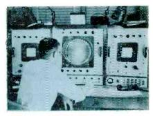
WEATHER RADAR Control console is nerve center for new storm-finding radar at Miami, Fla., Weather Bureau. Antenna system supplied by 1-T-E Circuit Breaker Co. Range is 250 miles.
