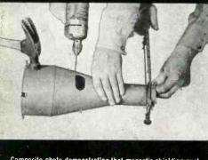
Composite photo demonstrating that magnetic shielding qualities of NETIC alloy material are not affected by vibration, shock (including d.opping) etc. Furthermore, NETIC does not retain residual magnetism nor require periodic annealing.
