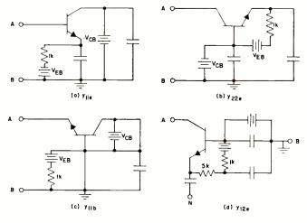
Fig. 3: Circuits for measuring y11e, y22e, y11b and y12e
