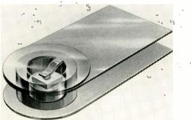
No larger than the head of a match, tunnel diode in RCA developed low-inductance case with integral ribbon measures less than  $\frac{1}{4}$  in. in overall length and has a height of about 1/16 in. Cylindrical ceramic case and ribbon lead-and-tab construction provide an inductance of only 0.4 millimicrohenry. The tiny component is now being offered on a sampling basis by the RCA Semiconductor and Materials Division for engineering evaluation.
