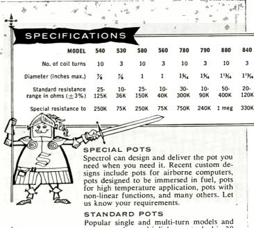
Popular single and multi-turn models and turns counting multi-dials are stocked in 30 electronics supply houses in the U. S. and Canada. Ten resistance ranges from 100 ohms to 200 k ohms with standard linearity tolerances of  $\pm 0.3\%$  are available.
