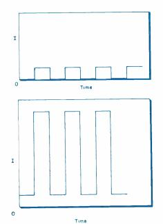
Fig. 17 (left): Pattern of square wave pulses used in measuring resistance. (top) zero biased low current pulses for initial measurement of forward voltage drop; (bottom) pulse pattern for diode self heating.
