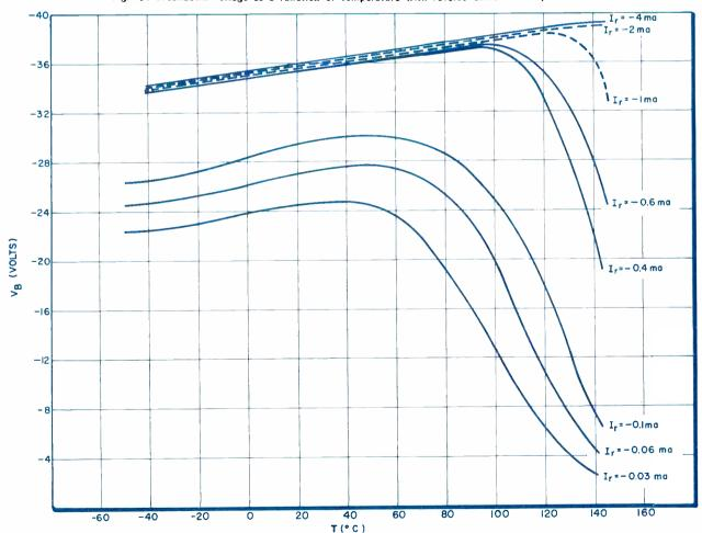
Fig. 15: Breakdown voltage as a function of temperature with reverse current as a parameter.
