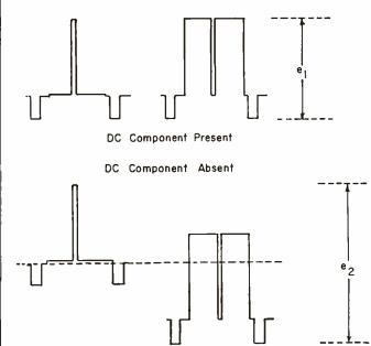
Fig. 7: Graphic illustration of the difference of dynamic range required for DC restored vs. unrestored systems. Peak-to-peak range required is e1 for restored system; e2 for unrestored.
