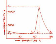
Fig. 1 Permittivity of a dielectric, barium titanate, around Curie temperature.
