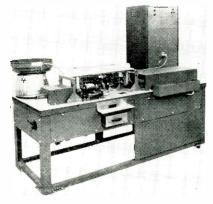
cycle is achieved by a sensitive automatic bridge. Counter provided for presetting turns-per-inch and spindle rpm. Industrial Instruments Automation Corp., 89 Commerce Rd., Cedar Grove, N. J.
