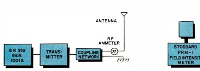
Fig. 5: Radiated field intensity measurements setup
