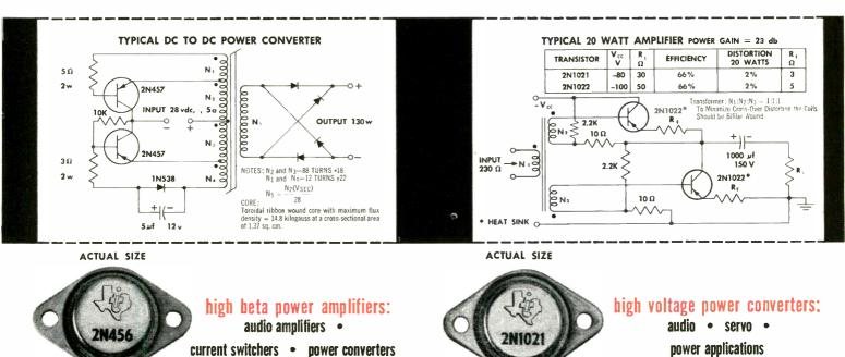
**TI 2N456** series alloy-junction transistors with **guaranteed** 50-w dissipation, **-40**, **-60**, **and -80**  $BV_{CBO}$  ratings and less than 0.048 ohm saturation resistance provide optimum performance characteristics.
