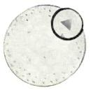
Dislocation density, Knapic silicon monocrystals grown by a modified Czochralski technique: Crystal diameter to  $\frac{3}{2}$ "-None;  $\frac{3}{2}$ " to  $\frac{3}{2}$ "less than 10 per sq. cm.;  $\frac{3}{2}$ " to  $\frac{1}{2}$ "-less than 100 per sq. cm.;  $\frac{1}{2}$ " to 2" less than 1000 per sq. cm.;
