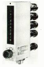
are capable of counting at a 100,-000 cps rate. Specifications input: negative pulse, 75-100v. peak; Rise Time—1 μsec max; Duration —at least 2 μsec; Input Impedance —100 μμf in series with 16,000 ohms; Preset Coincidence Output —positive pulse, approximately 50 v. peak. Computer-Measurements Corp., North Hollywood, Calif. (Ref. No. 11-22).
