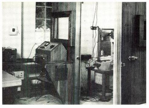
Fig. 2: Steel lined booth with bullet proof windows houses the 130,000 rpm spin rig.
