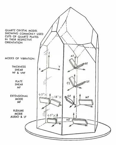
As a guide to circuit designers, this article reviews the various cuts of crystals and their applications in electronic circuits. Testing procedures are described and operational problems are viewed from several highly practical viewpoints. The comparative ability of several crystal oscillator circuits is studied.
