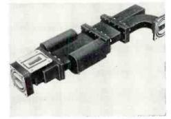
good AFC performance has been developed. Does not need an ATR tube or require use of a high power TR tube. Unit can operate at high power levels. Magnetron to load isolation is a built-in feature. Duplexer has a nominal 1 way insertion loss of 0.5 db over range of 8500-9600 MC. Unit has wide application in all high power radars. Airtron, Inc., Linden, N. J. (Ref. No. 11-3).
