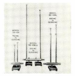
let locks have been added to each stub, permitting quick locking of the tuning position. The relative positions of the 2 stubs is readily adjustable to either of 3 positions, avoiding the impracticability of tuner use experienced when the relative position of both stubs is fixed. Weinschel Engineering, Kensington, Md. (Ref. No. 11-9).
