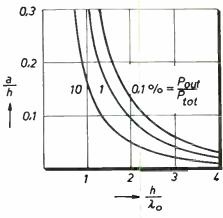
Fig. 4: Guide geometry for energy ratios.
