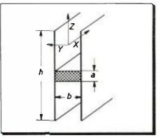
Fig. 6: Cross-sectional view of H-guide
