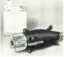
viewing. The new camera is less than 6 in. long, measuring only  $1\frac{7}{8}$  in. in diameter. Equipped with two sets of spring-loaded guide rollers, it travels through pipes that have an I.D. of  $2\frac{3}{8}$  in. or more, and a bending radius of a mere 14 inches. This remote-controlled unit contains a miniresistron and a number of subminiature tubes that serve as amplifying elements. Majestic International Corp., Chicago (Ref. No. 11-45).
