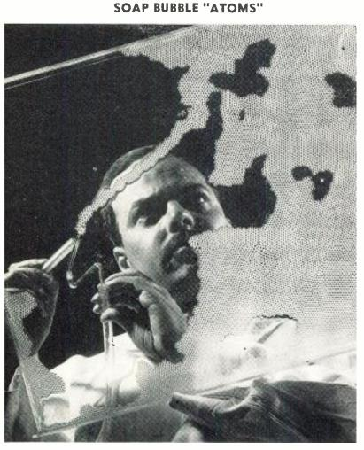
Dr. Wm. Mullins of Westinghouse Research Labs illustrates with soap bubbles how atoms group themselves into orderly "crystal structures." "Bubble" technique permits scientists to investigate on a vastly larger scale the patterns and defect structures formed by atoms in nature.
