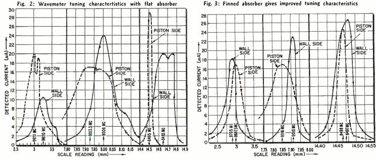
Fig. 2: Wavemeter tuning charactertistics with flat absorber
