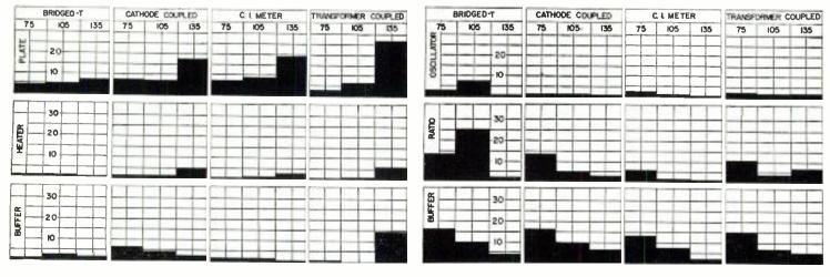
Fig. 6: Relative frequency stability merits of 4 oscillators
