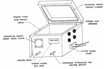
Fig. 1: Design features of effectively shielded enclosure.
