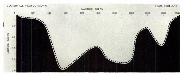
Contour of ocean bed where cable swiftly and clearly carries 36 conversations simultaneously. This is deep-sea part of system – a joint enterprise of the American Telephone and Telegraph Company, British Post Office and Canadian Overseas Telecommunications Corporation.
