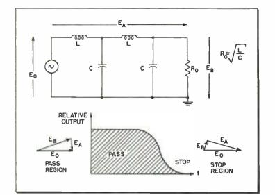
Fig. 1: Low-pass filter and output characteristic
