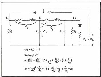
Fig. 2: Two-section single-ended balanced discriminator
