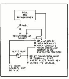
Diagram for carrier alarm circuit.
