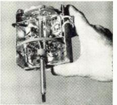
strips, antenna and osc. circuits are located on 2 disks or rotors connected by a tuning shaft. Eventually it will be incorporated in the new 10-, 14-, and 17-inch portables. Admiral Corp., Chicago (Ref. No. 11-28).
