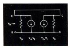
Fig: 1: Collector shorted to emitter for determination of fwd. transfer admittance
