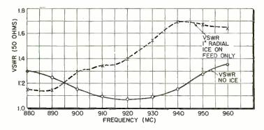
Fig. 2: (above) VSWR for normal operation and for operation with 1 inch ice load on the active element
