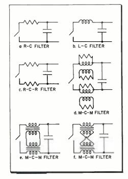
Fig. 5: Switching transient filters.
