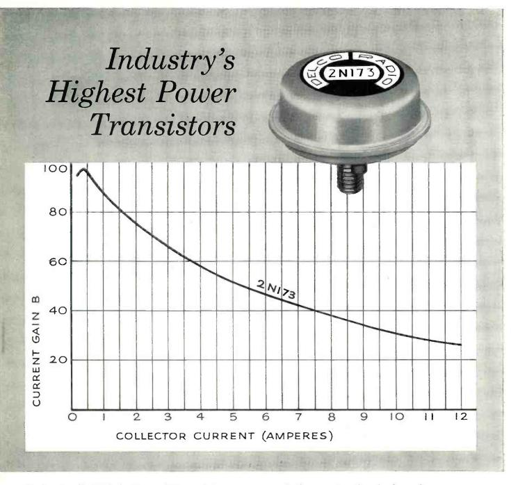
Delco Radio "High-Power" Transistors set a new industry standard of performance – Produced by the thousands each day !
