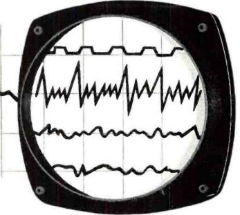
The Beamplexer is actually a fast electronic switch. Its heart is the Burroughs Beam Switching Tube which acts as a gate, picking the ten parallel input signals off in sequence, at adjustable speeds ranging from push button to 100 kc, and putting them out on one line. Each signal can be located on the scope as desired, and even superimposed on one another through individual positioning pedestal controls for each channel. Other controls include separate amplification for each channel.
