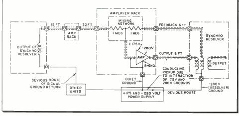
Fig. 3: This circuit developed high noise level due to magnetic and inductive pickup troubles
