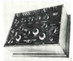
brate four-arm systems without the necessity of complicated hookups. All loads applied to a transducer are read directly in force. acceleration, torque, pressure, etc., and the usual tedious arithmetic is eliminated in a linearity check. Accuracy of the instrument is  $\pm 0.05$  per cent while total thermal EMF is less than 3 pv. Allegany Instrument Company, Metuchen, N. J. (Ref. No. 11-19).
