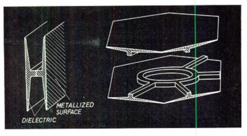
material would fill the space between the walls. Both have different values if the cross-sectional structure is composed of different materials, as is the case in the H-guide. In this guide, the actual guide wave length is reduced by the influence of the dielectric slab. On the other hand, it is greater than it would be in a guide completely filled with the dielectric of the slab.
