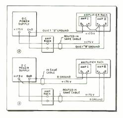
Fig. 2: Separate ground return reduces noise
