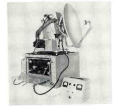
is speeded by the provision of 2 azimuth positions. Modulation consists of a 1 µsec pulses at rep rate of 1000/sec. Specs: 24 in. parabola, 33 db gain, & 3.5° beam width. Color Television, Inc., San Carlos, Calif. (Ref. No. 11-5).
