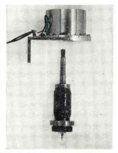
Fig. 4: Rotating secondary and stationary primary of information coupling xformer.
