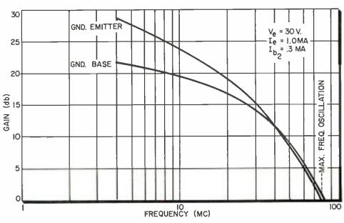
Fig. 2: Common emitter configuration is more advantageous for higher transistor gain
