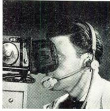
3.3 KC. A boom mounted carbon microphone is provided. Movement of the arm is restricted by stops to 90 degrees allowing adequate adjustment when in use. Amplivox Ltd., London, England. (Ref. No. 11-47).
