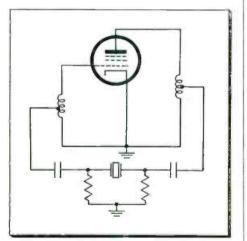
Fig. 10: Transformer coupled Osc.
