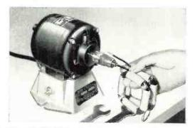
This Model "L-2" Wire Stripper strips Formex and similar insulations from ends of solid (not stranded) wires from AWG #29 to AWG #6—cleanly, with-out nicking or abrading the wire. It can be testrented for one month for only \$11.00.
