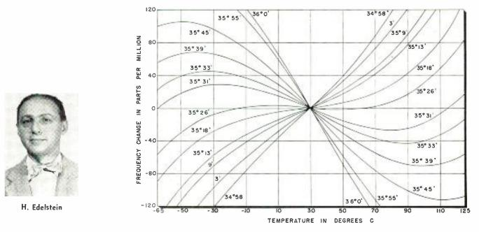
Fig. 2: Frequency-temperature characteristics of an AT cut resonator.
