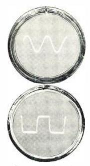
Photos show single transient pulses, 20 microseconds wide with a one microsecond rise time, showing writing capabilities of one million inches per second. These photos were taken in full daylight without a hood.
