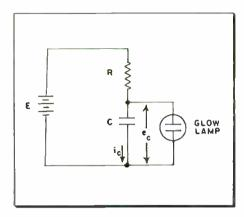
Fig. 3: RC-glow lamp relaxation circuit
