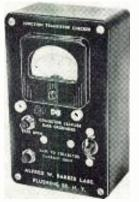
reads gain directly. Pin jacks connect to base emitter and collector circuits for plugging in clip leads. \$31.50. Instant Circuits, Div. of Alfred W. Barber Labs. ELEC-TRONIC INDUSTRIES & Tele-Tech (Ref. No. 10-14).
