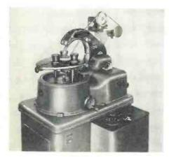
pitch control and special manual feeding attachment for hand winding. Models U-9, U-14, and U-20, to wind tape from 3% in. to 1 in. Universal Manufacturing Co., Hillside, N. J. ELECTRONIC IN-DUSTRIES & Tele-Tech (Ref. No. 10-19).
