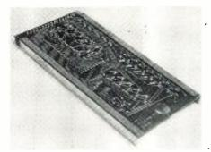
Fig. 2: Typical Formica XXXP-36 P-C board
