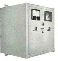
This is a high voltage power supply for electrostatic dust collecting and air conditioning equipment. Operating on 230 volt single phase, 60 cycle, it supplies 12 KV direct current up to 30 ma. D.C. voltage is adjustable to load.
