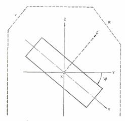
Fig. 1: Quartz bar orientation for YZ flexural mode
