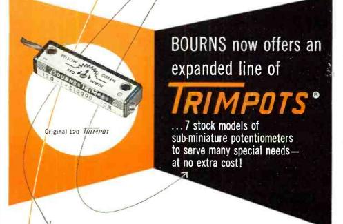
First there's the 120 Wirewound  $\overline{RimP0T}$ , with features common to all other BOURNS  $\overline{RimP0Ts}$ . It's a 25-turn potentiometer, easily adjusted, and weighing only 0.1 oz. Rectangular in shape, it fits readily into miniature electronic circuits. You can mount it individually, or stack it compactly with standard screws. Mountings are interchangeable with those on all other  $\overline{RimP0Ts}$ .
