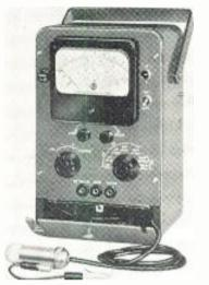
DC voltmeter with 100 megohms input resistance; and an ohmmeter capable of measuring resistance from 0 to 1000 megohms. Accurate measurements to 700 mc, and voltage measurements as high as 32.000 v DC and 1600 v AC. RCA, Camden, N. J. ELEC-TRONIC INDUSTRIES & Tele-Tech (Ref. No. 10-13).
