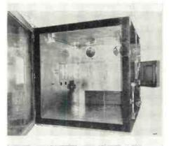
ture changes. This low-temperature test chamber has a range of  $-100^{\circ}$ F to  $+220^{\circ}$ F ( $+2^{\circ}$ F); relative humidity range of 20% to 95%, 35°F to 180°F, 35°F minimum dew point; special operation of 5% to  $+160^{\circ}$ F; heat dissipation load of 30,000 BTU/hr. at  $-70^{\circ}$ F. Tenney Engineering Inc., Union. N. J. ELECTRONIC IN-DUSTRIES & Tele-Tech (Ref. No. 10-23).
