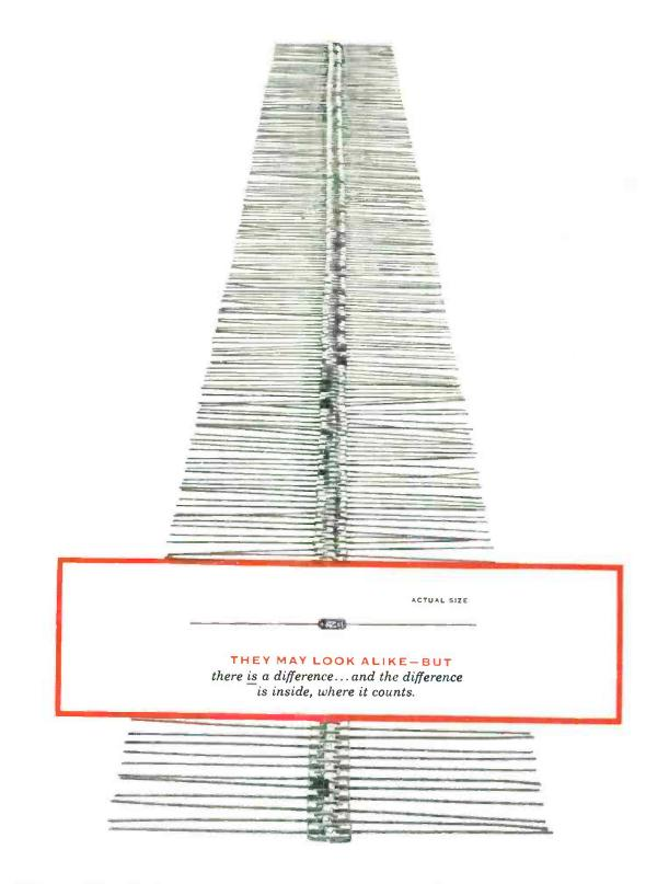
All Hughes diodes resemble each otherexternally. Germanium point-contact or silicon junction, they are all glass-bodied<sup>°</sup> and tiny (actual dimensions: 0.265 by 0.105 inch). But minute, meticulously controlled variations in the manufacturing process impart individual characteristics to the diodes, make them just right for specific applications. This gives you the
