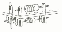
tion has a narrow tapered slot with serrated edges, which firmly grip the wire lead of any size between 0.030 and 0.045 in. Vector Electronics Co., Los Angeles. ELECTRONIC INDUSTRIES & Tele-Tech (Ref. No. 10-5).
