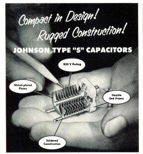
The Johnson Type "S" capacitor falls midway between the type "M" and "K" capacitors in physical size. Design is compact, construction rugged! End frames are DC-200 treated steatite—plates are nickel-plated brass. Avail-able as a "single" type, the "S" capacitor has a plate spacing of .013" with a peak voltage rating of 850
