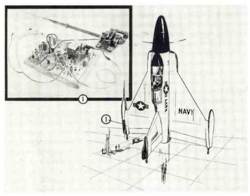
Fig. 1: 10 KMC doppler unit guides XFY-1 "Pogo-Stick" landing
