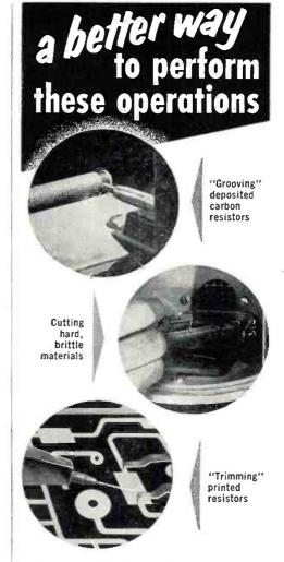
It's the "Airbrasive" way – the method that uses gas-propelled abrasive to do the work. There's no heat, shock or vibration. The cutting is always constant and can be controlled to remove extremely minute amounts of material. SEND US YOUR PARTS and an outline of your requirements for trials. We'll be glad to make recommendations.
