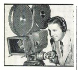
Auricon 16 mm SOUND-ON-FILM "SUPER 1200" CAMERA with Full-Frame Reflex Ground-Glass FOCUSING OPTICAL SYSTEM
