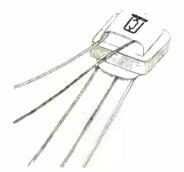
plied with 4 in. color coded leads suitable for use in dip soldered printed circuits. Molded nylon bobbins, high-nickel laminations. and Mylar insulation are used to permit maximum size reduction. Primarily designed for transistor circuitry in guided missiles and airborne equipment. Stock units also available for single-ended and vacuum tube applications. Microtran Co., Valley Stream, N. Y. ELECTRONIC INDUSTRIES & Tele-Tech (Ref. No. 10-7).
