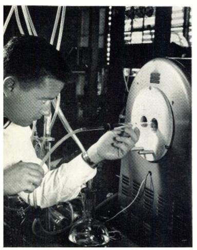
Germanium blanks for Philco's new surface-barrier diffused (SBDT) transistors are shown being prepared by engineer R. A. Williams. New process in which particles of metal are diffused into germanium surface results in transistors operating up to 500 MC.
