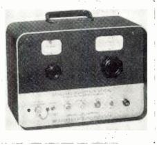
network of the Model 202-C contains a Bolometer which produces a resistance unbalance proportional to the signal. Measurements Corp., Boonton, N. J. ELEC-TRONIC INDUSTRIES & Tele-Tech (Ref. No. 10-18).
