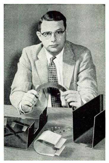
R.F. Bogart, one of National's staff of applications engineers, shown holding a postformed copper clad PHENOLITE printed circuit.
