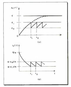
Fig. 4: Condenser voltage (a) and current (b)
