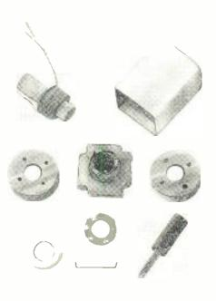
forms were attached and wired to a mica filled phenolic (melmac) combination base and electrical terminal block.
