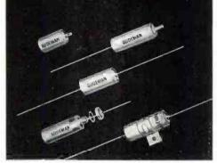
The development of the Gudeman "XC" capacitors results in a new line of high temperature capacitors that has exceptionally high insulation resistance, low power factor and low dielectric absorption. The case sizes were selected whereby no voltage derating is required when the capacitors are used within a temperature range from  $-65^{\circ}$  C. to  $+165^{\circ}$  C.
