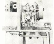
number up to 1000. The machine then counts, marks, and ejects automatically all circuit plates placed in the magazine. The ejector in turn replaces the marked plates in another magazine, all in perfect sequence. Speed is 3600 marked plates per hour. Acromark Co.. Elizabeth. N. J. ELECTRONIC INDUSTRIES & Tele-Tech (Ref. No. 10-2).
