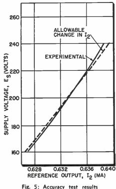
a limiting value which requires a supply voltage of infinity. Thus, the current output of this type of reference is limited, but it may be increased by increasing  $\varepsilon$ , reducing  $\Delta E_s/E_s$ , making  $I_{1 \min}$  smaller or using a different diode. If the reference is being designed for maximum output current, a plot of  $E_s$  versus  $I_2$  may be made and the largest practical value of  $I_2$  selected from the curve.
