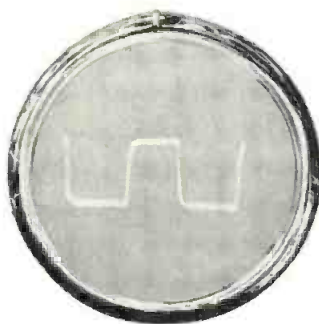
Single transient pulse, 20 micro-seconds wide with a one micro-second rise time, showing writing capabilities of one million inches per second. This photo was taken in full daylight without a hood.
