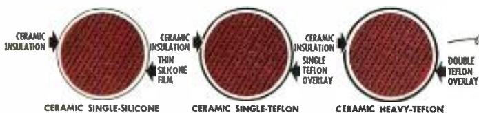
ENLARGED CROSS-SECTIONS OF CEROC® COPPER MAGNET WIRE
