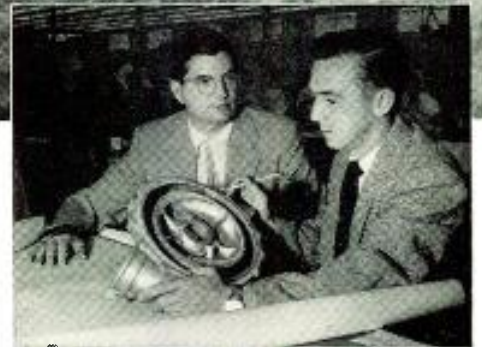
AiResearch two stage lightweight gas turbine compressor provides pneumatic power for aircraft main engine starting and serves as auxiliary power source for a variety of ground and in-flight services.
