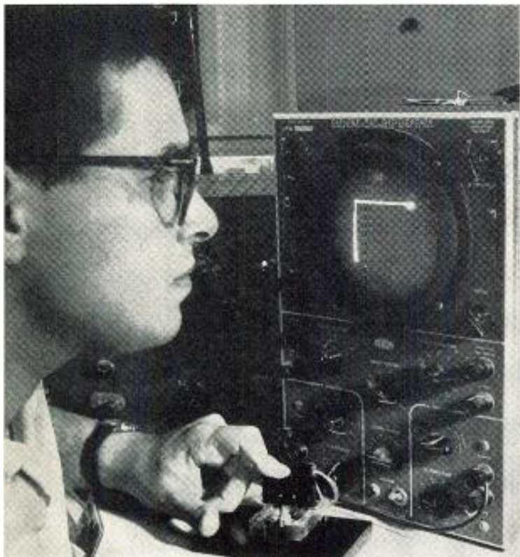
Bell Labs' Dr. H. S. Veloric checks a new diffused junction silicon "avalanche" diode, so-called because it exhibits a very sharp reduction in impedance at a certain specific inverse voltage. New units find application in voltage regulation or control devices.
