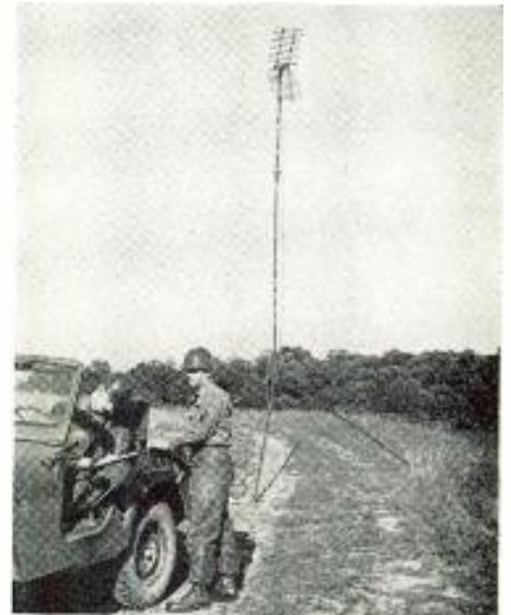
This Signal Corps "radar ruler," used for great distances, enables a surveyor to survey 50 miles at a time accurately and in any weather.
