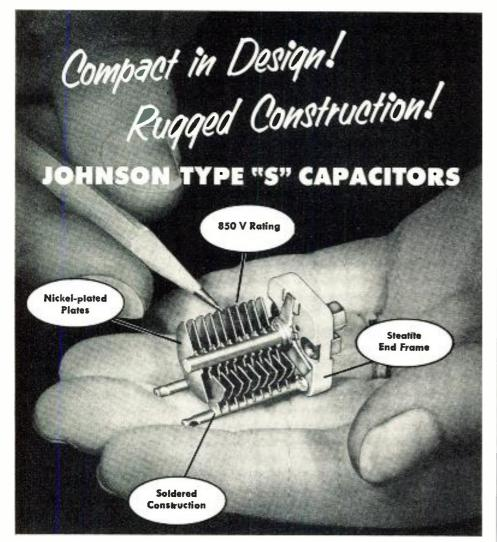
The Johnson Type "S" capacitor falls midway between the type "M" and "K" capacitors in physical size. Design is compact, construction rugged! End frames are DC-200 treated steatite—plates are nickel-plated brass. Available as a "single" type, the "S" capacitor has a plate spacing of .013" with a peak voltage rating of 850
