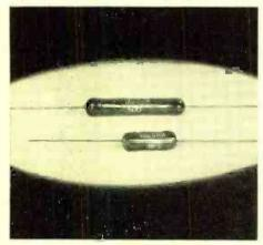
tance; the junction of the resistance element is silver brazed and then coated with vitreous enamel which is then fired at high temp. This unit is capable of continuous operation at 300° C. They are offered in 3, 5 and 10 watt sizes. Tru-Ohm Products Div. of Model Engineering & Mfg. Co., 2800 N. Milwaukee Ave., Chicago, Ill. Tele-Tech & ELECTRONIC INDUS-TRIES (Ask for 7-148)
