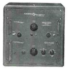
**Model TMC-211** Panoramic Simultaneous 11-Point Calibrator is an instrument especially designed to calibrate the FM/FM Telemetering Subcarrier Discriminator linearity simultaneously, accurately, quickly and conveniently. Eleven equally spaced frequency points are provided within the  $\pm 71/2\%$  or the  $\pm 15\%$  limits.
