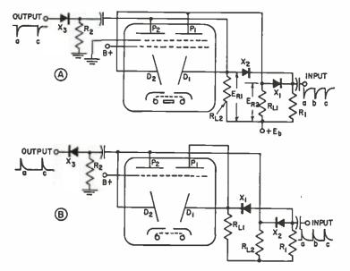
Fig. 1: Unipolar pulse binary counters using primary (A) or secondary (B) emission Bistable operation with voltage increments as low as .66 v. is possible with a new twin target vacuum tube. The tube has use as high speed binary counter, oscillator, flip-flop and cascade dc amplifier
