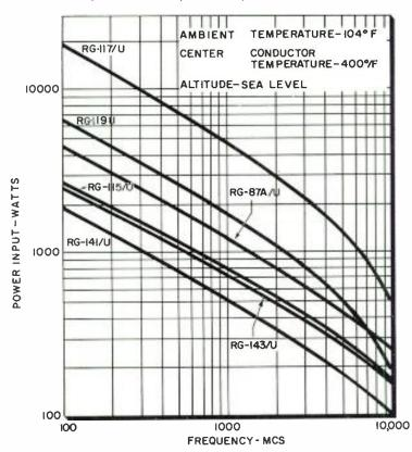
Fig. 2A: Power input vs. freq. of teflon cables
