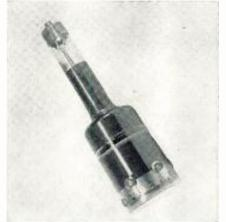
indefinitely, until they are intentionally erased. Traces that exceed the maximum writing speed of the tube can be visibly displayed by repeated retracing at repetition rates sufficiently high to produce cumulative storage. Hughes Products, Div. of Hughes Aircraft Co., Los Angeles, Calif. TELE-TECH & ELECTRONIC IN-DUSTRIES (Ask for 7-91)
