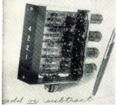
The internal gating is a unique circuit employing reliable longlife neon bulbs. Read-out is visual in binary coded decimal and electrical by a "staircase" voltage indicating the count. Max. continuous speed 50,000 cps. Controller Instrument Co., 1612 Que St., N.W., Washington, D. C. Tele-Tech & ELECTRONIC INDUSTRIES (Ask for 7-147)
