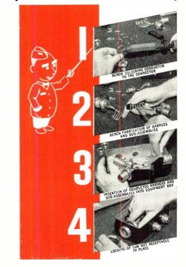
Jam nut receptacles offer such positive savings in assembly time that it will pay you to check into their application on your product. These receptacles permit bench wiring of harness and sub-assemblies prior to final installation with proven savings in assembly labor.
