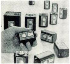
tude, and phase reversible. No DC power supplies are necessary for operation of the amplifiers and their transistor or tube control circuit. Ambient temperature range: --55°C to 100°C. Standard output ratings: 3, 6, 10, 16 and 40 watts. Timely Instruments & Controls Corp., 1645 W. 135th St., Gardena, Calif. Tele-Tech & ELECTRONIC INDUSTRIES (Ask for 7-192)
