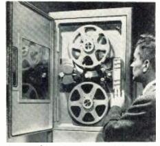
changeable plug-in amplifiers for Direct. FM, and PWM types of recording and reproduction. Instrumentation Div., Ampex Corp., 934 Charter St., Redwood City, Calif. Tele-Tech & ELECTRONIC INDUSTRIES (Ask for 7-7)
