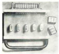
isting electronic circuit into separate component stages. Average dimensions: .313 x .717 x .312. Acoustical Electronic Laboratories. 3785 Broadway, New York 32, N. Y. Tele-Tech & ELEC-TRONIC INDUSTRIES (7-176)
