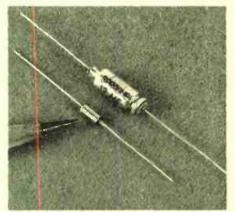
required. In its smallest version shown here, it is only  $\frac{1}{3}$  in. in diameter by  $\frac{1}{4}$  in. long. It occupies 1/10 the volume of the miniature aluminum electrolytic condenser shown behind it. It will find immediate use in the most severe military electronic applications. Sprague Electric Co., North Adams, Mass. Tele-Tech & ELECTRONIC INDUS-TRIES (Ask for 7-11)
