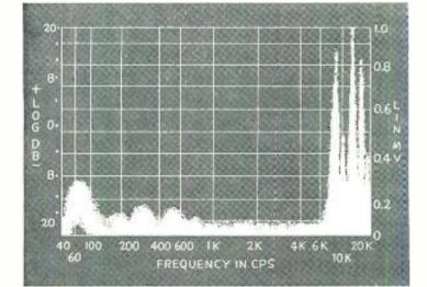
Fig. 3: Noise at 60 cps vibration
