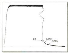
Fig. 5: Recovery time components
