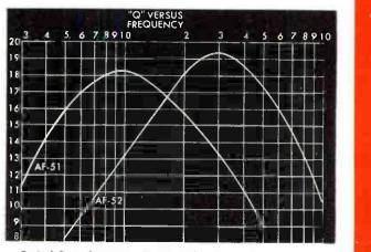
Typical Q vs. frequency characteristics of Variable Inductors.
