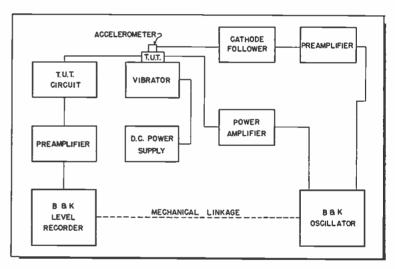
Fig. 1: "Swept frequency" test
