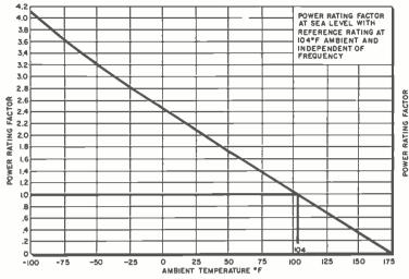
Fig. 5: Power rating vs. ambient temp. for polyethylene
