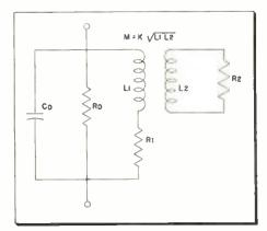
Fig. 4: Eddy losses shunt yoke
