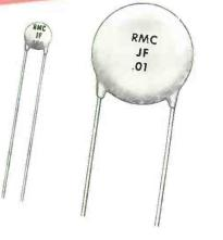
Type JF DISCAPS have outstanding frequency characteristics over a wide range of capacities and incorporate desirable temperature properties over an extremely useful range. Manufactured in capacities from 150 MMF to 10.000 MMF, Type JF DISCAPS extend the range of the RETMA Z5F capacitor between  $\pm 10^{\circ} - \pm 85^{\circ}$ C and meet Y5S specs from  $\pm 30^{\circ}$  to  $\pm 85^{\circ}$ C. (See graph)
