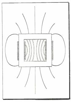
Magnetic deflection fields are affected by coil form, winding style, and external environment in the form of core, case, and other external components. The author discusses the many factors involved in deflection yoke efficiency and fast recovery time
