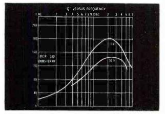
Typical Q vs frequency characteristics of Adjustoroids.
