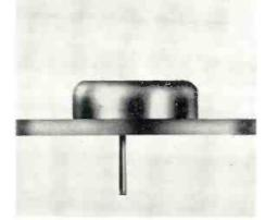
Class B operation, will provide 10 watts at less than 10% distortion from a 12 volt supply at 80°C. Motorola, Inc., 4545 Augusta Boulevard, Chicago 51, Ill. Tele-Tech & ELECTRONIC INDUSTRIES (Ask for 7-83)
