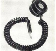
oz. With a 40 ohms impedance, and a frequency response in the 200 to 5,000 cps range, the mike should be used as a close talking unit. Elgin National Watch Co., Elgin, Ill. Tele-Tech & ELEC-TRONIC INDUSTRIES (7-13)
