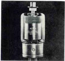
plications where space is limited to that occupied by the 4C35, but where the capabilities of the 4C35 are exceeded. Max. ratings of the PL-165: Peak plate voltage, 12 kv.; peak plate current, 325 a. Max. dimensions: height overall, 6.25 in.; seated height, 5.63 in.; diameter, 2.56 in. Penta Laboratories, Inc., 312 N. Nopal St., Santa Barbara, Calif. Tele-Tech & ELEC-TRONIC INDUSTRIES (Ask for 7-58)
