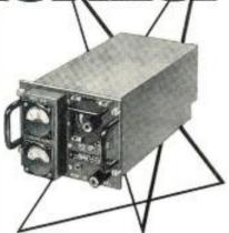
SPECIFICATIONS SPECIFICATIONS Frequency Range: 215 to 235 mc. Crystal Stability: ±0.005% Frequency Deviation: ±150 kc maximum Selectivity: 50 db minimum rejection of imoge frequency and IF frequencies Sensitivity: 20 db minimum quieting at input level of 6 microvolts (noise figure: less than 7 db) IF Band Width: 350 kc minimum AFC: high gain—appraximately 50 Size: 5¼' x 4½'' x 11½'' Weight: 10 lbs.
