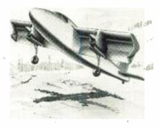
New "Vertiplane," to be built for the Army by Ryan Aeronautical Co., achieves vertical takeoff and landing by the deflected slipstream principle, using retractable wing flaps
