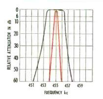
**MECHANICAL FILTERS** (Developed and mfd. by Collins Radio Co.) The Mechanical Filter provides far better bandpass selectivity in one small sealed unit than a series of bulky conventional IF transformers. Excellent characteristics allow closer spacing of information channels, lower adjacentchannel interference and improved signal to noise ratios. These Filters have been proven in thousands of military and commercial receivers, transmitters and microwave multiplex systems.
