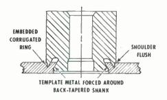
matic. Bushing holes are held to tolerances of drill size plus .0001 min. to drill size plus .0005 max. Penn Engineering & Manufacturing Corp., Doylestown, Pa. 'fele-Tech & ELECTRONIC INDUS-TRIES (Ask for 7-25)
