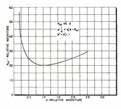
Fig. 1: Experimental curves for wire loss
