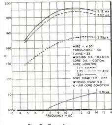
Fig. 9: Q vs frequency
