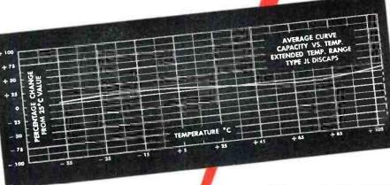
RMC Type JL DISCAPS feature exceptional temperature stability over an extended range. The maximum capacity change between  $-60^{\circ}$  and  $\pm 110^{\circ}$ C is only  $\pm 7.5\%$  of capacity at 25°C. With a standard working voltage of 1000 V.D.C., Type JL DISCAPS are the ideal cost saving replacement for paper and general purpose mica capacitors.
