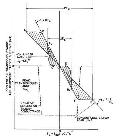
Fig. 4: Non-linear load line operation
