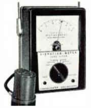
range, uses two ordinary 22½ v. dry batteries to provide power. This all-transistor design alleviates the problem of microphonics (an important consideration in jet-engine testing where high noise levels are encountered. Consolidated Electrodynamics Corp., 300 N. Sierra Madre Villa, Pasadena, Calif. Tele-Tech & ELEC-TRONIC INDUSTRIES (7-4)
