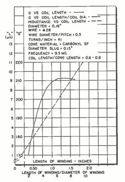
The total copper losses of the winding can be expressed as indicated below for the length of wire will remain constant for a given winding.
