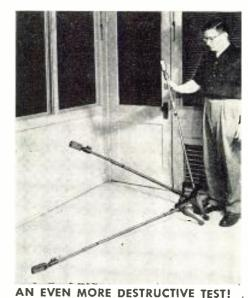
The identical microphone, mounted on a floor stand, was crashed onto the bare floor. This was done six times—still no noticeable change
