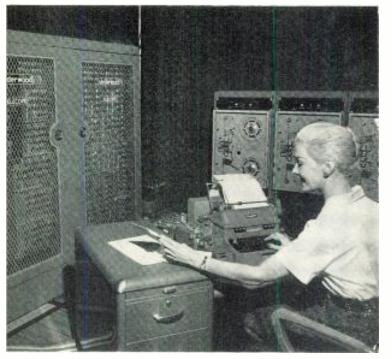
Newest in the line of electronic office equipment is this Underwood "ELECOM" File processor which reduces the contents of 1600 conventional file cabinet drawers to less than 3 cu. ft. of space. The unit also feeds desired information via tape to a companion computer.
