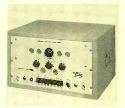
ever is greater. Other inherent characteristics: excellent degree of stability, low ripple present in output voltage, and low impedance. Output voltages delivered are from 10 to 310 v. in 1 v. steps, continuously variable between steps, at 150 ma.; from 0-150 v. continuously variable at 5 ma. and 6.3 volts at 3 am. center tapped, unregulated. Oregon Electronics, 2232 E. Burnside St., Portland 15, Ore. TELE-TECH & ELECTRONIC INDUSTRIES (Ask for 4-18)
