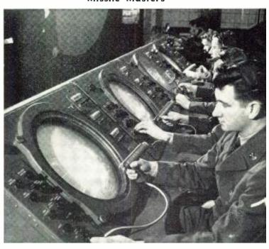
Electronic consoles, similar to these radar entry consoles in the system at Ft. Geo. G. Meade, Md., are heart of the new Martin "Missile Master" system which controls and coordinates NIKE antiaircraft missile batteries. Systems will be located at key antiaircraft installations throughout the country.
