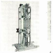
based on the insertion of a germanium or silicon seed into a similar molten metal, forming single crystals by the rate-growing process. Machines can be supplied in all sizes and types and with or without automatic programming. Kahle Engineering Co., 1300 Seventh St., North Bergen, N. J. TELE-TECH & ELECTRONIC INDUSTRIES (Ask for 5-20)
