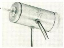
ertia is 2.85 gm.-cm<sup>2</sup>. The device consists of a size 11 2-phase 2-pole servo motor and a drag cup type tachometer integrated into a single compact homogeneous unit 1.03 in. max. dia. by 2.156 in. long and weighing 4.6 oz. Motor portion has 26v. 400 cycle input, .26 oz.-in. stall torque min., and 12.5 w. stall wattage. John Oster Manufacturing Co., Racine, Wis. TeleTech & ELECTRONIC INDUSTRIES (Ask for 5-1)
