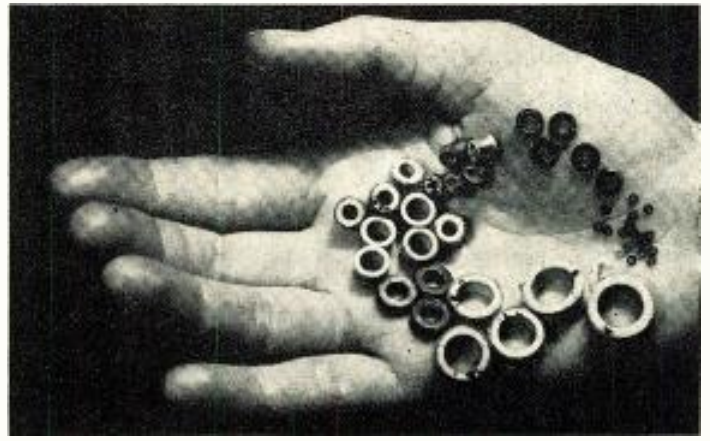
Fig. 1: Bistable ferromagnetic elements exist in 2 basic forms—microthin metallic tape and molded ferrites
