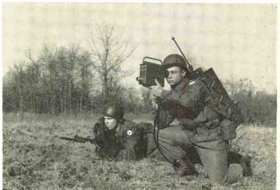
Shown in action is the new 55-lb. remote telecasting unit developed for the Army by Signal Corps Engineering Labs. Completely self-contained, the unit will transmit up to ½ mi. Power is supplied by rechargeable 5-cell silver zinc batteries. Camera weighs 8 lbs., and includes 4 lenses, including wide angle and telephoto. Soldier at left is providing audio report over handie-talkie phone.
