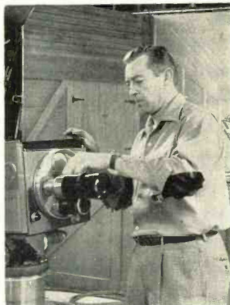
Fig. 7: Removing the camera lens turret
