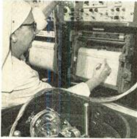
Sensitive gyroscopes, heart of new supersonic pilot for jet planes developed by Minneapolis-Honeywell, are put through "wobble test." Drift rate recorded must be less than .35° per minute.
