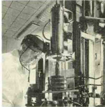
Physicist in Delco Radio Div.'s Semiconductor Lab is shown studying the growth of a large germanium crystal. In 5 hrs. the crystal will be 11 in. long, 1½ in. thick, and worth $3,000
