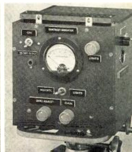
Figs. 2 & 3: Rear and front views of instrument. Contrast is read in percent change of indication
