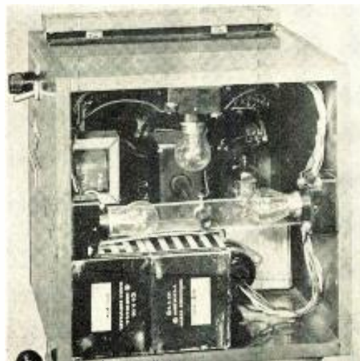
Figs. 2 & 3: Rear and front views of instrument. Contrast is read in percent change of indication
