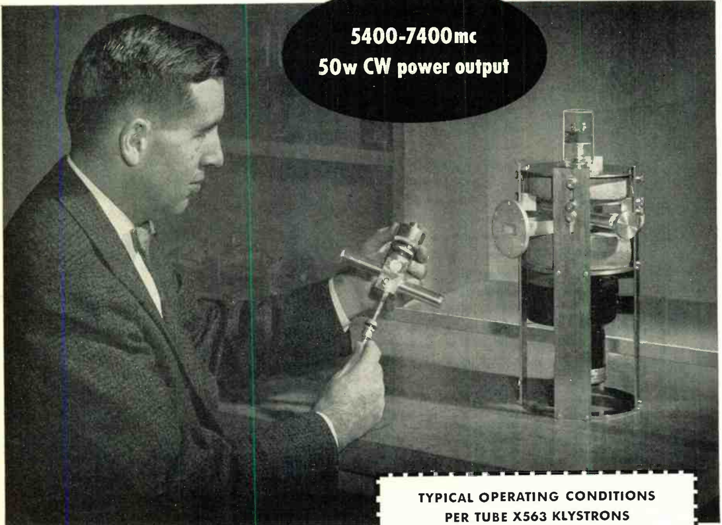
Eimac X563E, 5900-6400mc, and amplifier circuit assembly.
