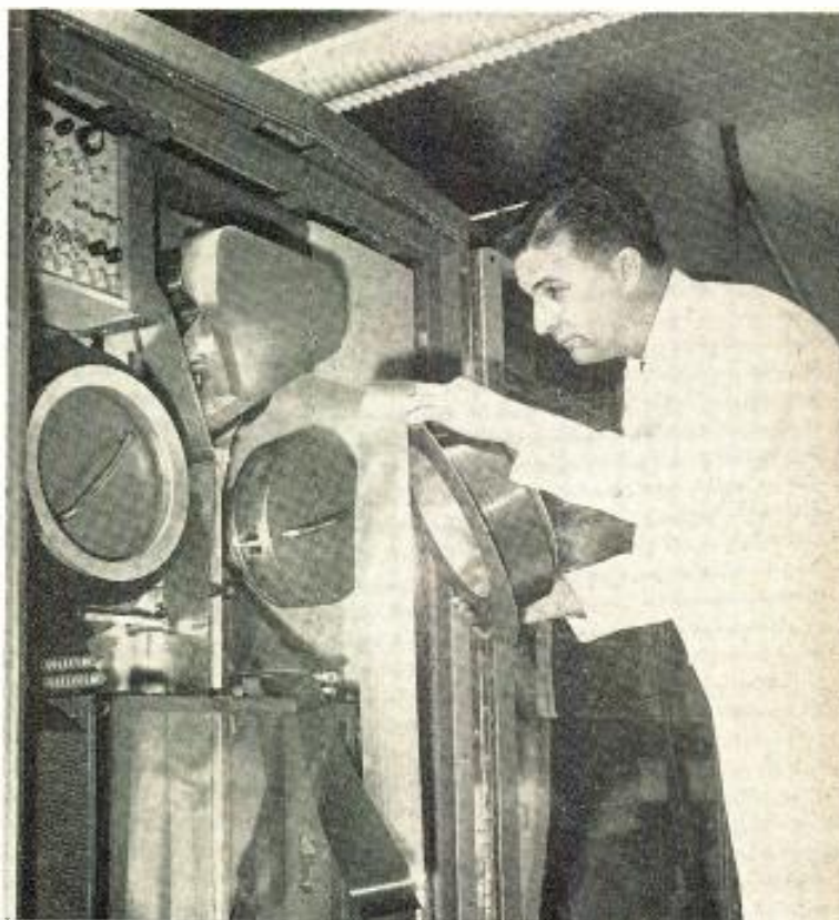
Single 2,700-ft. spool of magnetic tape shown being threaded into one of the 100 file units in the new "Datamatic 1000" computer by engineer Bob Wilkins, can store as much data on its 31 channels as can be found on a half-million punched cards.
