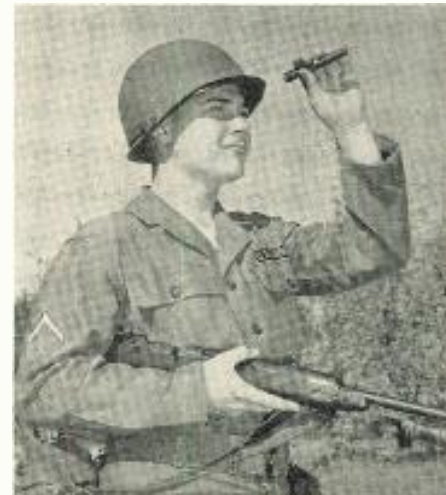
Soldier takes a quick reading of amount of gamma rays he absorbed from radioactive source
