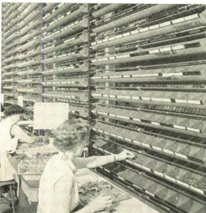
"Ferris wheel" arrangement of parts bins which move up or down by flip of a switch is used to speed assembly of military units at G-E's plant in Utica, N. Y. System was developed for specific needs of joblot military electronics assembly work. "Ferris wheel," with 3,000 bins, occupies 150 sq. ft. of floor space
