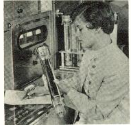
Pilots will see in the dark with daylight clarity with this new tube developed by the AF and Westinghouse. The tube is approx. 1,000 times more sensitive than the standard TV camera.
