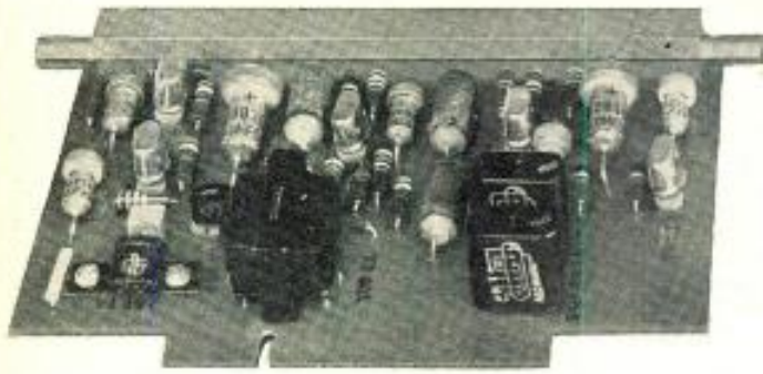
Fig. 1: Transistorized, printed circuit summing amplifier
