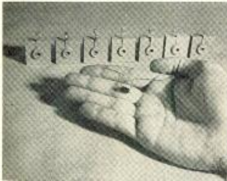
New silicon power rectifier in foreground developed at Bell Telephone Labs does same job as seven selenium units shown in rear
