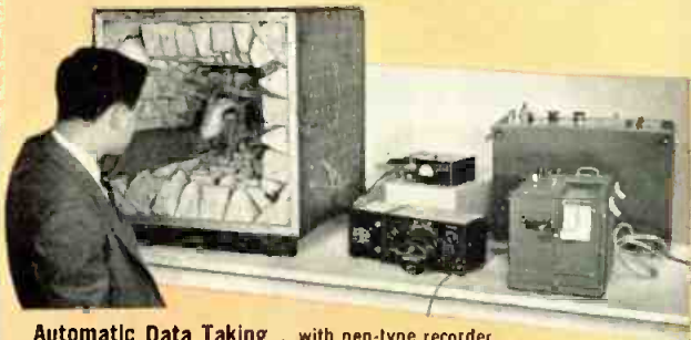
Automatic Data Taking . . . with pen-type recorder or CRO eliminates laborious point-by-point measurements . . . in photo, frequency response of small loud-speaker is recorded.
