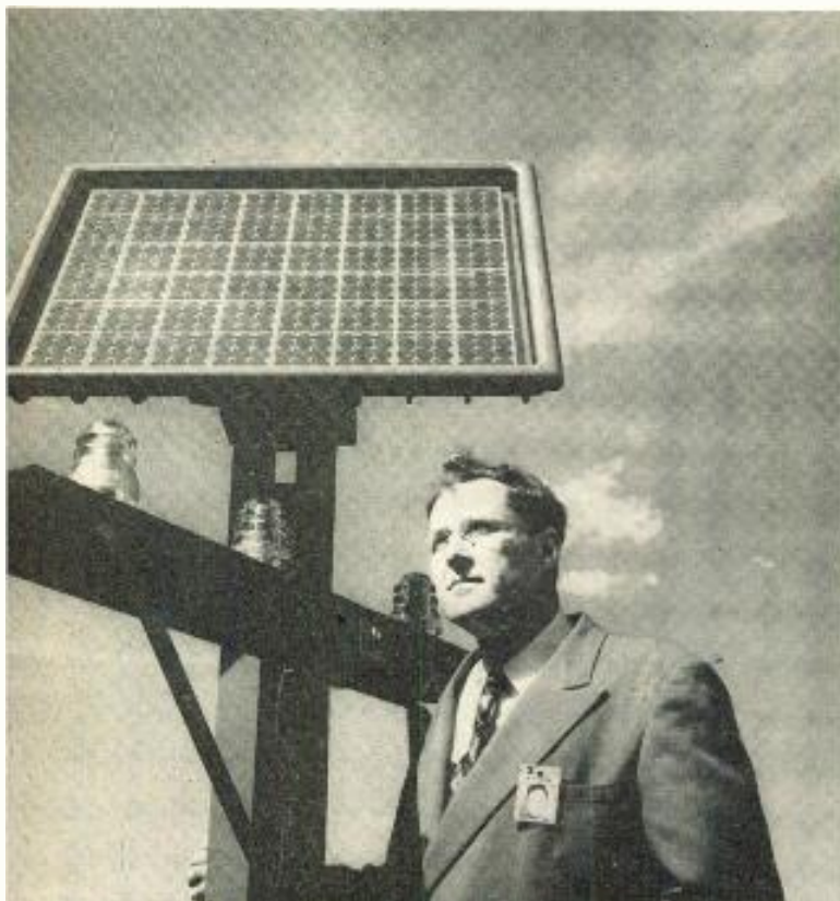
Bell Telephone Labs engineer, W. D. Gerdson, with a model of the Bell Solar battery mounted on a section of telephone pole. The solar battery is receiving its first practical test as part of the telephone system this summer in an experimental unit—essentially identical to the model shown—installed in Americus, Ga., to supply power to terminal equipment on rural telephone lines. During daylight hours the battery will power terminal equipment directly, and at the same time charge a storage battery to provide power for nighttime operation.
