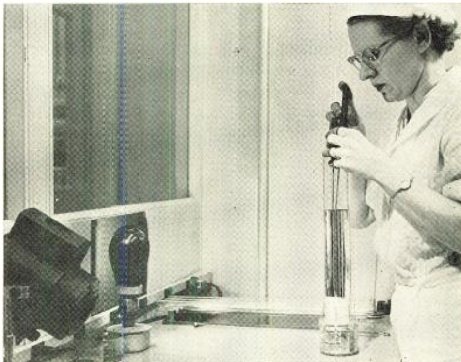
Factory production of image orthicons is now under way at GE's Schenectady tube plant. Here operator is shown adjusting target and mesh section in tube using 17-in. screwdriver. Previously RCA was sole producer.
