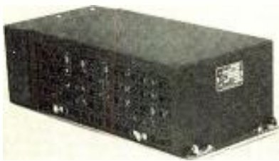
Fig. 6: Complete assembly of transmitter, receiver and power supply in metal housing
