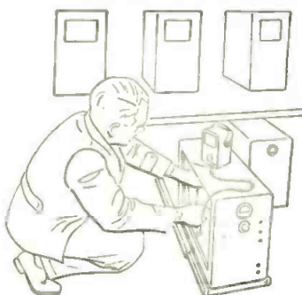
Picture distribution amplifier unit, synchronizing generator and power supply units are mounted on Grant Industrial Slides. Units are normally retracted but roll out for servicing and maintenance.
