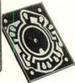
Switch plates, commutator discs, and drum commutators with printed circuits have proved themselves in many diversified applications. Low-cost printed circuit switches are ideal for simple switching, and show up to best economical advantage in complex switching functions.
