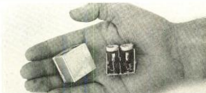
FIG. 5 Miniature i-f transformers employ toroids with Q of 140.
