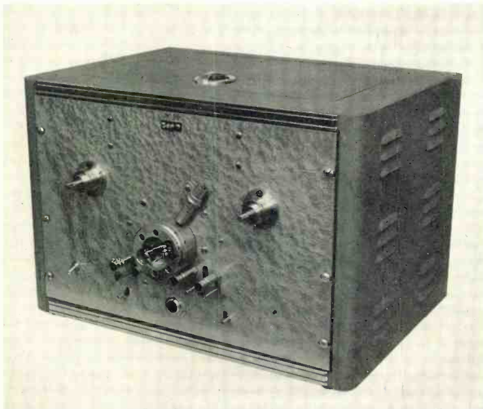
Fig. 1: (Left) Rotating head magnetic tape reader. Studs on front hold reels, guide tape past drum
