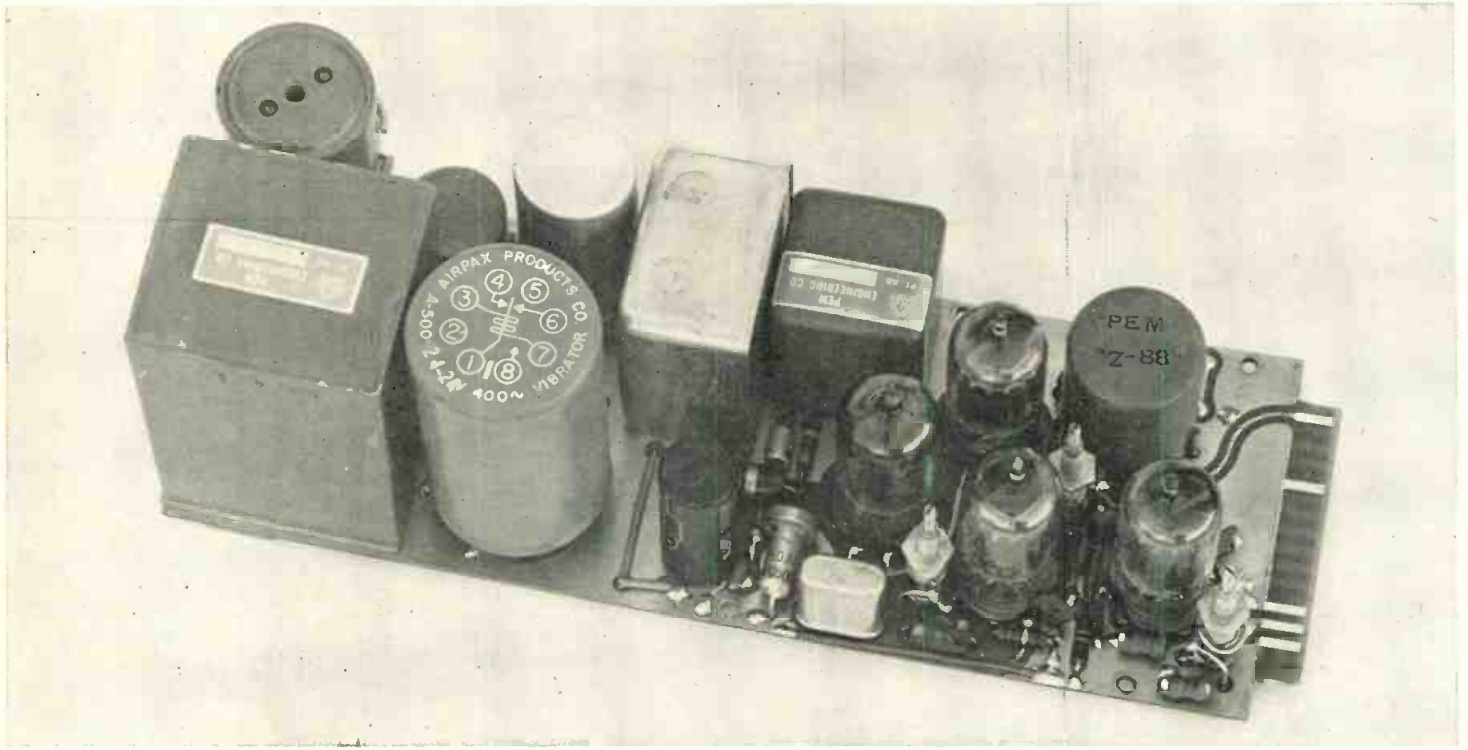
FIG. 1 Complete transmitter and power supply assembly is mounted on a single printed circuit card
