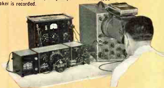
Network Transient Investigations . . . with R-C oscillator square waves; one measurement gives information on both amplitude and phase characteristics . . . in photo, engineer observes and records filter characteristics of G-R Type 1550-A Octave-Band Noise Analyzer.
