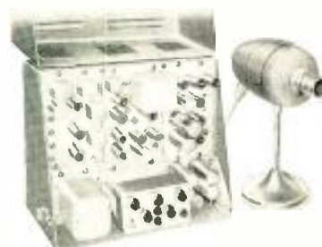
The "Bullet" TV Camera; for industrial, institutional and educational use. Produces useful pictures under conditions of poor light; feeds any TV receiver or monitor; unique packaging permits placement in ordinarily inaccessible areas; unitized construction with plug-in component chassis minimizes maintenance requirements.
