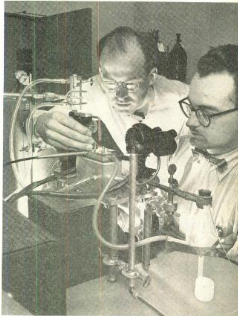
"Meltback" principle of manufacturing transistors, developed at GE by Dr. Robert N. Hall (l), cuts cooling time of crystals to less than 1 sec., permits thinner separating layers—and much higher frequencies of operation. Previous methods had called for 20 min. cooling period, during which impurities migrated from their proper layers to adjoining layers. At right is GE scientist, R. I. Scace.
