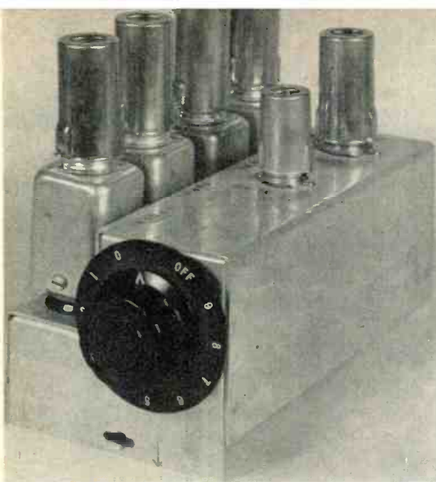
Fig. 1: Decade preset counter used in analog-digital time measuring system
