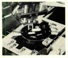
disc type capacitors; jumper wires; tube sockets; and i-f transformers. Included in this system is an advanced method of automatic dip soldering.
