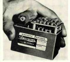
Power requirement, 115 v. 400 cPs, Power consumption; stand-by, 1.0 w., full output, 3.5 w. Input voltage, dc 0-1.0 v. or pulsating. AC, 0-1.0 v., phase angle 60° leading. Librascope, Inc., 808 Western Ave., Glendale, Calif. (Inquiry Card No. 6-14)
