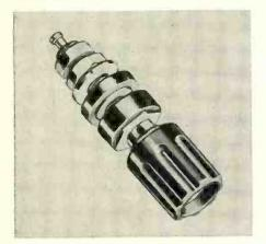
stand 50 hr. minimum salt spray exposure. Insulation is molded thermosetting phenolic in accordance with MIL-P-14, type CFG. Will withstand approximately  $295^{\circ}$ F without distortion. The  $\frac{4}{32}$  in. crosshole of the stud is flush with the base to minimize crimping or cutting the inserted wire lead. Grayhill, 561 Hillgrove Ave., La Grange, III. TELE-TECH & ELECTRONIC IN-DUSTRIES. (Ask for 5-21)
