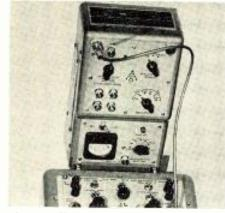
substantially below the noise level of vacuum tubes if suitable low noise operating parameters are selected. The new amplifier is expected to find application in biological research, hot-wire anemometer measurements, strain gauge measurements, etc. Input impedance 1,000 ohms, gain 1,000. Differential or adding input. Entirely battery operated, with 4 transistors, 6 vacuum tubes. Volkers & Schaffer Mfg., Corp., P.O. Box 996, Schenectady, N. Y. (Inquiry Card No. 6-20)
