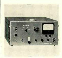
possible to measure large numbers of component parts visually or by meter reading without control readjustment. The instrument can be used as a Q meter by turning off the sweep. Frequency range is 20 to 220 MC. Q measure range, 0-125, 0-250. Resonating capacitor range, 7.5 to 100  $\mu\mu$ f, displayed on a digital counter for easy reading. Power supply, 105-125 v., 100 w. Kay Electric Co., 14 Maple Ave., Pinc Brook, N. J. (Inquiry Card No. 6-53)
