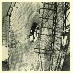
Photo above shows Felix Trombe's 40 ft. solar oven on Mt. Louis in the Pyrenees. It is one of the largest applications of solar energy and is used in production of refractory materials. 3000°C temperature is attained. Additional data is contained in "Research for Industry" published by Stanford Research Institute of Calif.
