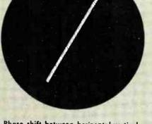
Phase shift between horizontal-vertical amplifiers, 0-100 kc-0°, to 1 mc within 2°; by internal adjustment with gain controls at max 0° phase shift possible on any specific frequency to 6 mc. 6 MC 4.5 MC Note flatness throughout specified
