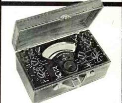
Universal 88". 88 range AC and DC Polyranger • 5.2" scale length • accuracy .5 of 1% on DC and .75 of 1% on AC.
