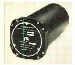
namic functions. The potentiometer wiper moves linearly with pressure over the range 3.42 to 30.36 in. of mercury. Accuracy,  $\pm 1\%$  of full scale voltage ratio. Trans-Sonics, Inc., Bedford Airport, Bedford, Mass. (Inquiry Card No. 6-38)
