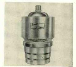
30 mc. The new tetrode delivers 10 kw. output in Class AB1 service and handles high inputs without going into the positive grid region. The simple coaxial structure allows low lead inductance, and a finned anode improves cooling with low air pressure. Offers greater electron tube reliability and increased immunity to thermal and physical shock damage. Eitel-McCullough, Inc., Technical Service Department, San Bruno, Calif., TELE-TECH & ELECTRONIC INDUSTRIES. (Ask for 6-9)
