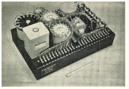
Fig. 1: Reference unit and preamplifier, using magamps, is part of a new high-speed regulating system for the excitation of large power generators
