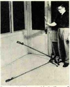
The same microphone used in the "hammer" test was mounted on a standard microphone floor stand. The stand was tipped until it fell over and the "333" crashed onto the bare floor. This was done six times—and there still was no noticeable change in the performance of the "333"!
