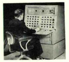
variables: mach number, pressure ratio, speed of sound ratio, engine thrust, airplane grossweight, reference area, and profile and induced drag coefficients. Under assumed steady state conditions, the computer exactly solves the two longitudinal equations of motion, simultaneously. Accuracy is generally consistent with input to 0.1%. Link Aviation, Inc., Binghamton, N. Y. (Inquiry Card No. 6-43)
