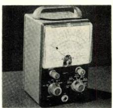
seven ac. (RMS) and dc. voltage ranges of 1.5, 5, 15, 50, 500, and 1,500; seven peak-to-peak ac voltage ranges of 4, 14, 40, 140, 400, 1,400, and 4,000; and ohm-meter ranges of X1, X10, X100, X1,000, X10k, X100k, and X1 meg-ohm. A db scale is provided and a zero-center operation is within the range of front panel controls. Employs 4½ in. meter-1% precision resistors –ac. power supply. Heath Co., 305 Territorial Rd., Benton Harbor, Mich. (Inquiry card No. 6-22)
