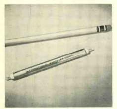
tive load. At 71°C ambient temperature --typical airborne ambient—the unit delivers 1.2 ma. dc current at 1,360 v. dc from 2,130 v. RMS ac. input. Lightweight tin-plated brass construction. Measures 5½ in. overall with a  $\frac{5}{16}$  in. O.D. Also available is a complete range of selenium rectifiers with input voltages from 33 v. to 660 v. International Rectifier Corp., 1521 E. Grand Ave., El Segundo, Calif., TELE-TECH & ELEC-TRONIC INDUSTRIES. (Ask for 5-65)
