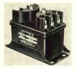
The units meet or exceed the requirements of MIL-F-7414 (USAF). Including terminals and mounting plates, dimensions are  $4 \times 2\frac{1}{8} \times 3\frac{1}{4}$  in. Weight, 1.0 lb. The flasher is hermetically sealed and requires no maintenance. The interrupter circuit, operates on 24 to 30 v. dc. separately from the lamp circuits, which can use any voltage from 5 to 115 (ac or dc) at 30 amps. Electronic Specialty Co., 3456 Glendale Blvd., Los Angeles 39, Calif. (Inquiry Card No. 6-37)
