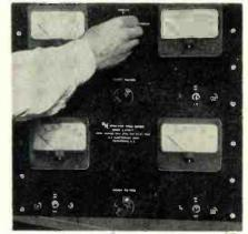
operation: series aiding, 400 to 1,000 v., 0-300 ma, grounded either polarity or anywhere between the two ends; parallel, 200-500 v., 0-600 ma, grounded either polarity with accurate load division up to full rating. Series bucking, 0-300 v. at 0-300 ma, grounded either polarity. Isolated, two identical, independent 200-500 v. supplies that can be operated in any polarity up to 1,500 v. apart. New Jersey Electronics Corp., 345 Carnegie Ave., Kenilworth, N.J. (Inquiry Card No. 6-77)
