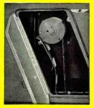
Telop III... interior view of automotic slide holder which accommodates 4" x 5" opaque slides...One lens... no registration problem... no keystoning.
