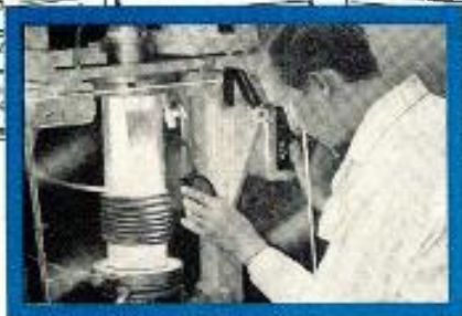
High-purity silicon crystals are drawn in PSI's high frequency induction furnaces.
