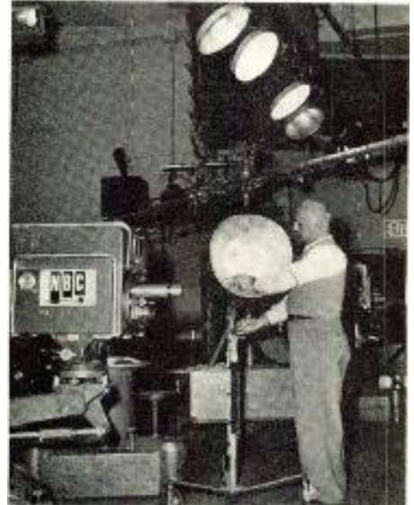
NBC's TV studio at Radio City, N. Y., now boasts a self-diffusing incandescent lamp that eliminates the need for a spun-glass diffusing "scrim" in producing a soft, white light. Developed by Westinghouse, the new 1000-watt lamp is shown being installed in a "scoop" fixture. Secret of the self-diffusing lamp bulb is an inner, baked-on coating of silica powder that absorbs a negligible amount of light. The fine white silica particles break up the beams reducing glare.
