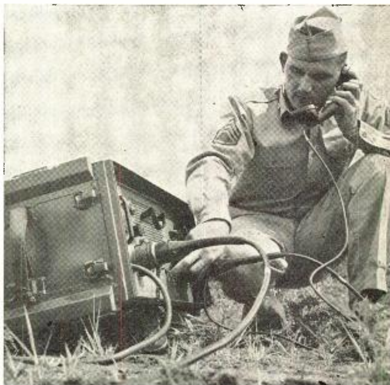
Portable, G. I. telephone system designed by Bell Telephone Labs. for the Army Signal Corps can handle four conversations at a time over a single cable. The repeater shown here is used to amplify the conversations, which may be transmitted over a distance of a hundred miles. It weighs only 178 lbs., a real improvement over the earlier version.
