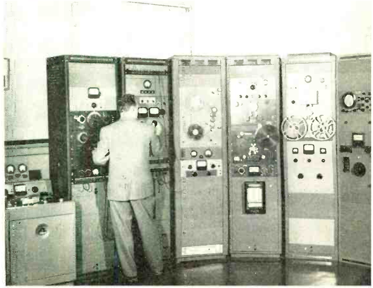
9 QUALITY CONTROL: All important manufacturing stages are closely monitored. Here custom-made quality control and test equipment at Audio Devices checks uniformity of "Audiotape"
