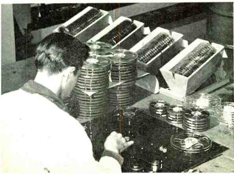
8 INSPECTION: "Encore" tape receives final physical inspection and cleaning prior to packaging. In some firms large magnets bulk erase any test signal remaining on sample reels
