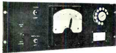
Fig. 4: Control panel for studio end of all-ac audio tone control system
