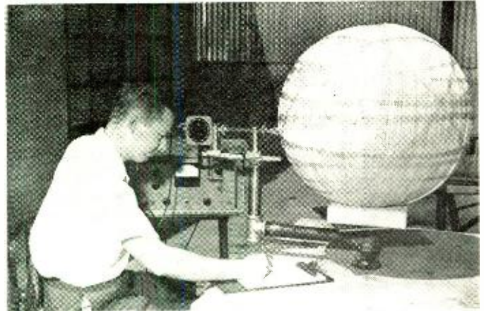
Fig. 2: Model of compressed styrofoam spherical-wedge lens
