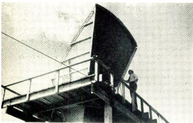
A new type of antenna resembling a giant sugar scoop has been designed by Bell Telephone Labs engineers to receive and transmit telephone and television signals. The horn-reflector antennas, to be used on Bell System radio relay routes, may eventually handle up to about 20,000 telephone circuits or 30 television programs at one time. They would handle simultaneously microwave radio systems in the 4,000, 6,000 and 11,000 MC bands.
