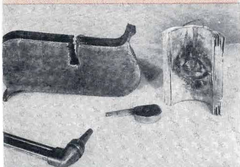
Class H insulation resists fire and combustion. The heat of the 5000° F. Oxygen-Acetylene torch, applied for the same interval, burned through the 2-inch steel plate, yet merely melted some of the glass fabric in the barrier.
