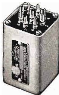
HIGH-FIDELITY INPUT TRANSFORMER, WF-20, for low impedance microphone, pickup or line to grid. Primary impedance 50, 125/150, 200, 250, 333, 500/600 ohms. Secondary impedance 50,000 ohms. Frequency response 30-20,000 cps. \pm 2 db. Negligible harmonic and intermodulation distortion. Grey enamel cast case with phenolic terminal board and tapped holes for flush mounting. 2" high by 1 \frac{1}{2} " square.
