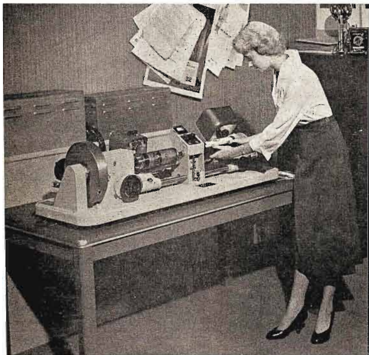
This Fairchild electronic engraver will make a four-column 85-line plastic halftone in 24 minutes, from a photograph of the same size. Already over 800 of these engraving machines have been installed in newspaper offices, making it possible for editors to produce engravings promptly and without sending the work out to the slow, old-fashioned acid-etching processes with many hand operations.
