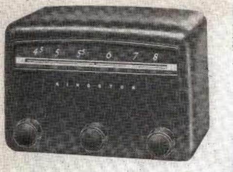
Fig. 1: Tuning, power and antenna changeover knobs protrude from front of the completed unit
