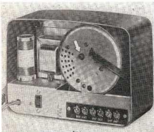
Fig. 2: Rear view shows panel board terminals for UHF antenna, VHF antenna and VHF receiver
