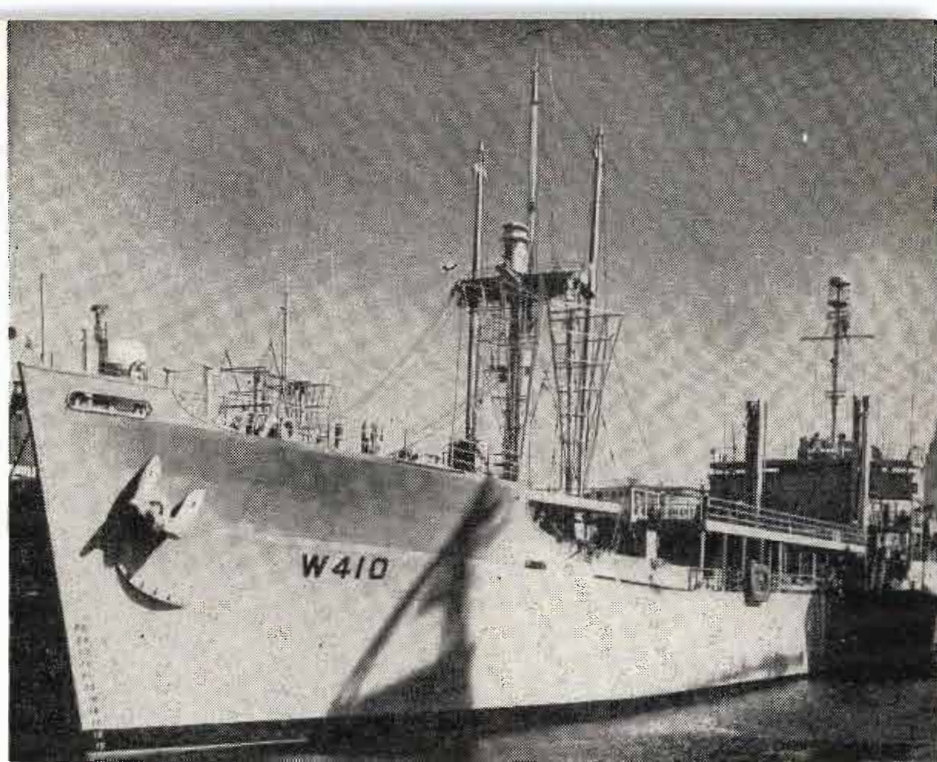
The Coast Guard cutter, COURIER , awaits orders for the tour of duty which will send it around the world, pouring radio information into Soviet controlled lands from off-shore. The raised platform seen amidships is a flight deck from which 69 x 33 ft. barrage balloons are released and sent 1,000 ft. into the air, carrying aloft the half-wave antenna for the 150 kw transmitter. Other features include eight whip antennas for dual diversity reception, and cork and reinforced concrete transmitter mountings.
