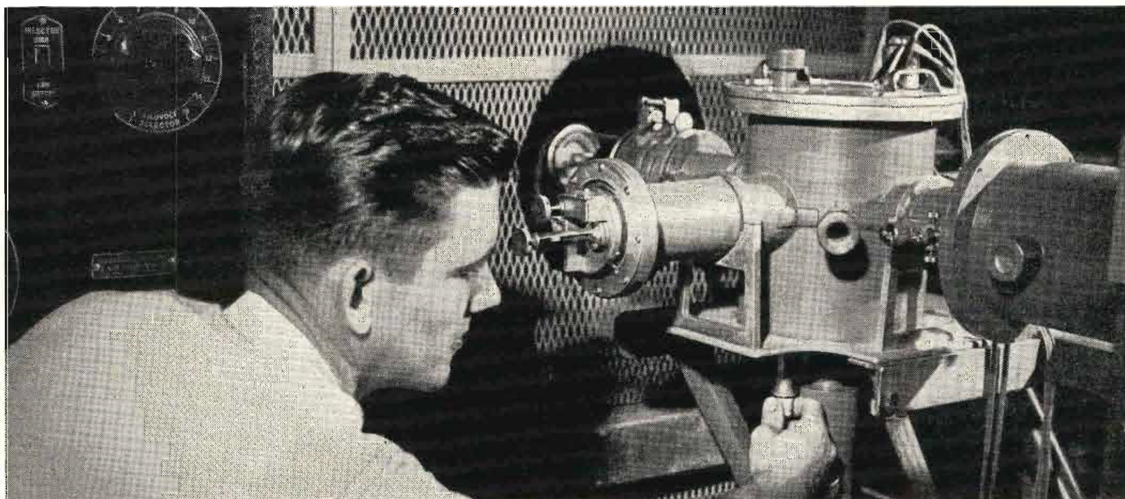
3 A Bell scientist adjusts electron diffraction camera. Electrons are projected on the specimen at glancing angles. They rebound in patterns which tell the arrangement of the atoms . . . help show how telephone materials can be improved.
