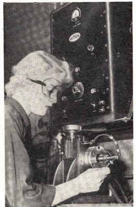
Photo of equipment arrangement using ultrasonics to salvage critical metals used in the manufacture of vacuum tubes.
