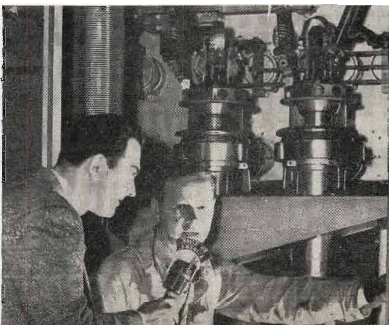
Jean Seymour describes the RCA 150 kw standard broadcast transmitter to Voice of America reporter Bob Jones. The four 9C21 tubes, connected in parallel in the final stage, are cooled with distilled water which passes through a salt water heat exchanger. Power is supplied from three 500 kw, three-phase, 440 CPS generators which are driven by individual diesels. Transmitter output may be fed to a balloon-supported half-wave antenna, or to a balloon-and-buoy rhombic, or to an emergency three-wire flat top.
