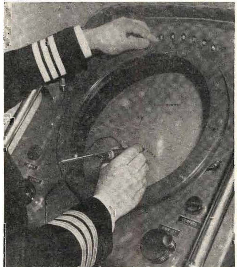
New "reflection plotter," developed by Raytheon for use in conjunction with shipboard radar, enables mariners to accurately interpret all movements of nearby vessels. By marking successive locations of ships on the plotter, as seen on the PPI below, it becomes possible to determine the course of all ships within range of the radar, and to determine how far away and when these vessels will pass. Any lines that project across center of PPI represent collision courses. By knowing elapsed time between successive position dots, what operating range radar is set for, the amount of time remaining to avert disaster can quickly be determined.
