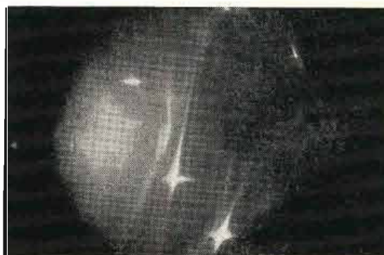
4 Diffraction pattern of polished germanium reveals minute impurities which would degrade the performance of a Transistor.
