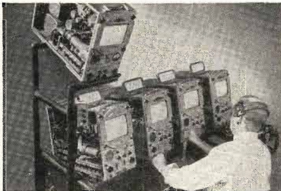
Compact GPL Cameras feature smooth operation, simplified control, (Swing-up and removable chassis permit easy servicing).
