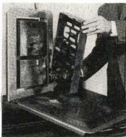
Stencil and stencil holder assembly used in fast spraying of component identification
