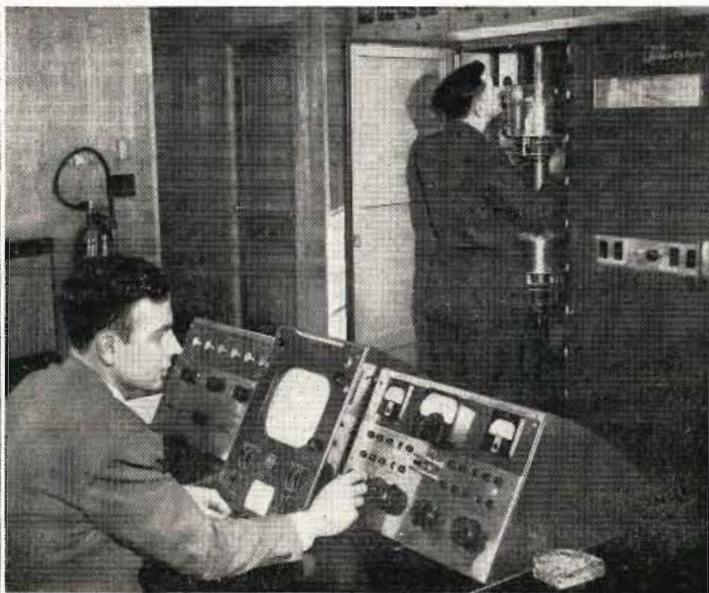
Station wagon (left) used for measuring field intensities of experimental UHF television station KC2XAK, Stratford, Conn. "Bow Tie" receiving antenna is mounted on roof of vehicle. Engineers (right) check control console and transmitter switchboard of the RCA-NBC station
