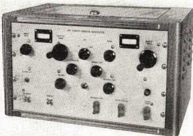
Fig. 9: Front panel view of developmental model UHF sweep generator. The instrument should prove a useful tool for obtaining rapid quantitative analyses of tuners, filters and associated units employed in UHF television equipment
