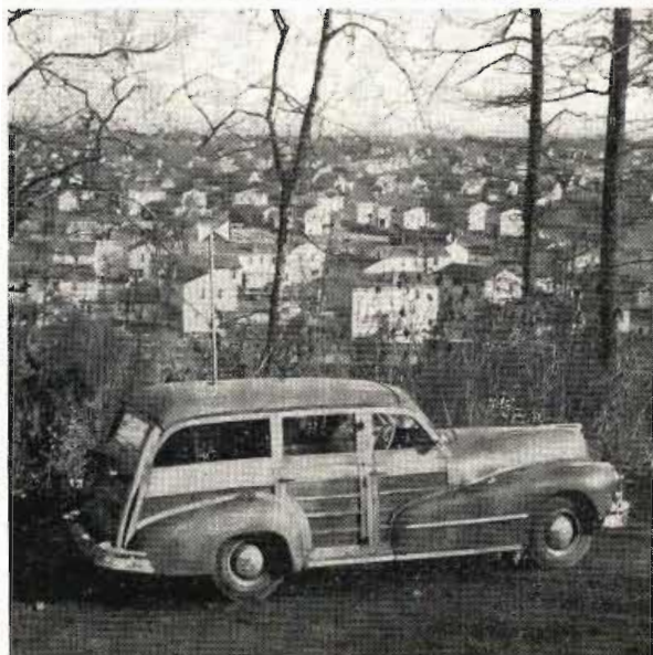
Station wagon (left) used for measuring field intensities of experimental UHF television station KC2XAK, Stratford, Conn. "Bow Tie" receiving antenna is mounted on roof of vehicle. Engineers (right) check control console and transmitter switchboard of the RCA-NBC station
