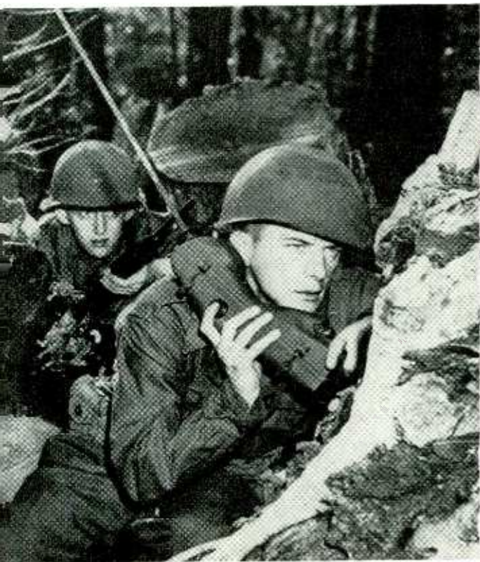
This new handie-talkie for Infantry, weighing 6½ lbs., has been redesigned to operate as an FM transceiver. It has a range of approximately one mile and will "net" with a greater number of other sets including the walkie-talkie. The latter equipment (SCR-300 in WW-II) has also been redesigned to about half its previous weight and bulk. These improved equipments will weld Infantry Armor and Artillery into a more coordinated team.
