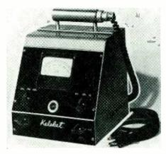
as model K-900. Geiger tube detecting element permits differentiation between beta and gam-ma radiation. The Geiger tube probe is con-nected to the main cabinet by a self-retract-ing cord. When not in use, the probe is mounted in the handle of the cabinet.—Kelly-Koett Manufacturing Co., 12-T East 6th St., Covington Ky.—TELE-TECH
