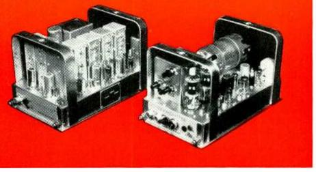
Fig. 1. Mobile transmitter (right) and receiver (left) for mobile narrow band FM
