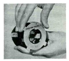
bly. It consists of a pair of rotating aluminum plates (one plate holds a permanent magnet) and is installed by snapping on the back cover of the television tube yoke. It will fit any standard yoke and is suitable for any size tube. The picture is centered by rotating the outer plate with the fingers. Fine adjust-ments are made by moving the outer plate up or down or to either side. Once set, the picture will not drift.—Perfection Electric Co., 829 South State St., Chicago 5, 111.—TELE-TECH TECH
