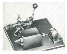
ing is removed, a new stripping machlne can perform this operation at 600 cuts per hour. It leaves a square cut and a clean shoulder absolutely free from frayed ends and does not damage the inner polyvinyl tube. Most wire strippers which use knives or brushes cannot perform this operation and meet in-spection requirements.—Wire Stripper Co., 1722 Eastham Ave., E. Cleveland, Ohio— TELE-TECH
