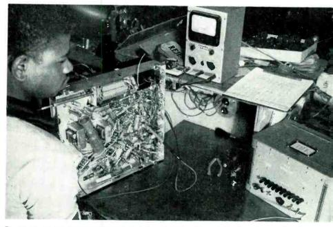
Fig. 3: View of i-f alignment station on main production line of Air King plant in Brooklyn, N. Y. Tel-Instrument type 1900 multi-frequency generator is used as signal source with an EICO VTVM being used as an alignment indicator. Generator, in furnishing 10 crystal controlled test signals, can be used to align stagger tuned i-f systems in TV receivers
