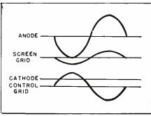
Fig. 4: Electrode potentials for r-f cycle
