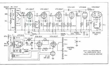
Fig. 3: Circuit diagram of the logarithmic amplifier which has a gain of 100 db
