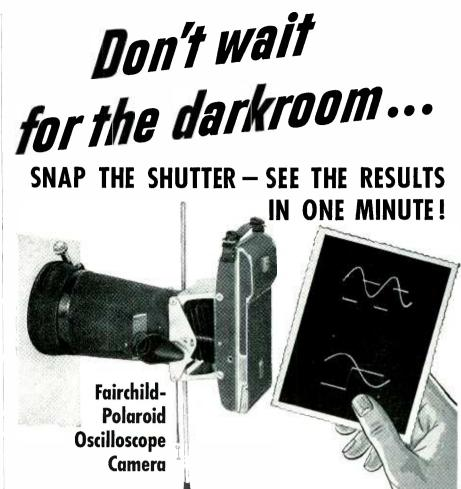
There's no longer any need to wait for carkroom processing before evaluating newly exposed photographic "stills" of oscilloscope images. This 3¼ x 4¼ print of a multi-beam scope image was ready for evaluation a minute after the shutter was snapped.
