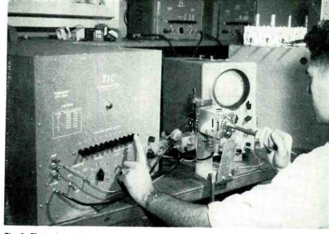
Fig. 2: Physical appearance of test diagrammed in Fig. 1. Tel-Instrument 1200-A r-f wobbulator is at left, tuner and test jig in center, and DuMont 274-A oscilloscope at right. Photo taken in advanced development laboratory of Air King Products Inc., Brooklyn, N. Y.
