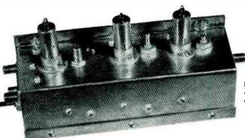
Fig. 1: Exterior view of unit whose overall dimensions are 1% x 1% x 5¼ inches
