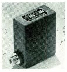
resistor, which forms the center conductor of a special self-terminated coaxial structure. Constant impedance properties depend upon shape of coaxial assembly and distribution of resistance along length of outer surface of resistor. Acting as an almost perfect termina-tion for 50-52 ohm coaxial lines, the VSWR of the model 80A is less than 1.05 from d-c to 400 MC and less than 1.2 to 2000 MC.-Bird Electronic Corp., 1800 East 38th St., Cleveland 14, Ohio-TELE-TECH
