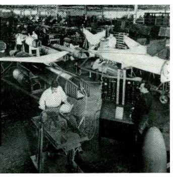
The Navy's new Martin KDM-1 pilotless target drones come off the sleepless Baltimore production lines. Powered by ram-jet engines, the target-drones are remote-controlled by radio and tracked by radar, to simulate the flight of an attacking airplane
