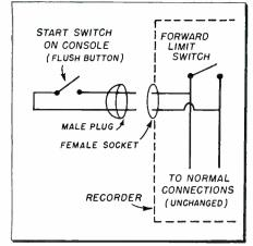
Wiring remote start switch for Brush recorder
