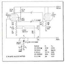
Fig. 2: Detailed diagram of oscillator
