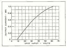
Fig. 1: 6SN7 output stage typical response
