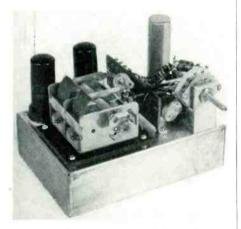
Fig. 1: New wide-range R-C oscillator
