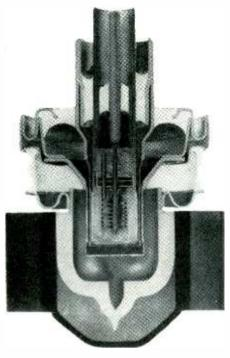
Fig. 1: Cross-sectional view of Eimac 4X150G
