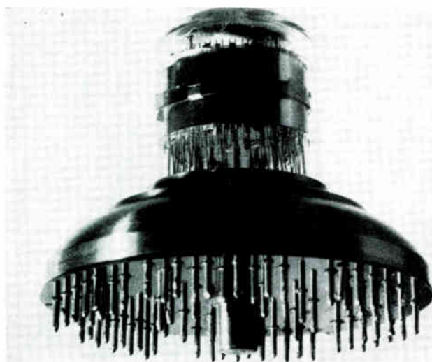
Fig. 4: (left) A forest of pins in the base of this tube is needed to connect with all of the elements of this radial beam tube. Fig. 5: (right) A rubber membrane provides an analogy with the
