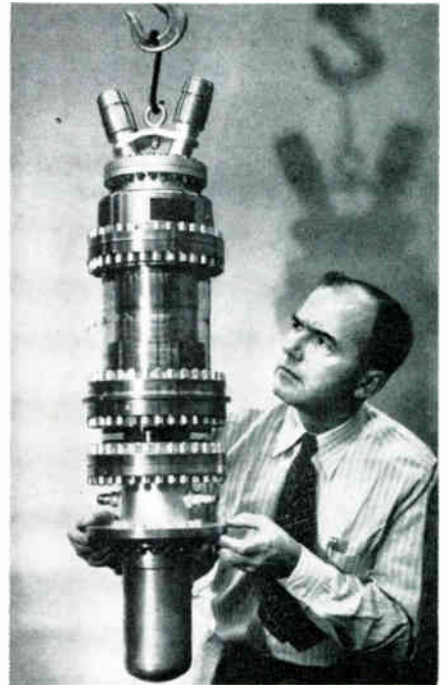
Dr. L. P. Garner, head of Advance Development Labs., RCA Lancaster, Pa., tube plant shown with the new "super-power beam triode" which is capable of 500 kw output, and which has been tested at one million watts input. Compact design weighs only 135 lbs. and measures 38 3/4 in. in length. Present applications are for CW high power operation and for international broadcasting
