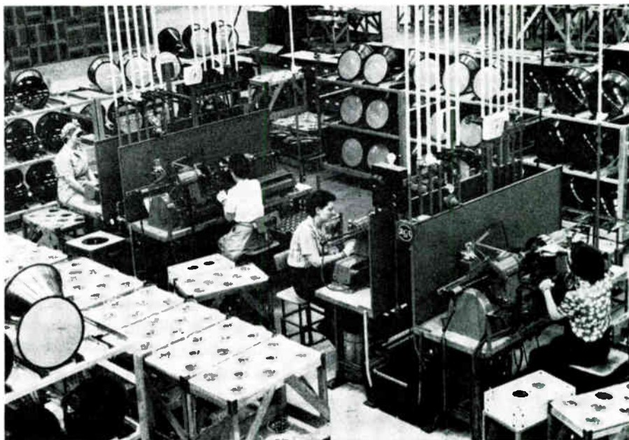
Interior view of RCA's new tube plant in Marion, Indiana, showing women operators at glass lathes where neck section of 16-in. metal TV tubes are fused to the cones. The plant, which at present is largely devoted to the manufacture of short-necked 16-in. tubes, is expected to become one of the world's largest TV tube producers
