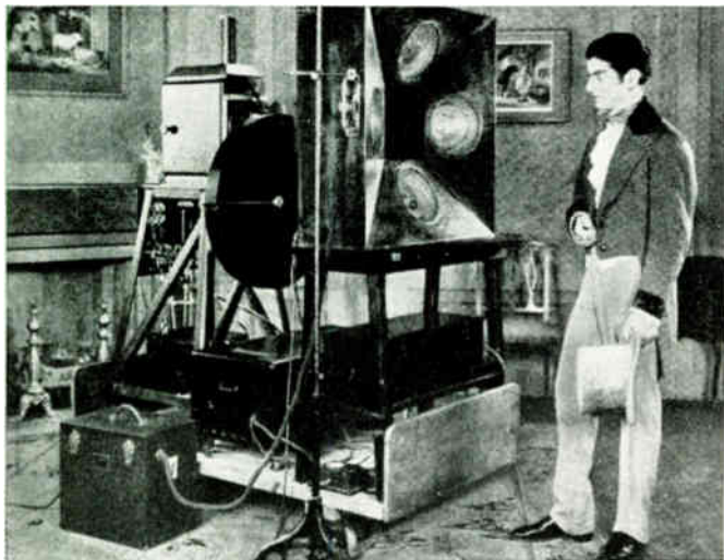
Mechanical scanning equipment, used at RCA-NBC experimental television station W2XBS in 1928, long before the present RCA image orthicon camera came into existence.
