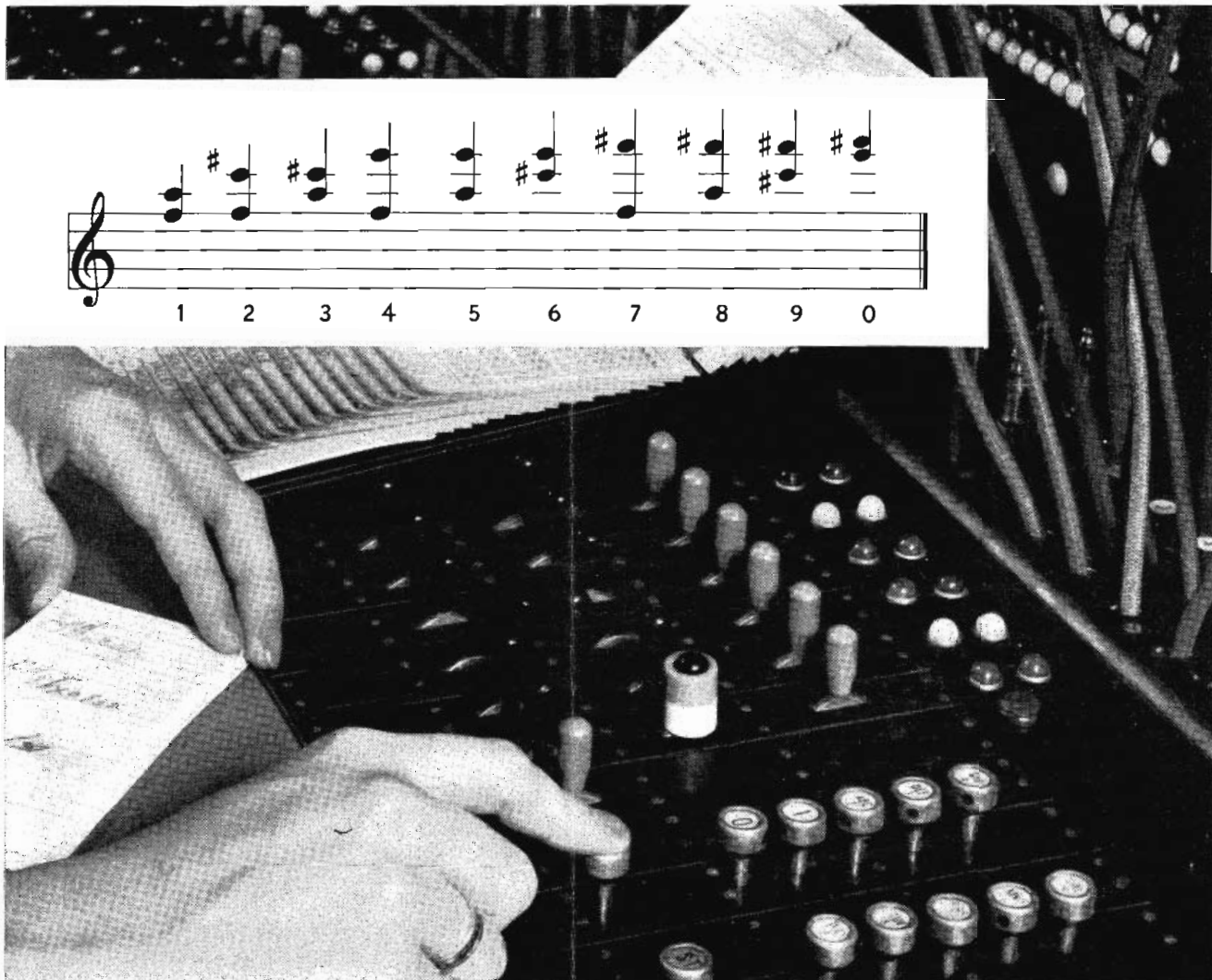
Above is the Bell System's new "musical keyboard." Insert shows the digits of telephone numbers in musical notation, just as they are sent across country.
