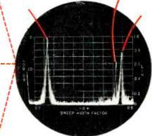
Interference analysis with Model SA-8b Panadaptor. Sidebands from AM channel #3 is seen to spill into band occupied by intermittent CW channel #2.
