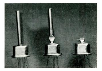
Fig. 9: Commercially produced units are encased in a standard transistor casing.
