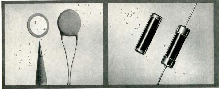
• A Du Pont silver coating has been fired onto the barium titanate ceramic capacitor disc shown above. This disc is then solder-dipped to attach wire leads.
