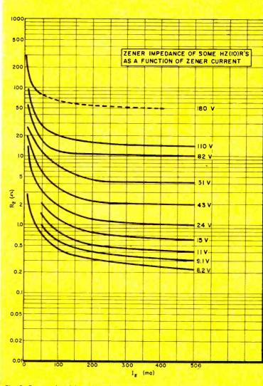
Fig. 9: Reverse breakdown impedance as a function of reverse current.
