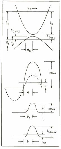
Fig. 1: Class C tube operation. The dotted curve in second group represents the fundamental frequency.
