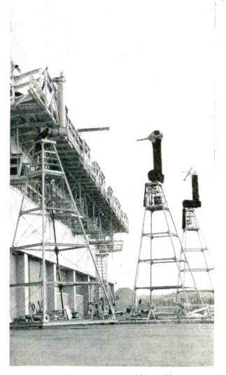
ANTENNA PATTERN RANGE, with movable towers capable of handling models up to 1000 pounds. Boeing has openings in ECM antenna development, and in gas, solid and liquid dielectric research, as well as large-aperture antennas for ASMs, orbital vehicles and airborne warning systems. Other openings are available in instrumentation, missile guidance and control.
