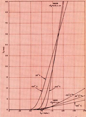
Fig. 4: Forward voltage drop as a function of forward current for diodes of varying base layer resistivity with temperature as a parameter.
