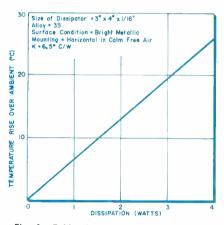
Fig. 1: Calibration curve for dissipator
