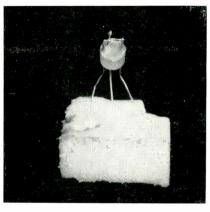
Fig. 8: Small diameter wire makes spring contact on the plating in the groove.
