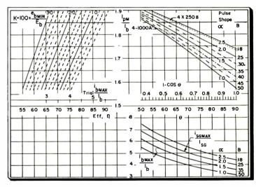
Fig. 2 (above): Charts used for the design of an amplifier.
