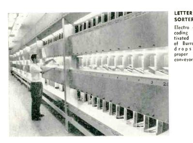
SORTER Electro - mechanical coding system activated by operator of Burroughs sorter d r o p s letters into proper bins f r o m conveyor.
