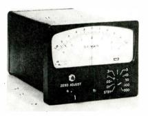
amplifier. A dc loop, including the chopper itself, is established by returning the metered demodulated signal via the chopper to the input of the instrument. Metronix, Inc., Chesterland, Ohio.
