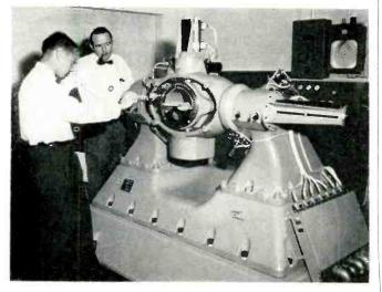
Convair engineers examine features of a new Bendix flight simulator table which has successfully tested B-58 equipment.
