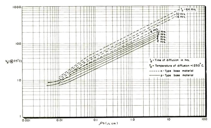
Fig. 7: Breakdown junction of diffused junction diodes measured at a reverse current of 10 ma., as a function of base layer resistivity for n- and p-type base regions with diffusion time as a parameter.
