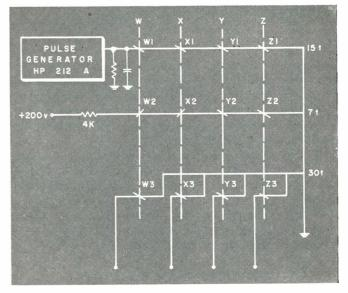
Fig. 2: Drawing shows magnetic drivers for diode matrix input
