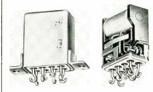
R-575C and MIL-R-25018. Standard operating coils are 26.5 vdc nominal —coil resistance, 400 ohms. Weight is 3 oz. Size is  $\frac{5}{8} \times 1-1/32 \times 1\frac{1}{4}$  in. Hook type and long and short wire lead terminals available. Headers have 0.2 in. grid spacing. Struthers-Dunn, Inc., Pitman, N. J.
