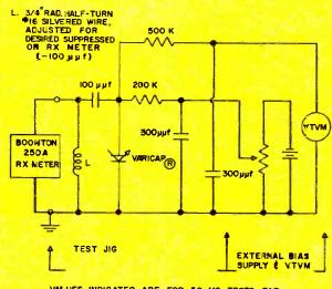
VALUES INDICATED ARE FOR 50 MC TESTS FOR CAPACITANCES UP TO 170 µ µ f
