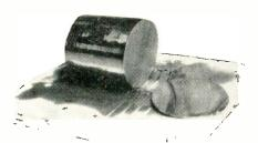
Fig. 1: Germanium crystal is shellacmounted on tile for easy diamond saw slicing. One of the slices is on the right. Two methods of manufacture are presented: the laboratory procedure detailed fully; the industrial process outlined briefly. The former, successfully developed by the author, provides units suitable for investigative experiments.
