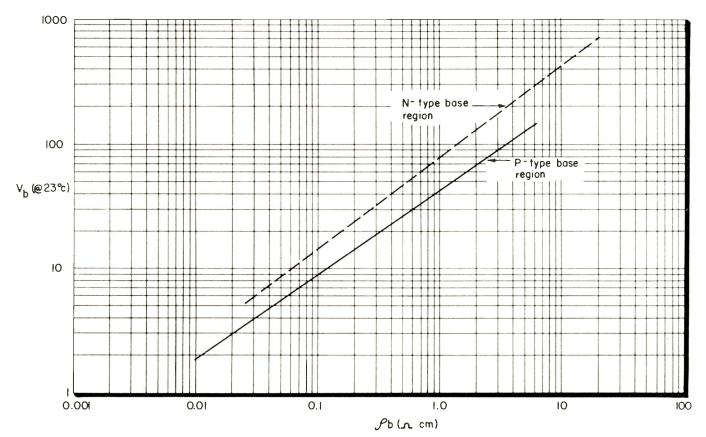
Fig. 5: Reverse breakdown voltage of alloy junctions as a function of base layer resistivity for n- and p-type base regions.
