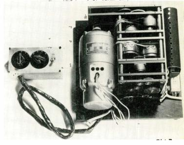
speed transmission are for recording instruments such as oscillographs and other recording devices requiring constant and precise speeds. It can also be used as a laboratory device for testing servo packages along with many other uses.
