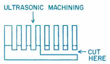
Fig. 11: Ultrasonic tool cuts 30 small bars from the crystal in just one pass.
