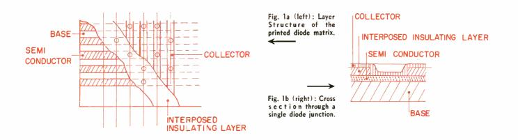
Compact matrices of low cost and high reliability are one of the most powerful building elements in data handling systems. To accomplish this, printed circuit techniques are contemplated for manufacturing these compact diode or resistor networks. Progress and state of the art are given here.
