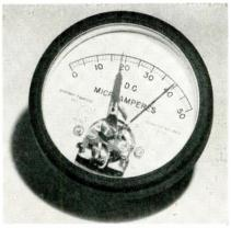
Indicating pointer has passed set point but control circuits remain energized. Note position of toggle, on adjustable pointer.
