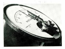
separate coil increases control dependability by boosting contact torque at set point and thus insuring positive actuation of a load relay.
