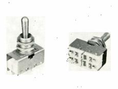
position off. Detent action gives positive "feel." Each pole of the switch element is rated at 6 amps, 125/250 vac, 30 vdc, resistive and 3 amps, 30 vdc, inductive. Weight is approximately 1 oz. Exposed parts are stainless steel or corrosion resistant. Electrosnap Corporation, 4218 W. Lake Street, Chicago 24, Illinois.
