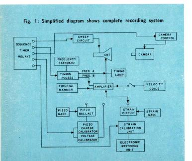
Piezoelectric gages incorporate, as an active element, material such as quartz, tourmaline or barium titanate and measure fluid pressure such as that produced in a chamber by an explosive or the air blast in the path of a detonation wave. Resistance type gages can measure quantities, such as strain and temperature, which are capable of varying resistivity of these transducers.
