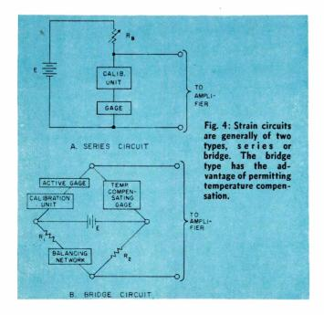
directly to various types of transducers to measure other parameters. For example, fluid pressure can be measured by the change in resistance of a coil of wire attached to the outside surface of a tube which is expanded by the pressure.
