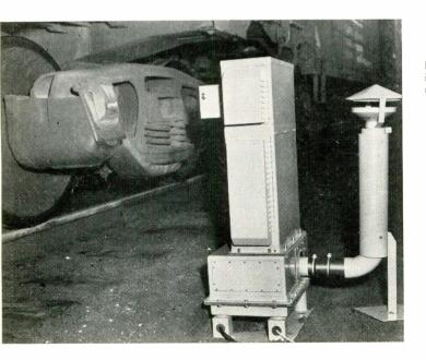
Foolproof detection is provided through unique temperature sensing and comparison mechanisms; thermocouple is used in place of a bolometer.
