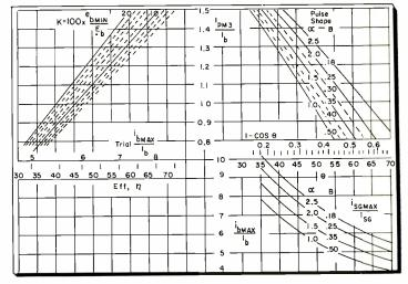
Fig. 4: Frequency tripler design is eased with this chart.
