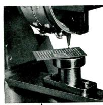
Part of the secret's in Segal's unique anvil tool holder and spring loaded work table (shown at left) which allow the eyelet to pass through the assembly before staking or flaring. Avoids loose settings, compensates for material variations, too.
