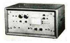
load. Designed for scintillation spectrometry and proportional counting. Several optional accessories are available. The Victoreen Instrument Co., 5806 Hough Ave., Cleveland 3, Ohio.
