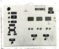
Fully automatic readout feature makes possible positive detection without the need for operator judgment. Audible alarm eliminates need for constant surveillance.
