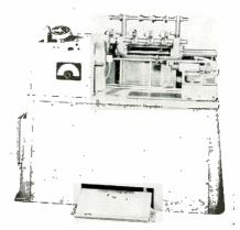
similar types of coils. Dial is calibrated in wire sizes from 10 to 31 A.W.G., for selection of correct winding pitch. Machine also handles wire finer than 31. Max. coil OD is 16 in. Max. winding stroke 9 in. Max. loading distance for multiple winding 24 in. Geo. Stevens Mfg. Co., Inc., Pulaski Rd. at Peterson, Chicago 46, Ill.
