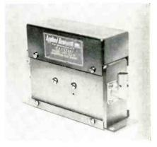
They are aligned to obey the Butterworth condition, and have a low insertion loss. Typical unit operates at 332 MC with 3 db bandwidth of 24 MC. With this center frequency, weight of the filter is 20 ounces. Dimensions are  $5\frac{1}{8}$  in. x 1 11/16 in. x 3¼ in. Applied Research Inc., 76 South Bayles Ave., Port Washington, N. Y.
