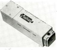
connector block for wiring to telephone lines. A balanced filter, it can be employed for any audio purpose. Filter is rated at 0.5 a.; 30 v.; 0 to 60 CFS. Resistance: 12 ohms, size:  $8\frac{3}{4}$  in. long x  $2\frac{1}{2}$  in. square. Antran Div., International Electronics Mfg. Co., 2nd St. Extended, Greenwood Acres, Annapolis, Md.
