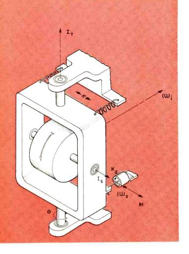
Fig. 1: Schematic representation of a rate gyro. Symbols are identified in Table 1.
