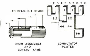
Fig. 3 (Left): Brushes read consumption in a 4-digit, binary code, from position on commutator.
