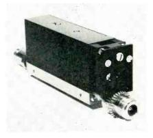
ing; in-line shaft adjustment; and direct reading, calibrated dial. Specs include: frequency band, available band widths from 4-7 to 7-11 KMC; attenuation variation with frequency less than  $\pm 5\%$  expressed in db; vSwR on all settings less than 1.5; power handling capacity, 4 w; designed to produce a max. 40 db attenuation. Merrimac Research and Development, Inc., 584 Washington Ave., Belleville, N. J.
