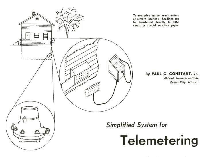
Remote reading of home meters would reduce costs and errors. The system could be extended to many shaft driven indicating devices.
