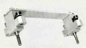
**HYDRAULIC STOP** A minimum size buffer used in a ballistic missile device to prevent inadvertent operation through handling shock. Provides tremendous damping force for its size.
