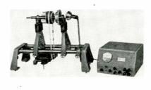
100 lbs., as well as a wide range of operating-balancing speeds. It is suitable for nearly every type of rotor up to a maximum diameter of 24 inches ... fans, armatures, blowers, pulleys, crankshafts, propellers, impellers, etc. Micro Balancing, Inc., Garden City Park, New York.
