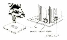
bottom edge of the i-f can, requiring no special cut-outs in the can or special assembly tools. Two barbs on the clip bite into the side of the can, providing firm retention and an excellent grounding connection between can and clip. A spring tab supplies tension until the final soldering operation. Tinnerman Products, Inc., Cleveland, Ohio.
