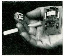
Miniaturized module makes it possible to pack five times more electronic gear in the nose cones of missiles.
