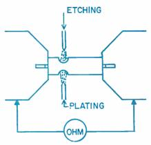
Fig. 12: This set-up continuously controls resistance of the bar during processing.
