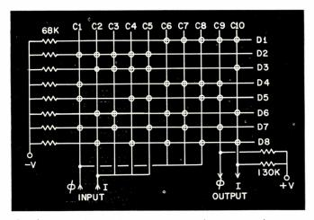
Fig. 6a: A decoder-encoder matrix pattern that was tested
