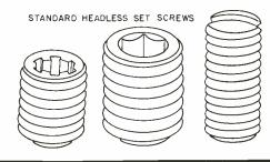
in pairs and located at an angle of  $90^{\circ}$  or 120° with at least one point bearing on a flattened portion of the shaft. Socket head screws, both hex and fluted, are available from size #0 to 2 in. diameter and are made of high strength steel with a class 3A thread per ASA **B18.3**, while the same screws with a slotted head are available in sizes from #5 to  $\frac{3}{4}$  in. with a case hardened surface and class 2A thread (ASA 18.6.2.).
