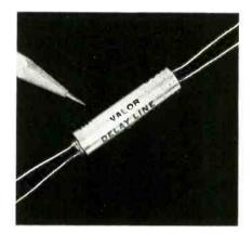
sistor applications. Specs: characteristic impedance 1400 ohms; attenuation 3%; temp. characteristic  $-0.03\%/^{\circ}$ C; temp. range  $-55^{\circ}$ C to  $+105^{\circ}$ C; build to MIL specs; molded in hermetically sealed brass tube with leads brought out through glassto-metal end seals; case finish—fused tin plate. Valor Instruments Inc., 13214 Crenshaw Blvd., Gardena, Calif.
