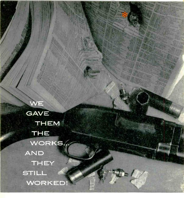
After being blasted out of a shotgun into a telephone directory, these International Rectifiers tested out to published specifications. Shock-resistant ruggedness like this is just one distinguishing feature of the reliability you can depend upon when you specify any International Rectifier.
