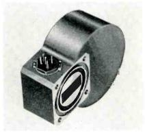
It may be used as a shutter or switch element. Featured are: Frequency Range 13.5 KMC  $\pm$ 15 MC; Isolation at 25 db min.; Insertion Loss is indicated at 0.3 db max.; Input vSWR Transmit is 1.10 max. at center frequency; Input vSWR Reject 30:1; Rise Time at 100  $\mu$ sec max.; Control Coil Power at 2 w max. Ambient temperature 85°C to 105°C. Kearfott Co., Inc., Microwave Div., 14844 Oxnard St., Van Nuys, Calif.
