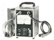
with an adjustable limit, visual leakage current-indicator. Models with the "Squawker" audible indicator are available with ac test potential output up to 6000 v. The visual and audible leakage indicators have an adjustment range from 300 µa to 3 ma as standard and to 10 ma on special order. Associated Research, Inc., 3777 W. Belmont Ave., Chicago 18, Ill.
