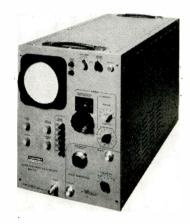
nal-to-noise ratio. Samples are taken from the successive, unamplified repetitive pulses under investigation, and their amplitudes are sampled for a very small time interval (400  $\mu\mu$ sec), amplified, stretched to about 1 msec. and displayed as a composite picture of the pulse shape on the CRT. Lumatron Electronics, Inc., Westbury, L. I., N. Y.
