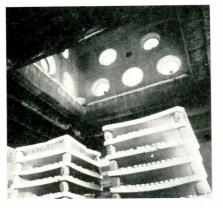
Fig. 3: A look into the heating chamber shows the pattern of the Duradiant burners in one wall. They have been lighted, stabilized, and are ready to fire the workload.
