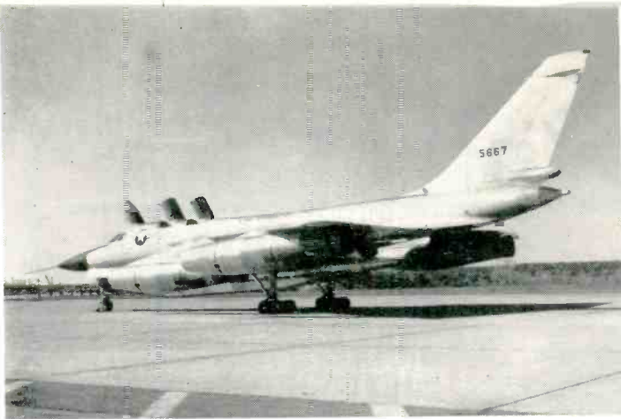
Fig. 1: Equipment will check the active defense system of the B-58. Note the location of the system at the tail above the Vulcan gun which fires 6000 round/min. Details are shown in Fig. 8.
