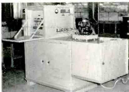
Fig. 3 (above): A & E Shop equipment tests the system's line replaceable units (LRU) like the tactical stable platform.
