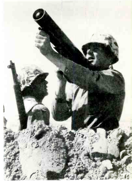
FOXHOLE MISSILE New "Red Eye" guided missile is designed for use against low strafing and bombing aircraft. Convair developed the 20-lb. 4-ft. long missile for the Army and Marine Corps.
