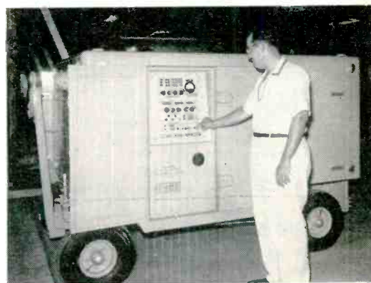
Fig. 7: Tactical System Test Set (TSTS) isolates a malfunction to a defective LRU which can be replaced on the flight line.
