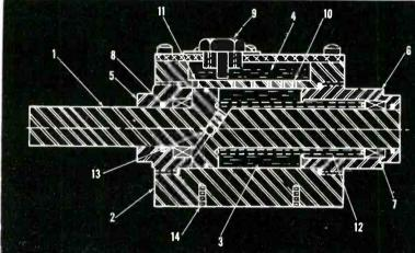
TYPICAL HOUDAILLE BUFFER 1 Ram 2 Housing 3 Cylinder 4 Reservoir 5 4 6 Closure flanges 7 Bearings 8 Seals 9 Fluid-level indicator and filler opening 10 Orifices 11 Return Port 12 Return Spring 13 Check Valve 14 Tapped Holes
