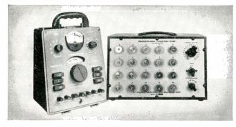
A full line of strain instruments—for static and dynamic strain measurements—is available through your B-L-H Sales-Engineering Representative. Instruments include (left) the B-L-H Type N Strain Indicator, calibrated to read directly in microinches per inch; (right) B-L-H switching and balancing unit, designed to facilitate bridge balancing and gage readout on multiple gage installations.
