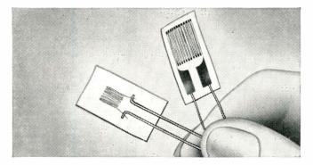
Why risk unreliable data by using *almost* the right strain gage. Select the one exactly suited to your application from the more than 250 different bonded wire and etched foil SR-4<sup>®</sup> Strain Gages listed in the current B-L-H catalog. High temperature, temperature-compensated, rosette and many other types are stocked by your B-L-H Sales-Engineering Representative for Immediate delivery.
