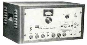
**Specifications:** In two ranges -0.5 MC to 400 MC and 275 MC to 1200 MC-with center at any frequency from 500 KC to 1000 MC and with sweep widths as broad as 400 MC and as narrow as 100 KC. The RF output-is flat within  $\pm 0.5$  db at full sweep width up to 800 MCS and  $\pm 1.5$  db from 800 MCS to 1200 MCS. When using sweep widths as narrow as 20 MCS flatness is approximately  $\pm 0.15$  db.
