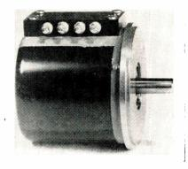
All joints and screw holes are sealed with a rubber potting compound on this humidity resistant Potentiometer. Teflon shield creates moisture barrier for shaft.
