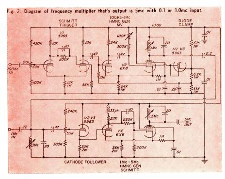
harmonic and nulls occur close to the ninth and eleventh harmonics. In the time domain again, this waveform results in two decay regions of the tank voltage, one of 4.5 and one of 5.5-cycle duration. This results in a smaller decrement than would occur if the tank circuit voltage were allowed to decay for the entire 10-cycle interval.
