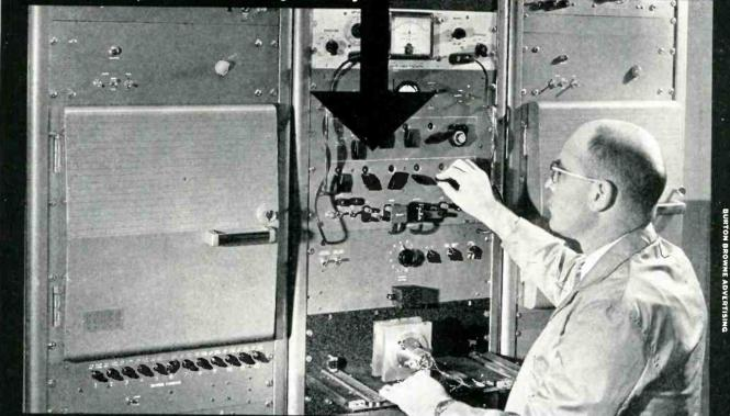
This Test Stand handles 12 units simultaneously, all temperature compensated to -55°C to +150°C. Also tests output voltage, phase shift and linearity. Test Stand has a speed accuracy of .01%, transformation accuracy of .001% and onese shift accuracy of 2 minutes.
