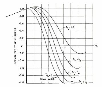
Fig. 3: Retrace yoke current applied to TV horizontal deflection.
