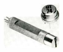
can be mounted so that the gaps of two adjacent heads are only 0.150 apart circumferentially, making the head ideal for close recirculating registers. The heads are low inductance for efficient transistor driving. Mechanically the diameter of the head is only 0.216 with an overall length of 1.062. The head is available with shielded and jacketed cable. Magne-Head Div., General Transistor Western Corp., 2660-64 So. La Cienega Blvd., Los Angeles 34, Calif.
