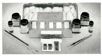
The proper application of a strain gage to a surface is fundamental in obtaining accurate strain data. B-L-H cements, solvents, waterproofing and lead materials and accessory equipment help you do the job right. Convenient strain gage application kits contain everything you need, including detailed instructions. Kit materials can also be supplied in bulk form in large or small quantities to suit your needs.
