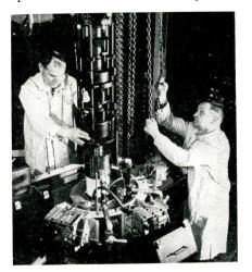
GE technicians install multi-million watt klystron in the FPS-7 super power radar
