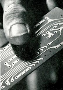
FOTOCERAM,<sup>®</sup> an unusual new printed circuit board We've resoldered more than fifty times on this board without damage to circuit runs or through-plate holes. No adhesives needed to bond copper to board. Bond strength between Fotoceram and metal is 15 to 20 lbs., when 1" strip is pulled perpendicular to board. Takes over 60 g vibration shock. All electrical properties equally outstanding.
