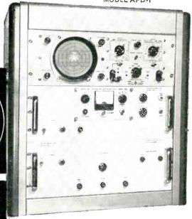
In one unit, either polar or rectangular coordinates; either log, linear or square root response
