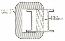
Fig. 2: Split bobbin fitted on the core.
