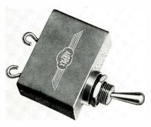
of ambient or operating temp. Units available for interrupting 50dc volts at currents from 0.05 to 10 amperes and for interrupting 120 RMS volts, 60 to 400 CPS at currents from 1.0 to 10 amperes. The toggle handle of the breaker is similar to conventional onoff switches. Booth 521, Airpax Electronics Inc., Cambridge Division, Cambridge, Maryland.
