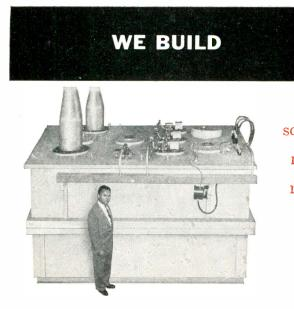
120 KV 2 A DC power supply installed at Eitel-McCullough, Inc. for klystron testing
