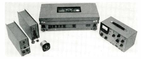
The complete recorder system includes, from left to right, a power converter, electronics box, the remote control unit, the AR-200 tape transport, and a test unit.
