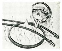
tude insensitive and moisture resistant. The cable core is modified semi-solid silica; inner and outer conductors are coated oxygen-free high conductivity copper wire. Nominal impedance is 50 ohms. Velocity of propagation is 69.0%. Maximum operating voltage is 1000 vrms. Amphenol Cable & Wire Div., Amphenol-Borg Electronics Corp., S. Harlem Ave. at 63rd St., Chicago 38, Ill.
