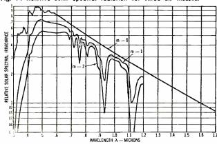
Fig. 8: Relative spectral response of short circuit current for solar radiation (uncoated cell), at three air masses
