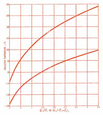
Fig. 9: Surface temperature of solar collectors in space
