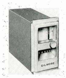
readout. It indicates and records forces, fluid flow, weights, or rpm's which can be converted into ac or dc mv. and eliminates errors due to parallax and interpolation of readings. It has a permanent recording chart. Dimensions: 6 x 111/8 x 12 in. Digital readout accuracy: 1/10 of 1%; chart accuracy is  $\pm 1\%$ . Gilmore Industries, Inc., 13015 Woodland Ave., Cleveland 20, Ohio.
