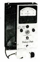
Fixed tuning range: 0.5-500 MC; variable: 0.5-1000 MC. Min bandwidth for max vswr of 1.4 = 200 mc from 500 to 1000 MC. From 200 to 500 MC bandwidth increases. Below 200 MC the unit is broadband down to 0.5 MC. Booth 3114. Kay Electric Co., Maple Ave., Pine Brook, N. J. Circle 242 on Inquiry Card
