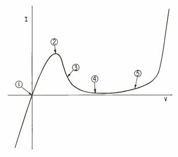
Fig. 6: Various bias conditions of the tunnel diode. The numbered points on the curve correspond to the diagram below.
