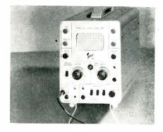
125 v or 220 to 250 v, 50 to 800 cPs. Vertical passband is dc to 5 mc, risetime is 0.07  $\mu$ sec, deflection factor is 10 mv/div. Sweep range is 0.5  $\mu$ sec/div to 0.5 sec/div in 19 calibrated steps. Accelerating potential is 4 kv on a 3 in. C-R tube. Amplitude calibrator is a 500 mv peak-to-peak 2 KC sq. wave. Booth 1801. Tektronix, Inc., P. O. Box 831, Portland 7, Ore.
