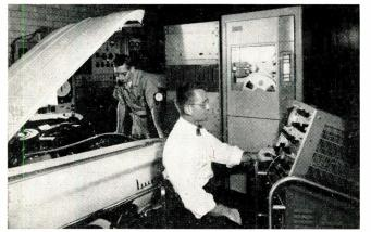
NGINEERS from Du Pont's E Petroleum Laboratory have developed a simple to use instrument for measuring the presence and extent of surface ignition which sometimes produces a rumbling noise and loss of power in modern automobile engines.
