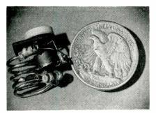
Complete transmitter using tunnel diode
