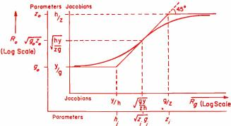
Fig. 6 (left): Common emitter curve and asymptotes for output resistance vs. generator resistance.
