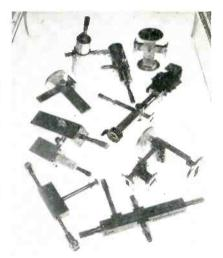
This family of parametric amplifiers includes the tiny units which can double the range of ground and aircraft radar.
