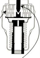
increasing to 23.5 kv at 40 mmfd and 30 kv at 10 mmfd. A switch is incorporated inside the vacuum to short out the total capacity under very high frequency operation. This also has the added advantage of having a common starting point, or a pre-set point, for the automatic tuning mechanism.
