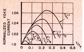
Fig. 4 (above): The initial portions of the retrace yoke current oscillations as shown in Fig. 3 are repeated here to a larger scale.
