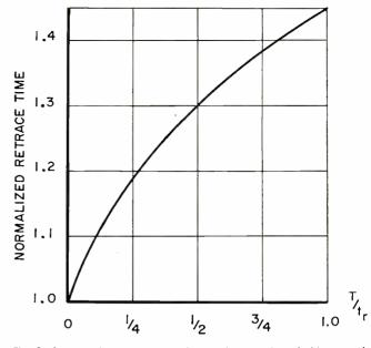
Fig. 9: Increase in retrace time due to decrease in switching speed.
