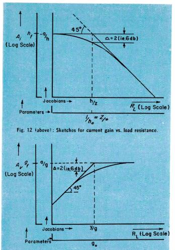
Fig. 13 (above): Relationship of voltage gain and load resistance.
