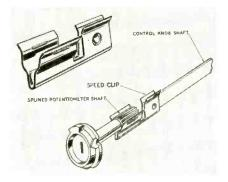
snapped into the U-shaped end of the speed clip where it is locked in position by a spring tab. The splined potentiometer shaft can then be inserted by pressing it between the semi-tubular spring legs, or by sliding it into the open end. Once the potentiometer has reached its turning limits, further turning of the knob results only in slippage of the clip. Tinnerman Products, Inc., Cleveland, Ohio.
