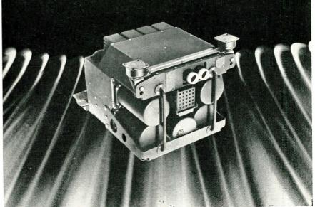
AiResearch Central Air Data Computer for North American's A3J, Navy's first weapon system, provides information dealing with bombing, navigation, engine inlet control, radar, automatic flight control and cockpit instrumentation.
