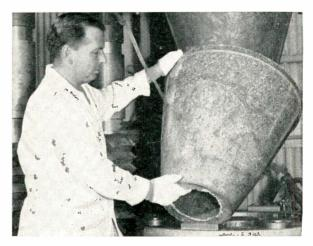
Exit cones capable of withstanding temperatures of  $6000^{\circ}$  F. represent one example of advanced engineering being performed by the Hughes Plastics Laboratory.
