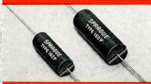
NEW!...DIFILM Type 162P slotted-base multi-purpose molded case capacitors for auto radios and other severe vibration applications. Slot prevents collection of moisture around leads when capacitor is end-mounted against chassis.
