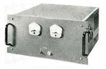
208-230 v. at any output voltage from 0 to max.; 1% load regulation from 0 to max. and max. to 0, recovery time 50  $\mu$ sec with no positive transient; 1% ripple; 60% eff. at max. voltage; 0.1% stability for 24 hrs.; operates indefinitely into a dead short; temp. coefficient 0.05%/°C. Booth 515. Kepco, Inc., 131-38 Sanford Ave., Flushing, N. Y.
