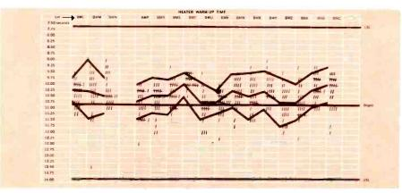
New variables inspection procedure gives a quantitative picture of the reliability of each important characteristic in Gold Brand Tubes
