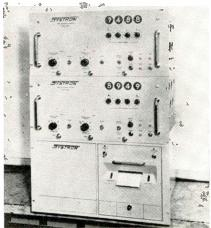
Model 1021-1 time interval meters take simultaneous measurements of elapsed time between the emitted signal and the return signal from two different ground stations. A Systron Model 1401-1 digital recorder provides a permanent printed record of both times and identifying code. Features include Nixie in-line readout, direct readout in nautical miles, and automatic subtraction of fixed delays. Systron Corp., 950 Galindo St., Concord, Calif.
