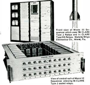
Automatic control of the countdown at the Air Force's Cape Canaveral Missile Test Center-from X minus 90 minutes to 10 minutes after a missile is firedis in the hands of a Milgo Model III Sequencer.
