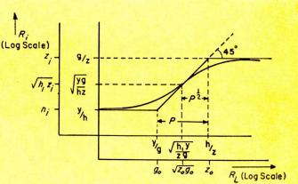
Fig. 1 (left): Common emitter relationships. The projection ratio, P, is numerically the ratio of the two coordinates.
