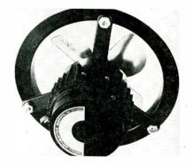
for running capacitors. A 4 in. axial fan (a typical unit) delivers 240 CFM at 0 in. S.P., 400 cycles. Ambient temperature range is  $-55^{\circ}$ C to  $+125^{\circ}$ C. These units have a typical application in airborne radar cooling and meet MIL-E-5400 and MIL-E-5272A. Booth 607. Air-Marine Motors, Inc., 369 Bayview Ave., Amityville, L. I., N. Y.
