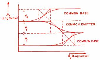
Fig. 9: Configuration of asymptotes for output resistance vs. generator resistance follows a similar pattern to that shown in Fig. 4.
