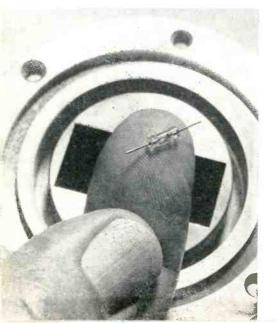
Laboratory comparator magnifies the inner structure of this gold-bonded diode.
