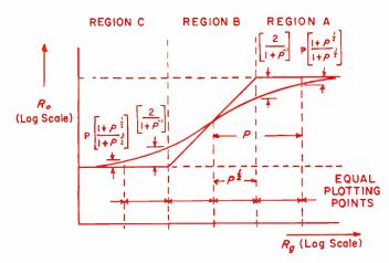
Fig. 8: The error ratio at equal plotting points from the center is given in terms of P, for conditions of Figs. 6 & 7.
