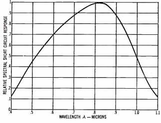
Fig. 6: Relative spectral response of short circuit 1 for uncoated cells for radiation of constant power per unit wavelength.
