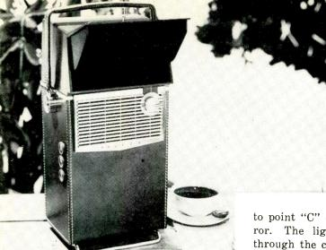
A TRANSISTORIZED portable television set has been placed on the market by the Philco Corporation. Called the "Safari," the portable TV set weighs 15 pounds including the battery. It is 83% inches wide, 165% inches high and 55% inches deep. The set employs twenty-one transistors, 14 diodes, and a 2-inch CRT.
