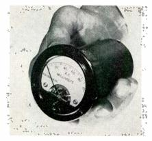
2 in. in dia. and less than 434 in. long. Basic range is 0, to 100 my RMS, Input impedance is 1 megohm, parallel by 10  $\mu\mu f$  adding almost no load to the circuit. It can be provided with any voltage range up to 300 v RMS. Frequency response is 20 CPS to 20 KC.  $\pm 2\%$ . Accuracy is  $\pm 3\%$  of full scale deflexion. Metronix, Inc., Chesterland, Ohio.
