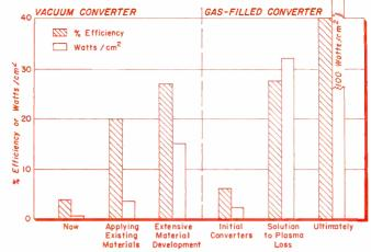
Fig. 17: The substantial research efforts of companies like General Electric (chart by Dr. Wilson of G.E.) indicate the "ultimate" column is feasible. At 40% efficiency, thermionic devices could effectively compete with conventional equipment.
