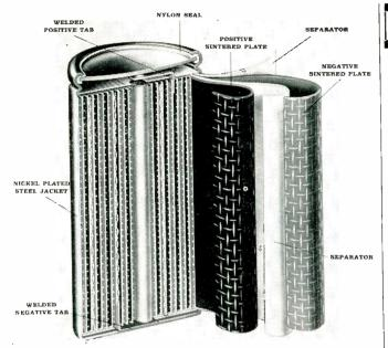
Tightly rolled sintered plates are made of fused metal particles.
