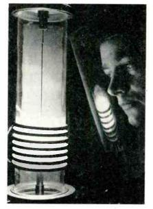
Westinghouse's J. J. Coleman watches ribbon-like germanium crystal rise from a molten pool in this furnace at the Company's Research Labs. Strips require none of the costly, cutting and grinding that wastes up to 80% of conventional ingots used in semiconductor device fabrication.
