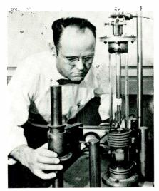
13: Research Fig. scientists at the National Bureau of Standards use this furnace to grow large single crystals by the Kyropolos technique. The crystals are used to study the thermoelectric (and other) properties of materials.
