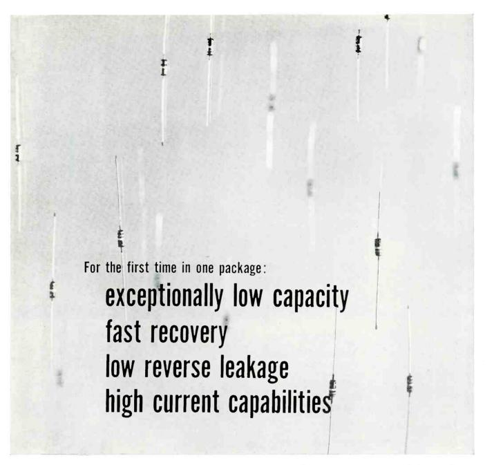
100 mA Min. @ 1V Forward Current...0.3  $\mu$ sec recovery...4  $\mu\mu$ f at -2V...that's what you get with the new Hughes computer diodes. With these characteristics, *these diodes will cover practically every major computer switching requirement*.
