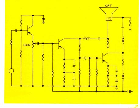
Fig. 14: (right) Cascaded push pull video amplifier.
