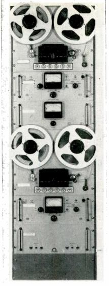
This rack houses an automatic tape recording system which delays signals up to one hour from time of original recording.
