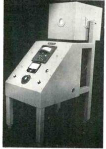
position at temperatures up to 1100°C. A clock motor is mounted for use in the growth of single crystals by the Bridgman technique. Furnace cores may be replaced within 2 min. while the furnace is still at temperature. A cast one piece insulation makes this a clean and simple operation. Replacement cores are supplied in wooden carrying cases. An anticipating controller, variac and ammeter are provided. Materials Research Corp., 47 Buena Vista Ave., Yonkers, N. Y.
