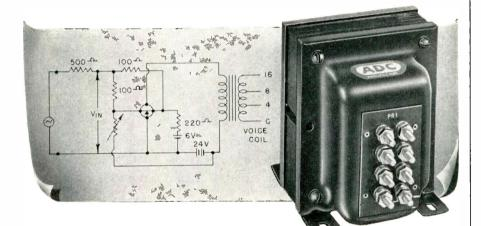
The tiny transistor transformers such as those illustrated at the right are for low power applications. Introduction of new, low distortion, power transistors has required larger transformers, especially for operation at low frequency. While these may
