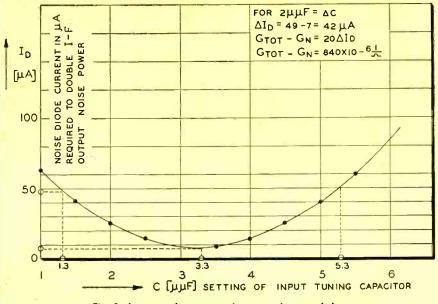
Fig. 2: Input conductance tuning curve is a parabola.
