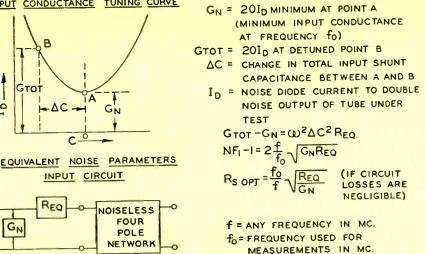
Fig. 4: Circuit components must have right characteristics at test frequencies.
