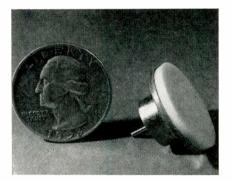
Fig. 2: High vacuum thermionic converter has special ceramic insulators developed by the General Electric Co. Coefficient expansion of of metal and ceramic parts are the same. Device operates from anv heat source. nuclear or conventional.
