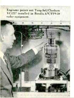
The Texas Tower and other key defense systems have required more and more powerful radar equipment. Bendix Radio, to keep pace with this need, replaced four bulky modulator tubes in its AN/FPS-20 radar unit with a single Tung-Sol/Chatham hydrogen thyratron.
