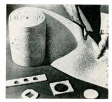
good tensile strength, density in the range of 20 lbs/cu. ft., good compression-deflection characteristics, useable temperature range  $-65^{\circ}F$  to  $500^{\circ}F$ . It is available from pilot plant equipment in sheets ¼ in. thick, 9 in. wide and 6 ft. long. The Connecticut Hard Rubber Co., 407 East St., New Haven 9. Conn.
