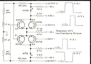
TYPICAL CIRCUITRY FOR OBTAINING 25-MC REP RATE IN NON-SATURATED FLIP-FLOP
