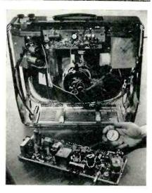
Loosening 3 screws, disconnecting 4 clip leads, and activating a spring loaded lever ejects the plated chassis board from Motorola's new TV set. Complete removal, or loosening for trouble shooting takes 33 sec.
