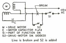
will not start until the drive-motor switch is closed, and when it is closed the tape recorder starts silently as the solenoid was energized previously. The tape recorder is stopped by opening the drive-motor switch. It does so silently as the solenoid remains energized.
