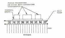
Fig. 3. Power transistor cooling device
