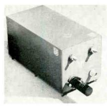
acteristics of the new Dual Delay Line are as follows: Delay, 1 to 1.5 µsec.; independently variable in each channel in increments of 0.05 µsec.; impedance—1000 ohms; output rise-time -0.06 µsec. per channel; dimensions— 8 x 4 x 4 inches. ESC Corporation, 534 Bergen Boulevard, Palisades Park, New Jersey.
