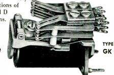
Operating Voltage: up to 220 volts d-c Contact Rating: up to 4 amperes at 150 watts Temperature Range: up to -55°C to +85°C Vibration: up to 10 to 55 cps at .062 inch double amplitude Operating Shock: up to 30 "g"
