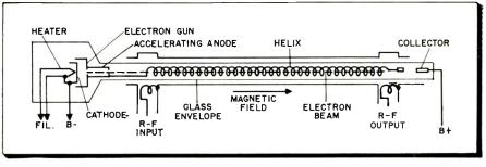
Fig. 4: Construction of the traveling wave tube
