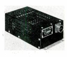
over the environmental range of  $-55^{\circ}$  C to  $+71^{\circ}$  C. Utilizing transistors in a bridge switching circuit for maximum reliability, 170-200 VA of single phase power and approximately 50 watts of three phase power are obtained from a unit weighing only 9½ lbs. Operates to 71° C without heat sinks or cooling air. Varo Manufacturing Co., Inc., 2201 Walnut St., Garland, Tex.
