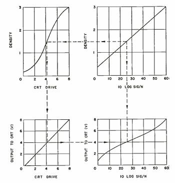
Fig. 10: Finding receiver compression for a linear density receiver.
