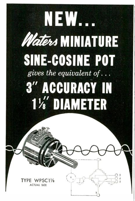
Designers of radar PPI displays and computer circuits, particularly, will welcome this new space-saving non-linear precision potentiometer. WPSC11/8 provides two accurate and separate 360° sinusoidal output voltages displaced 90° in phase, representing the sine and cosine of the angle of shaft rotation.
