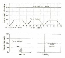
Charts show the lower efficiency and loss of transmitted power at desired frequency when the radar energy is pulsed.
