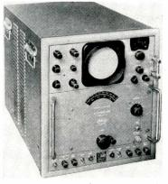
analyzes pulses as short as 0.1 microseconds. The instrument provides frequency dispersion up to 70 MC. It may be used for all microwave spectrum analysis work. For wide pulse analysis the instrument provides a narrower display bandwidth with 7 KC resolution. It features a logarithmic amplitude display. Polarad Electronics Corp., 43-20 34th St., Long Island City, N. Y.
