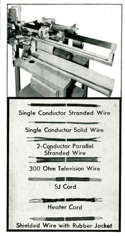
A new collecting device is now available for use on the popular Artos CS-6 wire-measuring, cutting and stripping machine. Illustration shows the new collecting trough (AE-478). Upper trough collects wire leads up to 60 inches long, then empties into the lower trough after wire has been cut, thus saving operator time.
