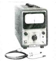
accuracy of  $\pm 3\%$  full scale. Use of a photoconductive chopper in place of the conventional mechanical vibrator helps achieve high sensitivity and reduces drift to less than 2  $\mu$ v. per hour after warm-up. Noise is less than 0.2  $\mu$ v. rms. It has a full-scale voltage sensitivity of  $\pm 10 \ \mu$ v. and a full-scale current sensitivity of  $\pm 10 \ \mu\mu$ a. Hewlett-Packard Co., 275 Page Mill Rd., Palo Alto, Calif.
