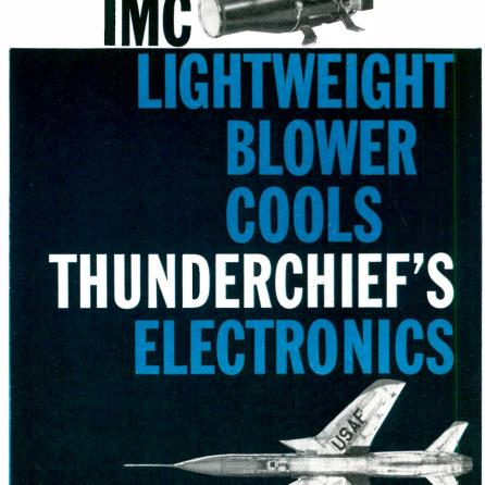
A 7-pound blower that delivers 180 cfm at 12 inches of static pressure! ... that's IMC's new unitized vaneaxial blower.
