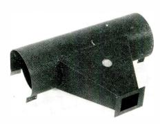
A ducted Netic traveling wave tube shield which directs the magnetic field developed by the enclosed solenoid structure, acts as a diversionary shield for fields originating in associated equipment, and provides more uniform cooling. Magnetic Shield Div. Perfection Mica Co.
