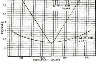
Fig. 8: VSWR of an input arm and the output of antenna arm
