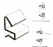
are snapped onto the panel. The male section of terminal connector is inserted into the rectangular panel hole, and as it passes through, spring legs of the clips compress and spring out again over the flanges projecting from either side of the connector. Flanges prevent the connector from passing completely through panel and clips prevent it from being pushed out when the other half of connector is applied. Tinnerman Products, Inc., Cleveland, Ohio.
