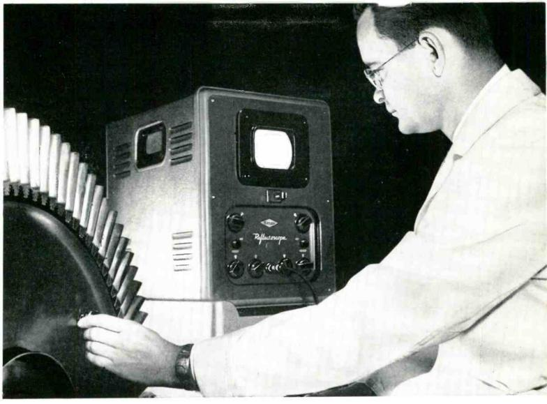
**TEST ENGINEER** touches Sperry Reflectoscope search unit to completed jet rotor forging in test for material flaws. A quartz crystal in the search unit converts high power pulse supplied by a Tung-Sol/Chatham 1258 hydrogen thyratron into ultrasonic vibrations. These traverse the forging . . . then echo back to be seen as "pips" on the scope. Irregularity of the "pip" pattern signals a material defect, thereby stopping costly trouble before it even starts.
