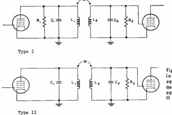
Fig. 1: Both of these interstages have equal resonant frequencies; Type I has equal damping, Type II unilateral. gain and the required bandwidth. From Figs. 2 and 3 the designer can determine the number of double-tuned interstages needed to meet these requirements. Fig. 2 is to be used for Type I interstages; Fig. 3 for Type II.
