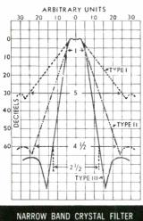
TYPICAL RESPONSE CURVES INDICATING THE VARIOUS SHAPE FACTORS AVAILABLE IN STANDARDIZED BURNELL CRYSTAL FILTERS ARBITRARY UNITS
