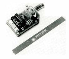
often eliminated. Design time can thus be concentrated on new circuitry. The modules also can be used in production of electronic equipment. They can be combined to build at least 35 complete circuits including tape recorder, broadcast, pre-amplifier, broadcast line amplifier, tape playback amplifier, public address system, control amplifiers and modulators. Packard-Bell Electronics Corp., 12333 W. Olympic Blvd., Los Angeles 64, Calif.
