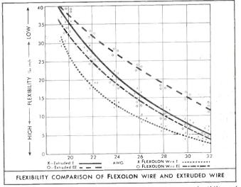
Plot of flexibility as recorded in tests proves greater flexibility of  $F_{LEXOLON}$  wire with R/M "Teflon" tape insulation. For complete testing data, call the man from Tensolite, or write for free FLEXOLON hook-up wire bulletin.
