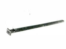
A broad-band, power absorbing, waveguide waterload, the B-570, absorbs up to 400 watts of CW power over the frequency range of 4.95 to 10.5 KMC, and the VSWR is under 1.20 over this range. This represents a reflected power of under 1%. Bomac Laboratories, Inc.
