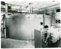
Delicate accelerometers for TITAN inertial guidance systems will be tested in new Genisco G-460 Ultra-Precision Centrifuge at American Bosch Arma Corp., Garden City, N. Y.
