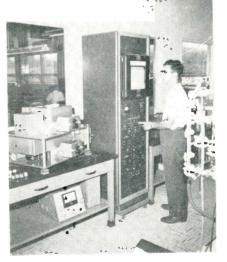
This ultra-violet emission-excitation Radiometer at Sylvania's new Towanda, Pa. research labs measures the spectral energy distribution of fluorescent phosphors.
