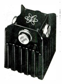
100 watts output at 40,000 ft. and operate at 71° C ambient temperature with no heat sink required. Converters are capable of output power up to 200 watts dc continuous. Operating range is from  $-55^{\circ}$  to 71° C. Unit weighs only 2.7 lbs. Communication Accessories Co., Lee's Summit, Mo. Circle 252 on Inquiry Card. page 149
