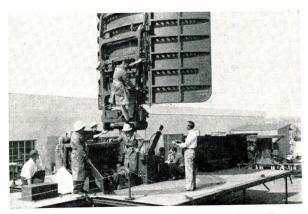
**Ground Systems** being developed at Hughes in Fullerton provide mobile three-dimensional radar protection and highspeed data handling.
