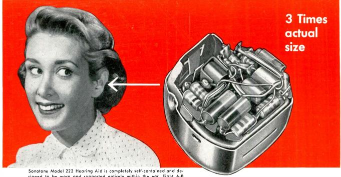
signed to be worn and supported entirely within the ear. Eight A-B Type TR, 1/10-watt resistors are used in the three-transistor amplifier.
