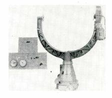
simultaneously tilt the antenna up to  $180^{\circ}$  and rotate  $370^{\circ}$  at variable speeds up to  $30^{\circ}$  per second. The rotator is remotely operated by means of a variac control and joy stick. Position indicators for both azimuth and tilt are in the control panel. It is built for service under severe weather conditions. Houston Fearless Corp. 11813 W. Olympic Blvd., Los Angeles, Calif.
