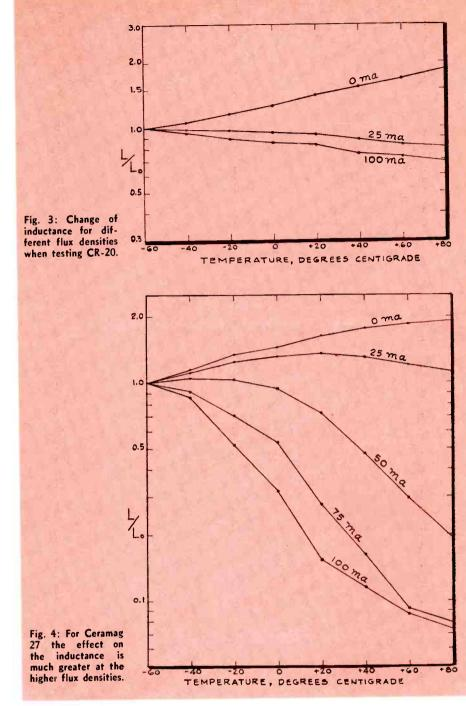
used temperature range of  $-60^{\circ}$  C to  $+80^{\circ}$  C, which were common in the early high permeability ferrites.
