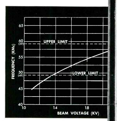
An exclusive Bendix Red Bank product, the Type TE-67 Backward-Wave Oscillator Tube generates microwave energy at extremely high frequencies never before available.
