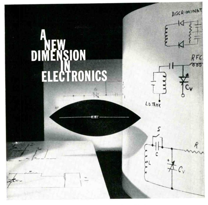
The Hughes silicon capacitor is a new kind of device whose full impact upon semiconductor electronics has yet to be determined. Most certainly, the silicon capacitor uncovers an entire realm of possibilities. Desirable equipment not now existing can be made for the first time. And, in every instance, bonus benefits of reduced size and weight plus greater simplicity result.
